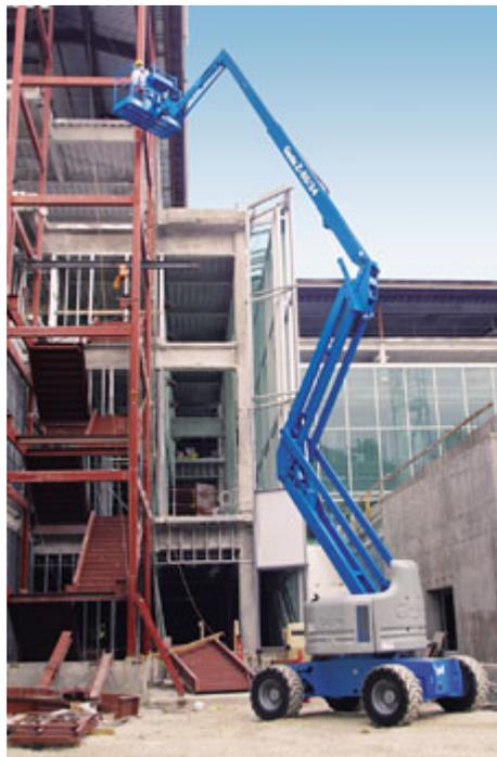
**Photograph 4** An articulating boom (Source – [www.geineindustries.com](http://www.geineindustries.com))
