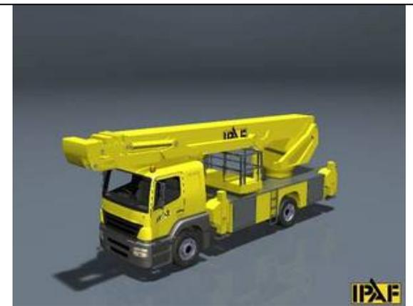
**Photographs 6 & 7** Two different types of vehicle mounted boom (Source – [www.ipaf.org](http://www.ipaf.org))
