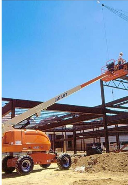
**Photograph 5** A telescopic boom (Source – [www.jlg.com](http://www.jlg.com))
