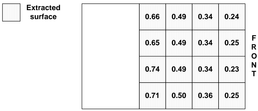
Figure 2.6 Velocity profile of downdraught bench operating at the recommended flow rate. Velocities quoted are in \text{ms}^{-1}
