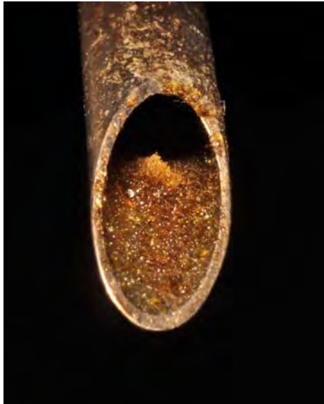
Figure 3.3 Close up photograph showing condensed colophony fume in the extraction nozzle tip. Fume also tended to condense at the point where the tube enters the extraction base unit
