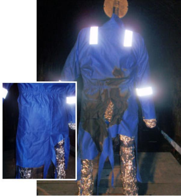
**Figure 4.4-2 New 'Antiflame' overall with light diesel contamination on mannequin before and after test**
