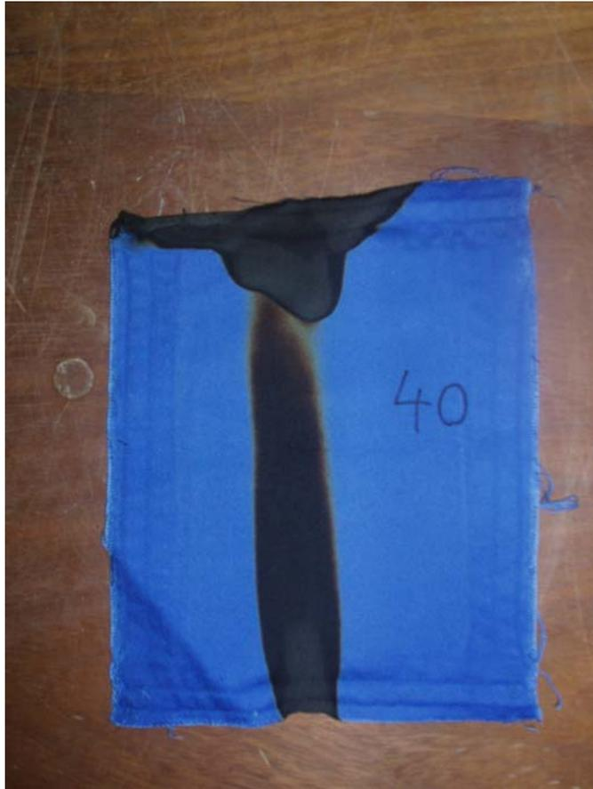
**Figure 4.3-1 'Antifiame' sample after 14 cycles of staining and washing**
