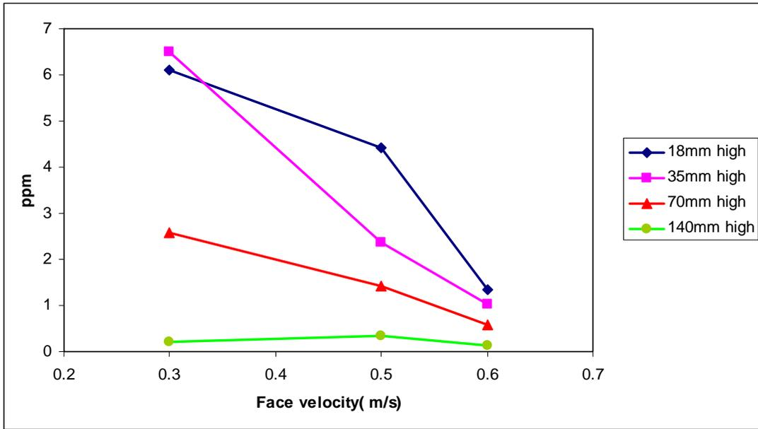
**Figure 3.13** Breathing zone concentration plotted against enclosure face velocity for various release heights
