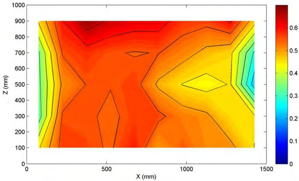
**Figure 3.1** Flooded velocity contour plot at the face of the enclosure. Circular rear baffle at 750 mm ( $0.75 \text{ m}^3 \text{ s}^{-1}$ ) Note: units of right hand scale are  $\text{ms}^{-1}$
