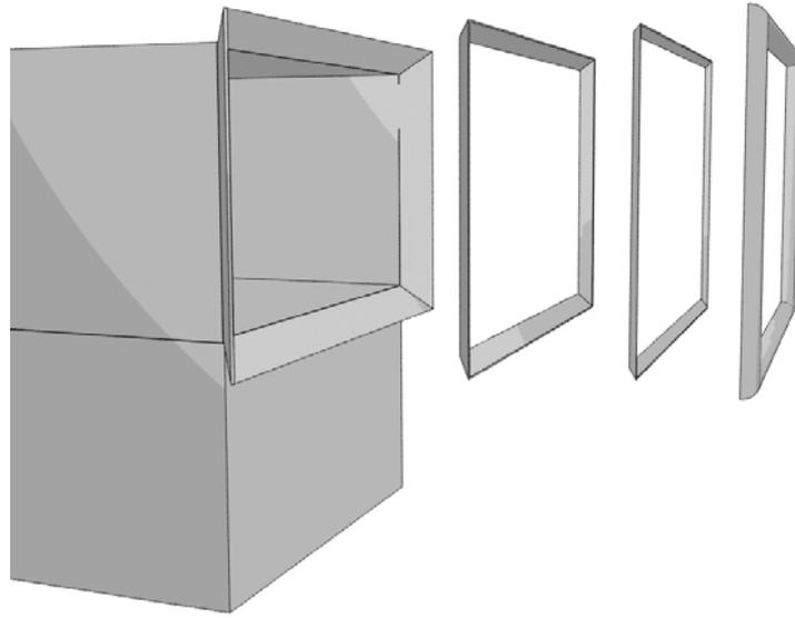
**Figure 2.2** Illustration showing the three 45° flanges and the half round flange
