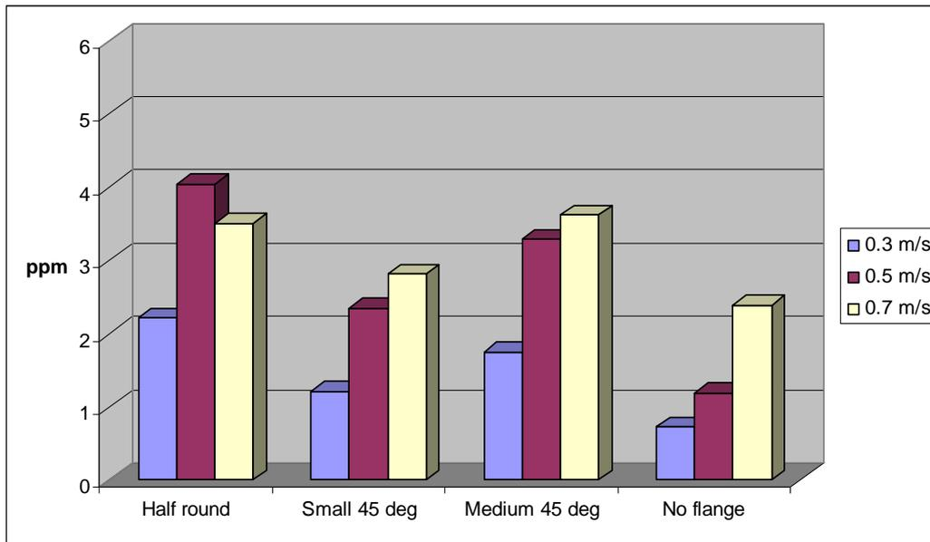
**Figure 3.10** Breathing zone concentration for three flanges and the no flange condition at three face velocities (Circular baffle fitted at 750 mm)
