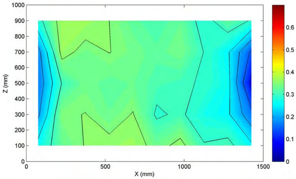
**Figure A.3** Flooded velocity contour plot at the face of the enclosure. Circular rear baffle at 750 mm ( $0.45 \text{ m}^3 \text{ s}^{-1}$ ) Note: units of right hand scale are  $\text{ms}^{-1}$
