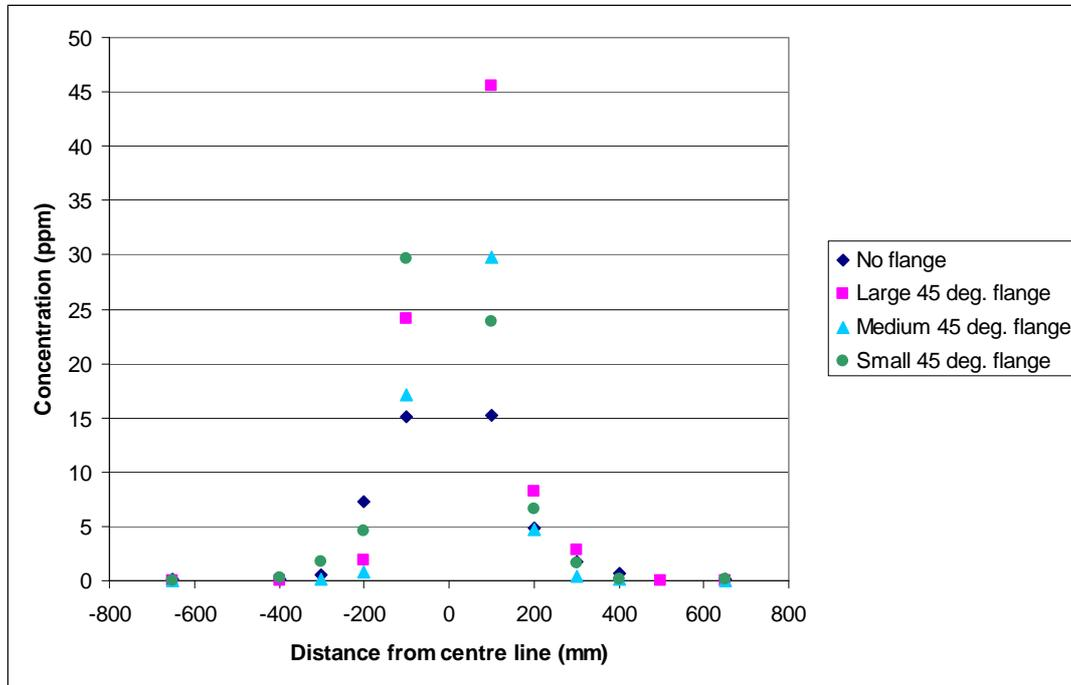
**Figure 3.8** Tracer gas concentrations either side of the release position
