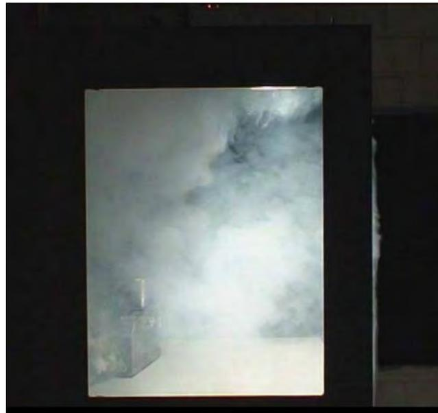
**Figure 3.4** Enclosure viewed from the side showing wall eddies protruding beyond the plane of the enclosure opening (see right of picture)
