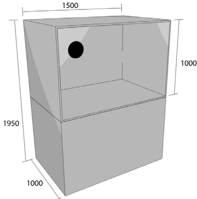
**Figure 2.1** Schematic of the enclosure with no baffle fitted
