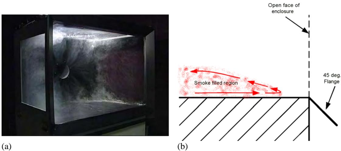
**Figure 3.5** Enclosure with large 45° flange fitted (a) Wall eddies made visible using smoke 5 seconds after smoke production was halted (b) illustration of wall eddies based on flow visualisation – side view of the floor of the enclosure
