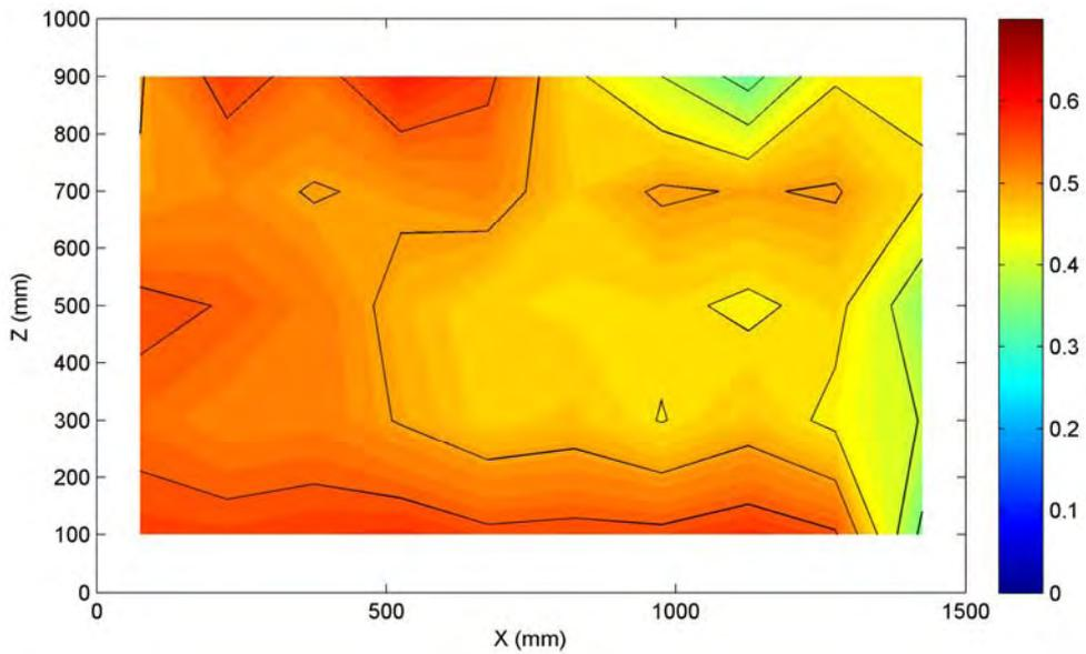
**Figure A.6** Flooded velocity at the face of the enclosure.
