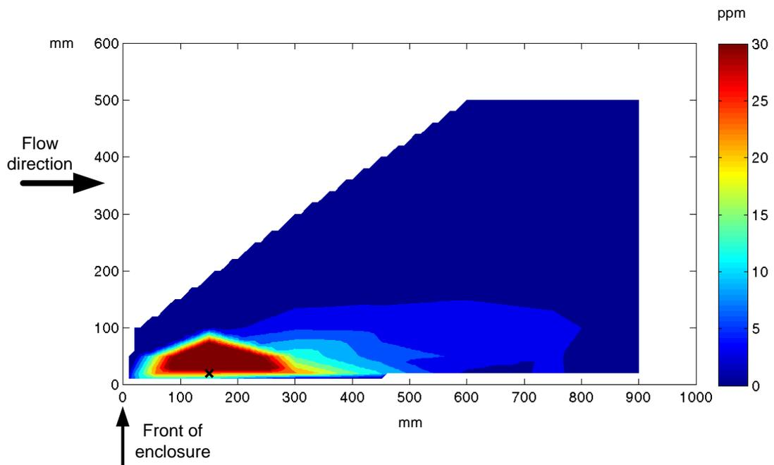
**Figure 3.7** Flooded concentration contour plot along the centre-line (front to rear) of the enclosure with the large  $45^\circ$  flange fitted ( $0.75 \text{ m}^3 \text{ s}^{-1}$ )
