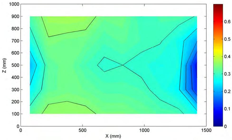
**Figure A.1** Flooded velocity at the face of the enclosure.
