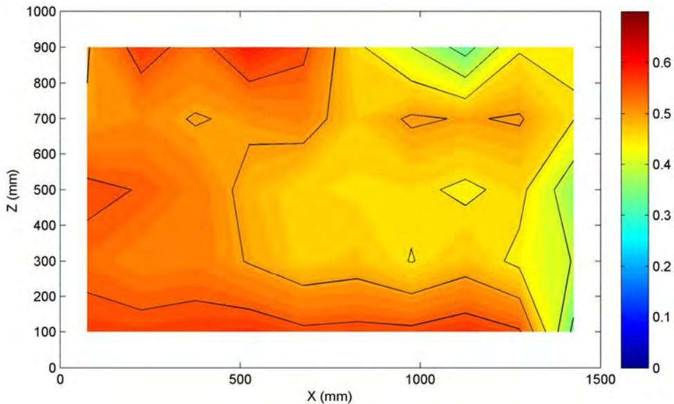
**Figure 3.2** Flooded velocity at the face of the enclosure. Slotted rear baffle at 750 mm ( $0.75 \text{ m}^3 \text{ s}^{-1}$ ) Note: units of right hand scale are  $\text{ms}^{-1}$
