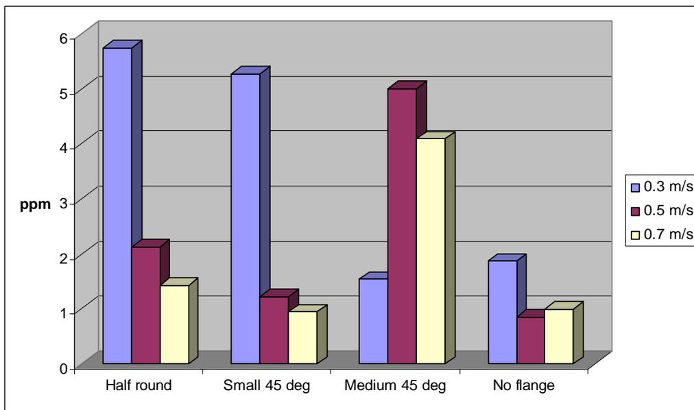
**Figure 3.11** Breathing zone concentration for three flanges and the no flange condition at three face velocities (Circular extraction opening at 1000 mm)
