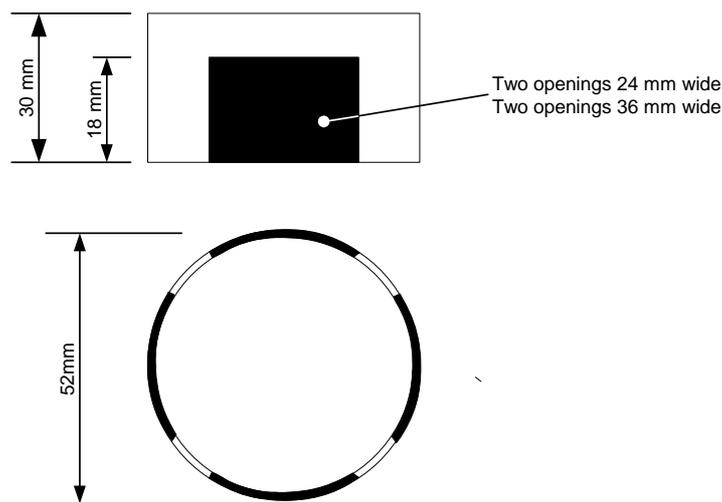
**Figure 3.12** Geometry of the cylindrical cap placed over the open end of the 28 mm tube
