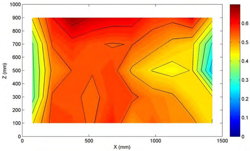
**Figure A.4** Flooded velocity contour plot at the face of the enclosure. Circular rear baffle at 750 mm ( $0.75 \text{ m}^3 \text{ s}^{-1}$ ) Note: units of right hand scale are  $\text{ms}^{-1}$
