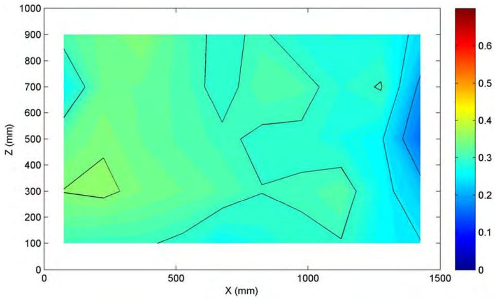
**Figure A.5** Flooded velocity at the face of the enclosure.
