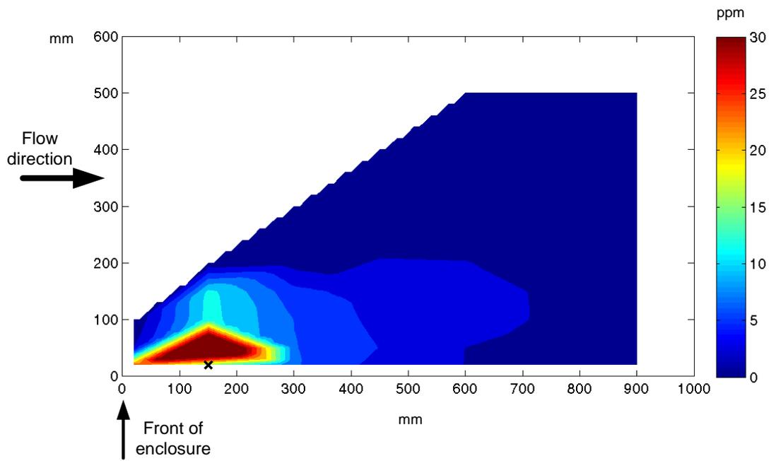
**Figure 3.6** Flooded concentration contour plot along the centre-line (front to rear) of the enclosure with no flange fitted ( $0.75 \text{ m}^3 \text{ s}^{-1}$ )
