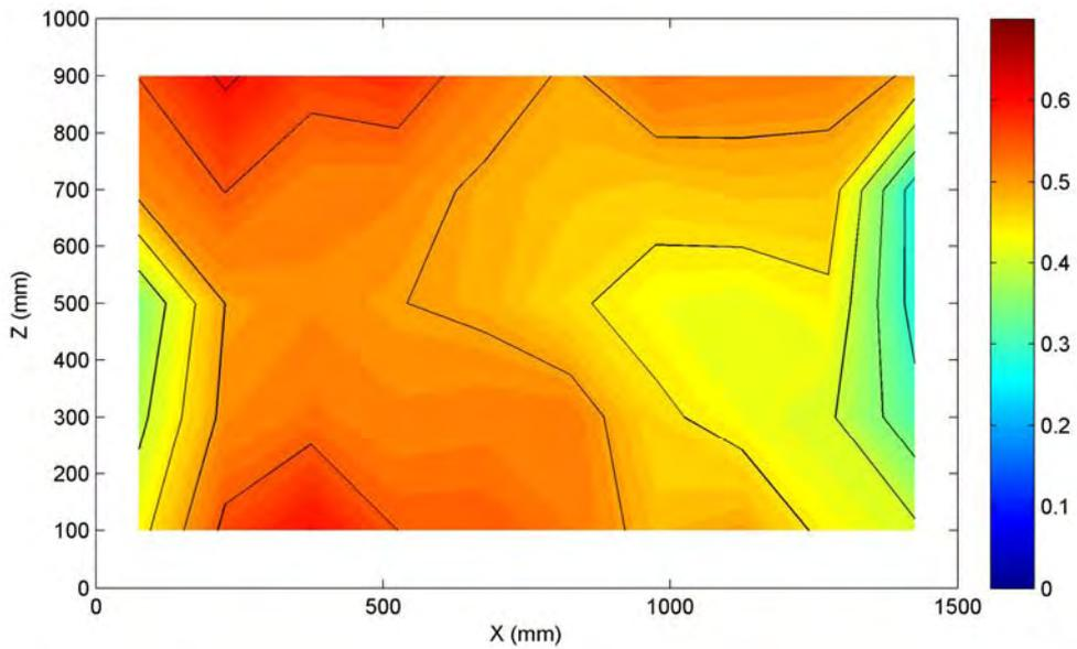
**Figure A.2** Flooded velocity at the face of the enclosure.
