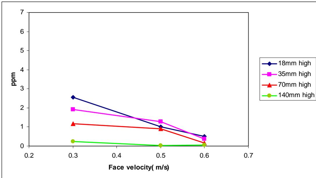
**Figure 3.14** Breathing zone concentration plotted against enclosure face velocity for various release heights
