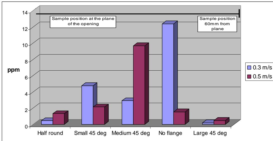
**Figure 3.9** Breathing zone concentration for four flanges and the no flange condition at two face velocities (slotted baffle fitted)
