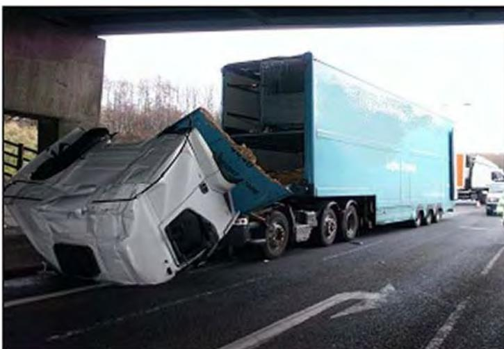
The incident shown in the photograph above occurred outside a distribution centre near Rochdale. The trailer was loaded with empty roll cages, which were not loaded to the headboard. As the vehicle braked for the junction, the roll cages rolled forwards and smashed through the headboard.
