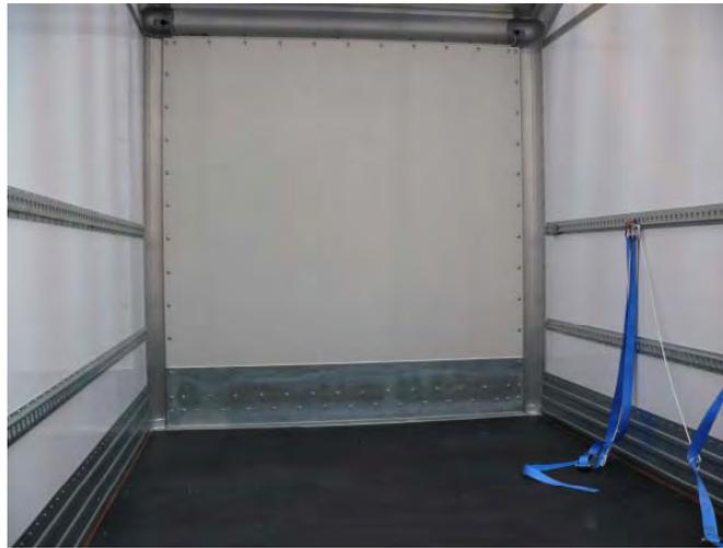
Figure 1 – Side rails in a box-sided trailer
