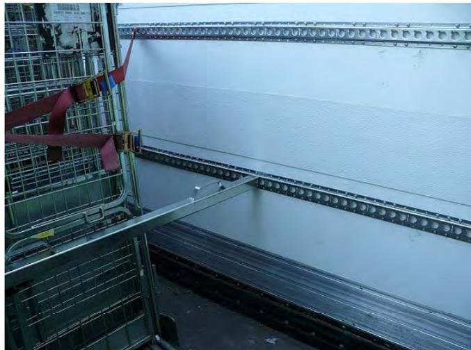
Figure 2 – side rails used with bars
