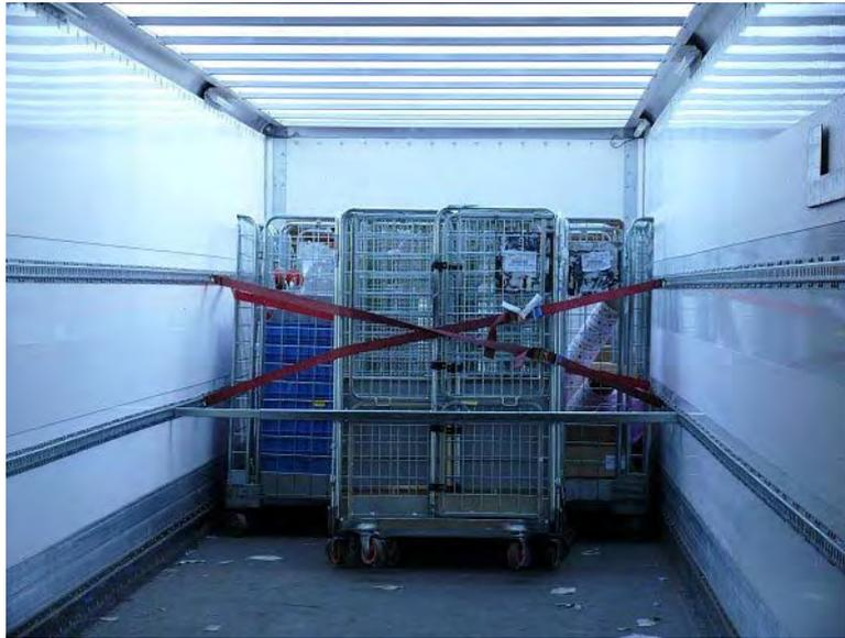
Figure 3 – combination straps and bars
