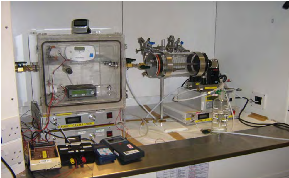
Figure A3: Equipment set up for the UL 2034 test
