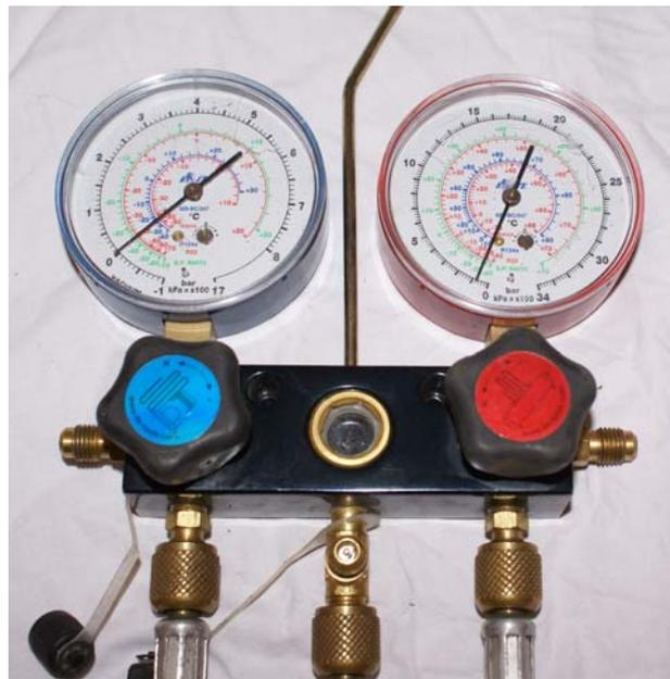
*A typical engineers manifold.*
