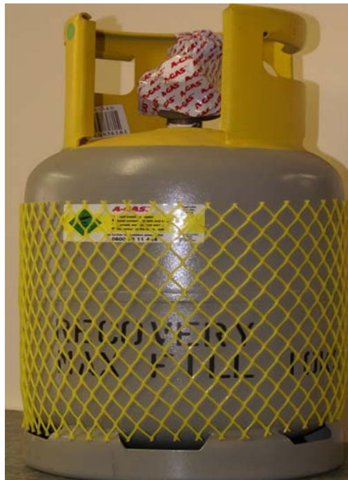
*A typical recovery cylinder, these can come in a variety of sizes.*
