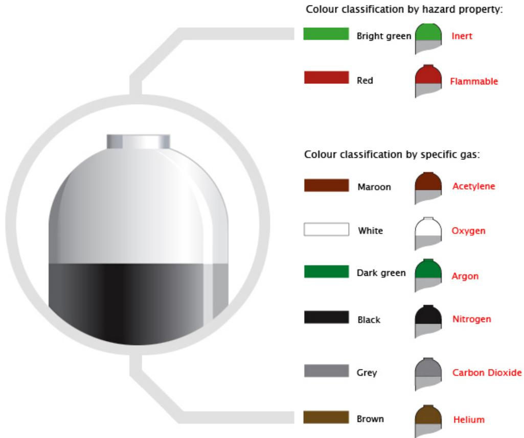
*A gas cylinder identification table. Reproduced with permission by BOC*
