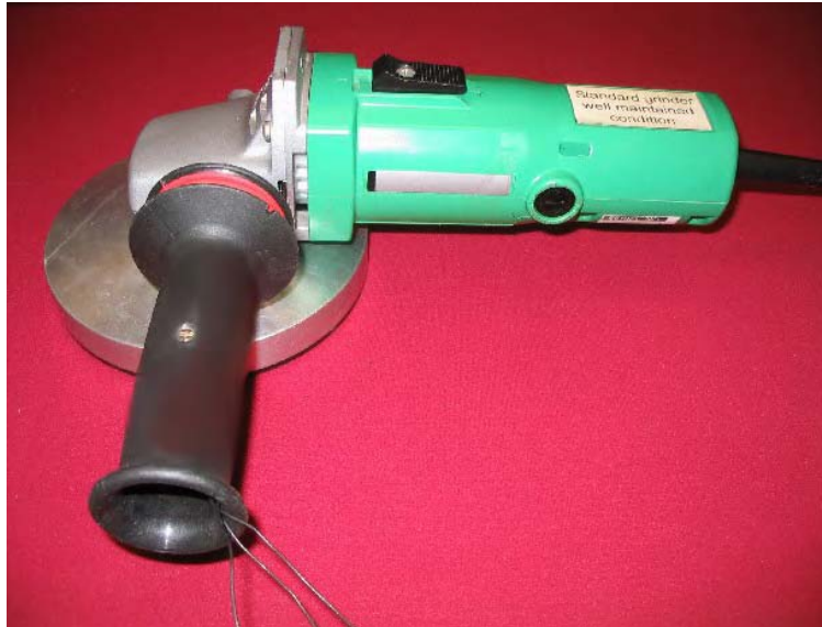
Figure A.1b. 125mm angle grinder used for tests on tool handles
