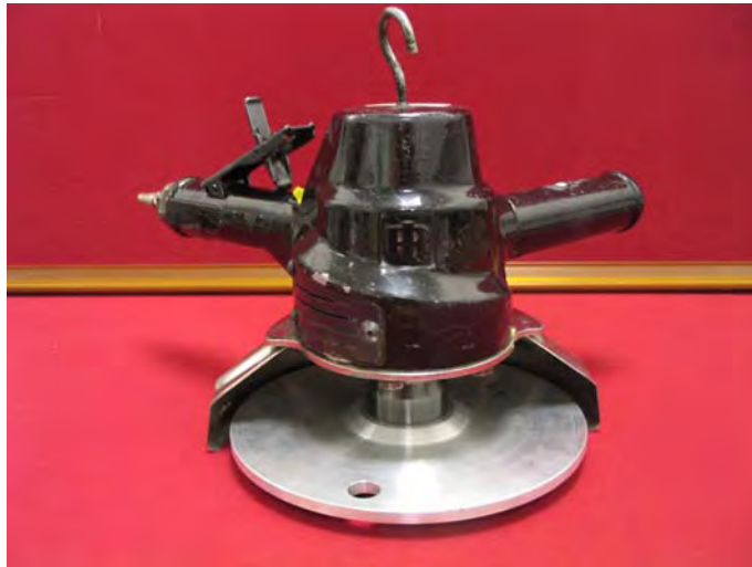
Figure A.1a. Vertical grinder used for tests on tool handles (handle to right of photograph used for measurements)
