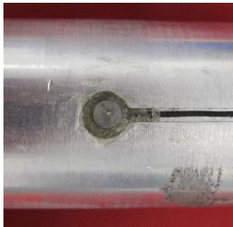
Figure 2c. Close-up of x/z axis transducer in surface of handle
