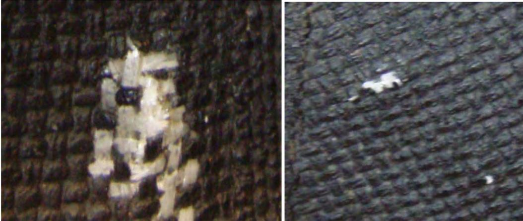
Image g and h. Internal surface marking from penetration testing.
