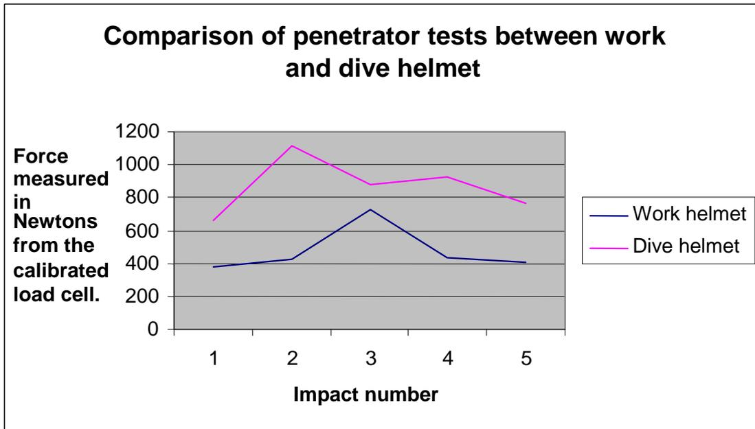
As per the 50-Joule impacts it can be seen that the dive helmet is not as effective as the work helmet for dissipating the force of an impact.
