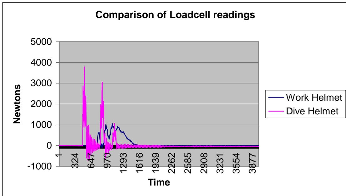
Comparison of the real time readings from impacts to Dive helmet run 9 and Work Helmet run 9. The data for the dive helmet shows a second impact from the impactor as the impactor bounces off the helmet. The work helmet for this run was a Yellow MSA Super Gard 11 date of manufacture first quarter of 1997.
