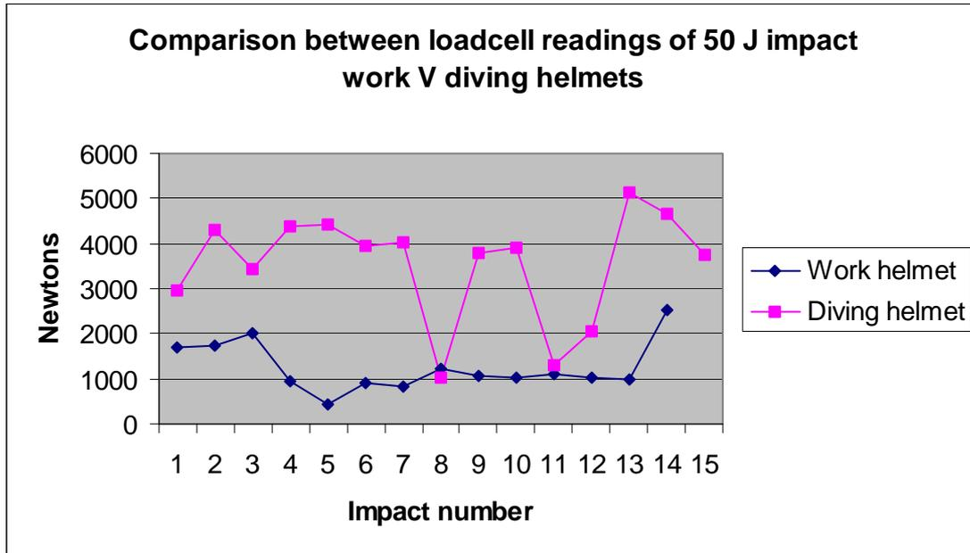
Data taken from calibrated load cell placed between headform and base. Impact 4, 5 and 6 for the dive helmet runs are with the non standard foam fitted to the head cushion.
