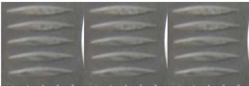
Measuring the PTV of this surface at 45° with either the 76mm or 38mm slider in water-wet conditions gives a reading of 27, suggesting that the 45° measurement is very close to the worst-case scenario for this flooring material. The narrow slider may be useful in separating the slip resistance effects of small regions of other profile patterns.
