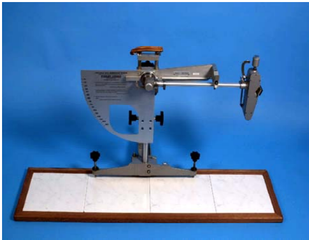
Figure 2.1. The ‘Stanley’ Pendulum CoF test
