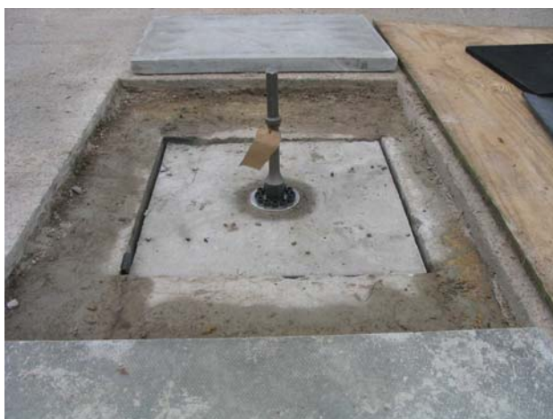
Figure 6c: Part of intermediate piece fitted with tools appropriately sized for the breaker under test
