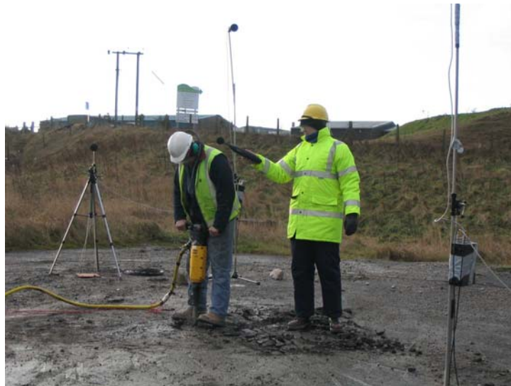
Figure 10: Noise measurements at the operator's ear
