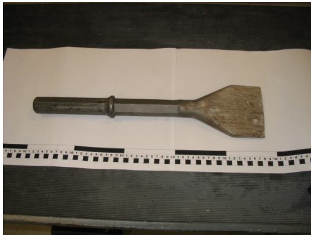
Figure 9a: Standard cutter used for breaking tarmac
