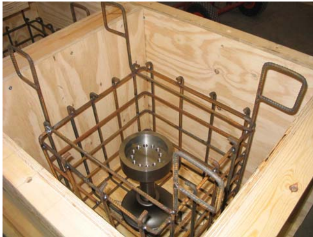
Figure 6a: Part of the intermediate piece embedded in concrete block (tool attached to rammer with 180 mm diameter)
