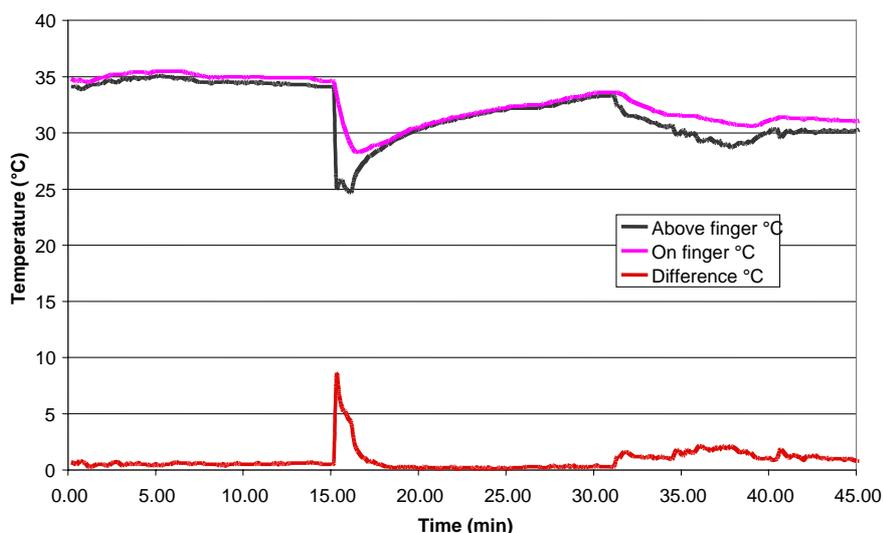
**Figure 13: Sensor response while wearing a glove**
