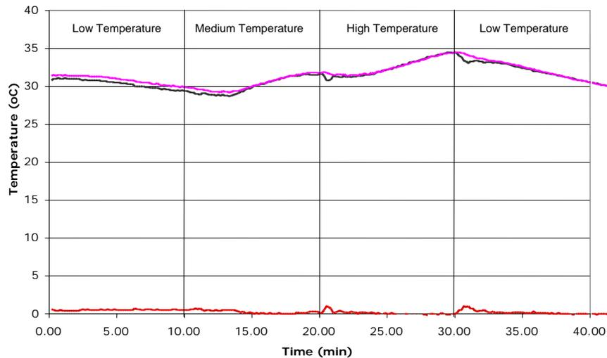
**Figure 11:** Sensor response to differences in environmental temperature
