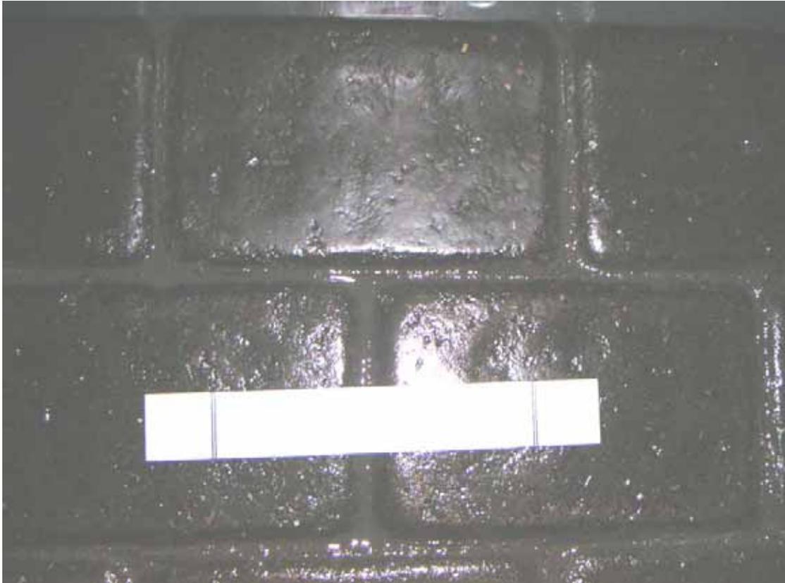
**Rz Surface Roughness:** 13.7  $\mu\text{m}$  (mean)
