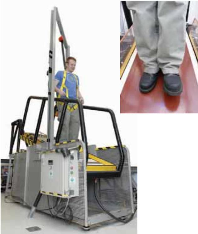
**Figure 4** The UKSRG ramp CoF test
