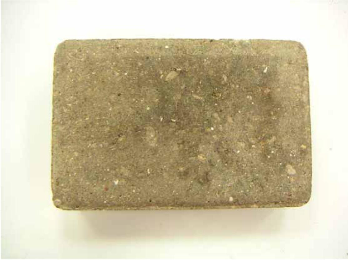
**Rz Surface Roughness:** 68.2  $\mu\text{m}$  (mean)
