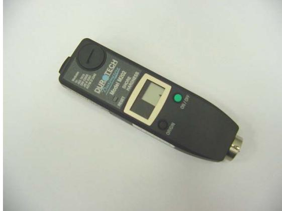
Figure 2.4 The Durotech M202 Shore hardness meter.
