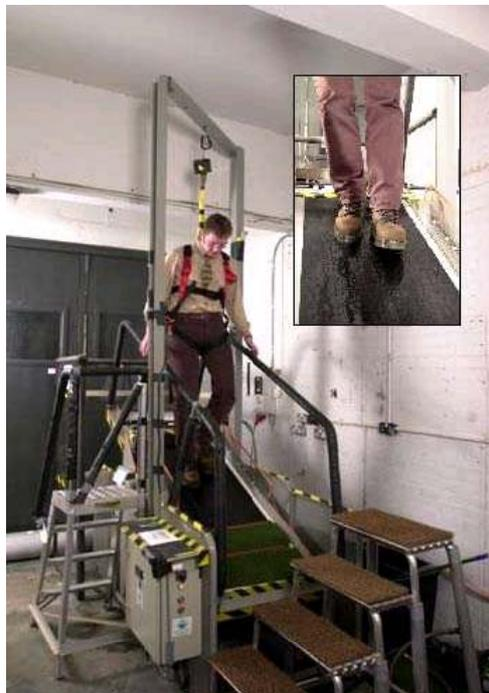
Figure 2.2 The HSL-PS-SOP-12 ramp-based coefficient of friction test.
