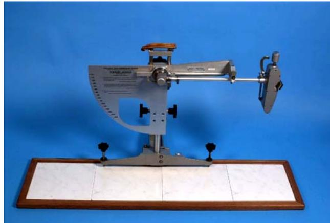
**Figure 2.2:** The “Stanley” Pendulum CoF test.
