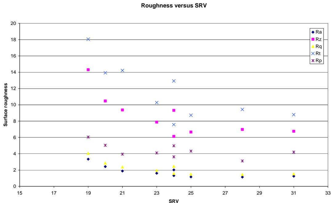
Figure 3.1 Graph showing a range of surface roughness parameters (all measured in  $\mu\text{m}$ ) plotted against SRV data for wet conditions.
