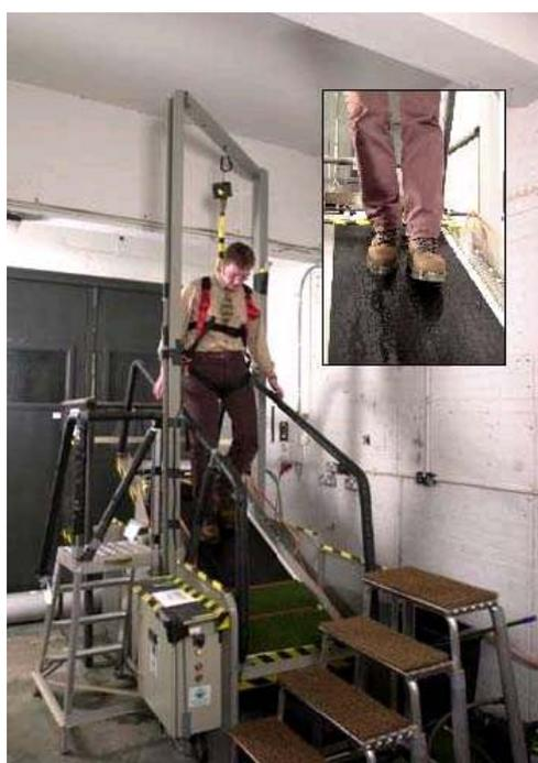
**Figure 2.3:** The ‘HSL-PS-SOP-12’ ramp CoF test.
