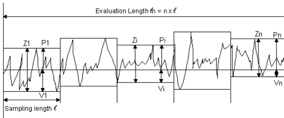
The Rz surface roughness parameter is defined as the mean of the sum of  $Z_i$  within each sampling length over the entire evaluation length.
