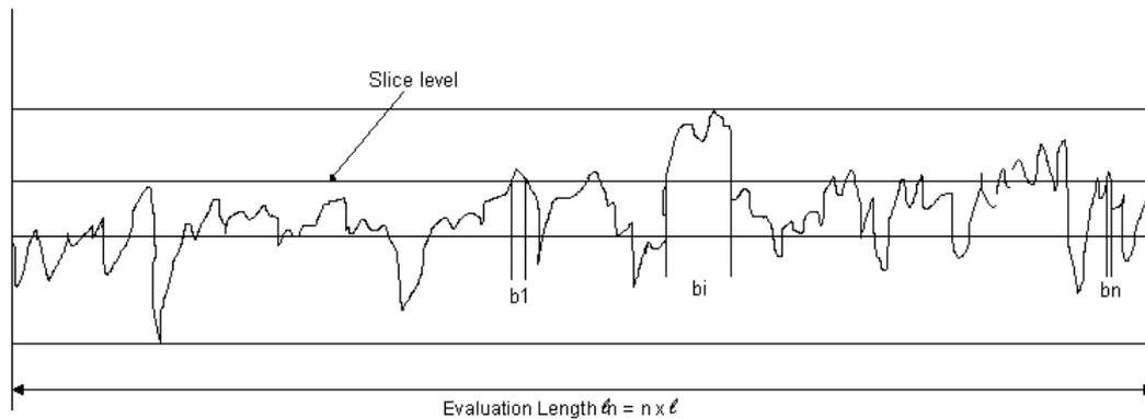
Schematic diagram showing how  $R_{mr}$  is calculated
