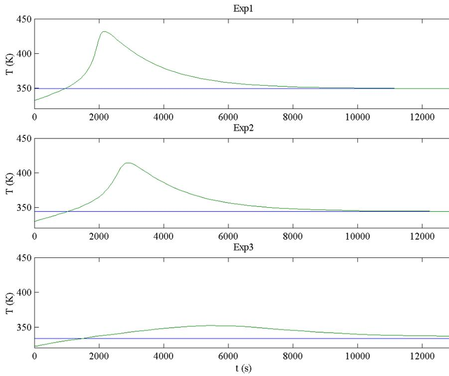
Figure 3. Jacket (blue) and reactor (green) simulated temperatures for Exp1, Exp2 and Exp3
