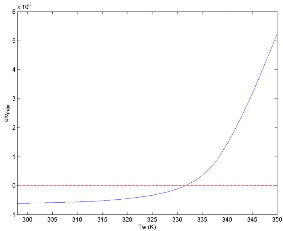
Figure 2. Maximum analytical divergence (blue) obtained in the first 12000 s for the studied system and divergence criterion runaway boundary (discontinuous red).
