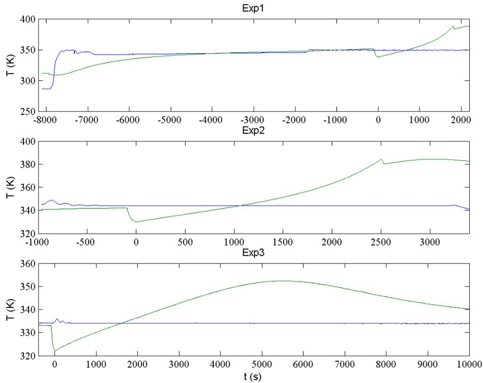
Figure 10. Experimental reactor (green) and jacket (blue) temperatures of 200 litres batch experiments Exp1, Exp2 and Exp3.
