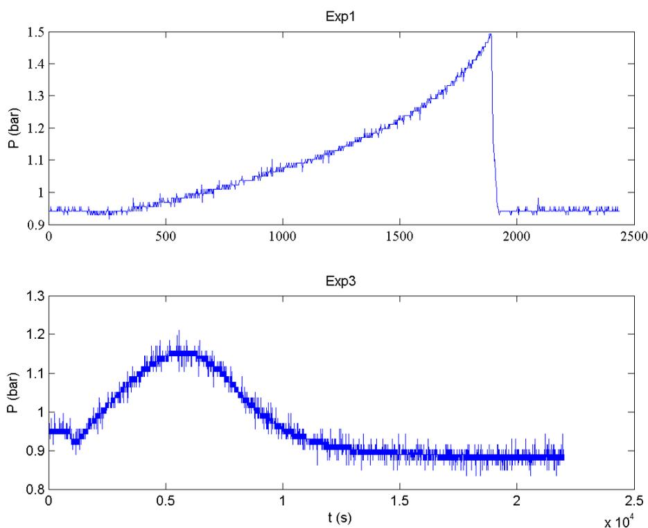
Figure 11. Pressure data recorded in Exp1 (upper layer) and Exp3 (lower layer)
