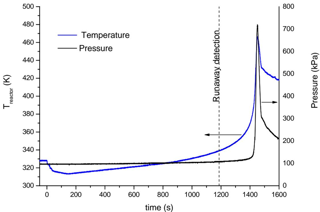
**Figure 2 Detection of runaway during test HP6**
