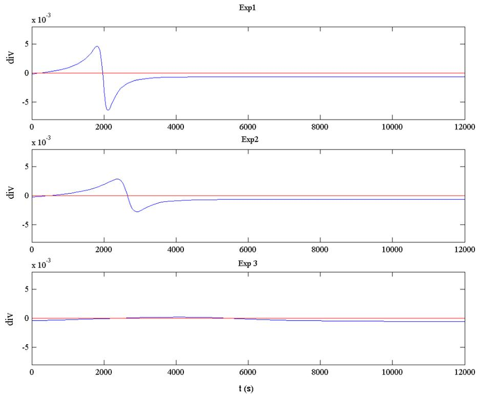
Figure 4. Divergence (blue) and divergence criterion limit (red) obtained from simulation of Exp1, Exp 2 and Exp 3.
