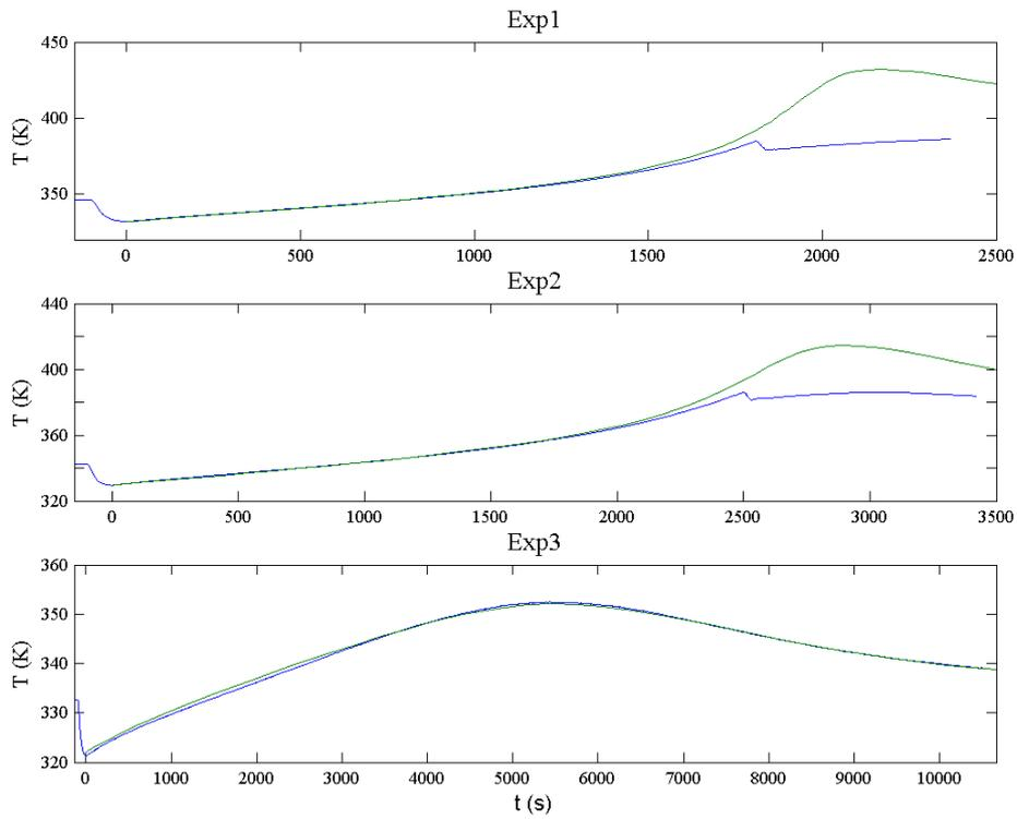
Figure 12. Experimental (blue) and simulated (green) reactor temperature in Exp1, Exp2 and Exp3
