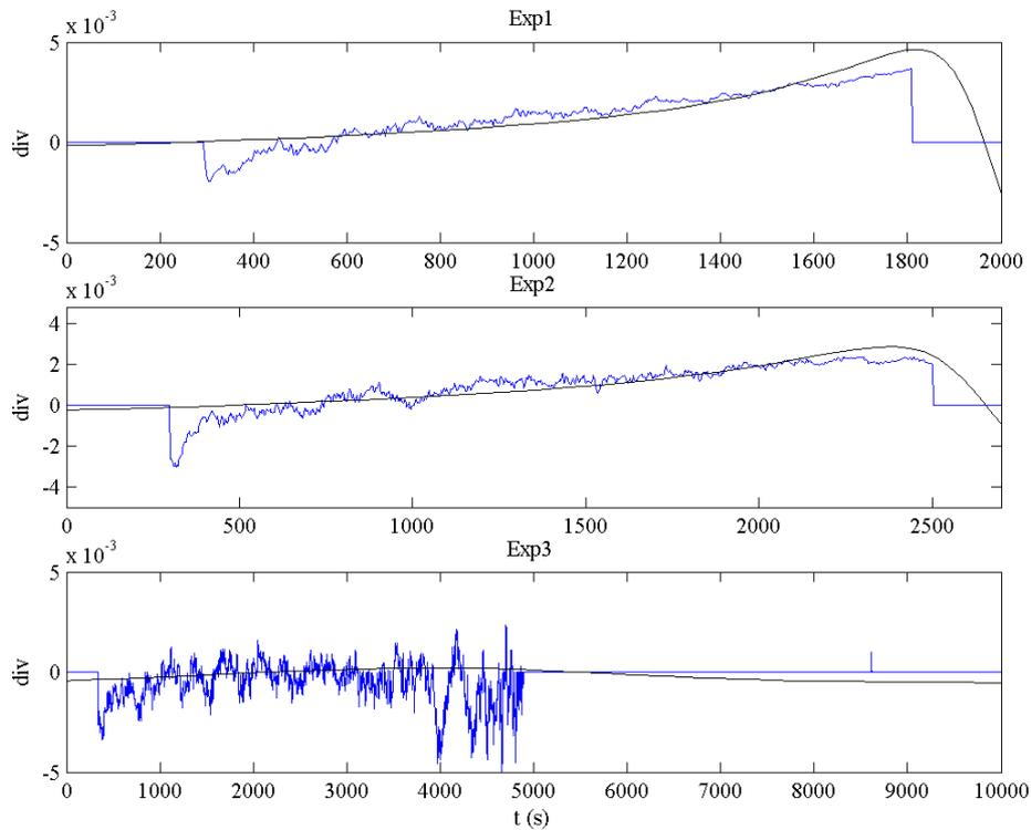
Figure 14. Reconstructed (blue) and analytical (black) divergence using  $\{T_r(t), T_r(t-\Delta t_2)\}$  state space on TT02 on HSL1, HSL2 and HSL3 ( $\Delta t_1 \Delta t_2= 100s$ )
