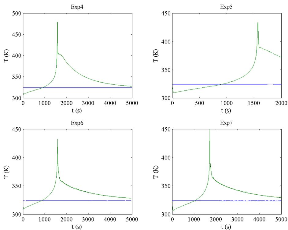
Figure 5. Jacket (blue) and reactor (green) temperatures profiles for Exp4, Exp5, Exp6 and Exp7.
