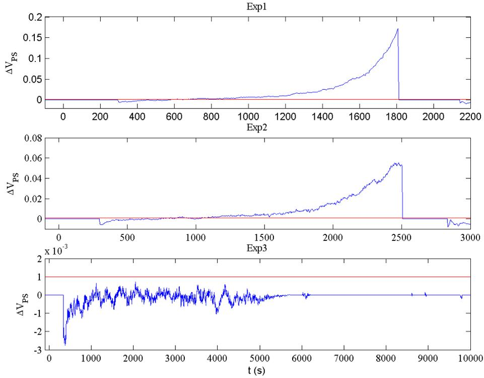
Figure 16.  $\Delta V_{PS}$  values (blue) obtained using  $\{T_r(t), T_r(t-\Delta t_2)\}$  state space on TT02 during HSL1, HSL2 and HSL3. ( $\Delta t_1=\Delta t_2= 100$ s and  $\Delta V_{PS}^{lim} = 1 \cdot 10^{-3}$ )
