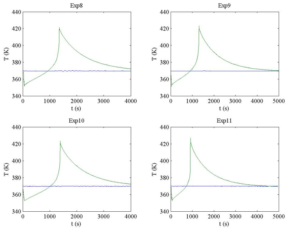
Figure 7. Jacket (blue) and reactor (green) temperatures profiles for Exp8, Exp9, Exp10 and Exp11
