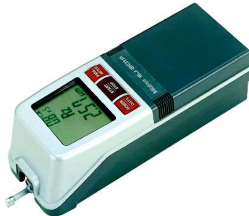
Figure 2.1 The Mitutoyo SJ-201P microroughness transducer
