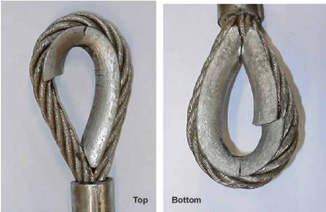
Figure 7 Collapsed thimbles on sample 4 after 5,185 cycles
