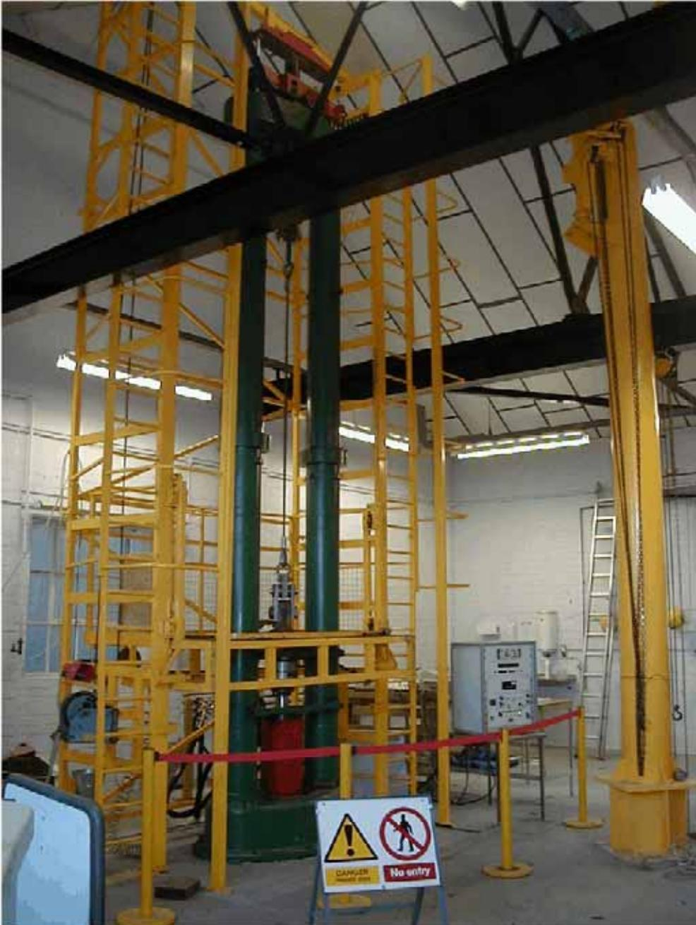
Figure 1 The axial fatigue facility with a wire rope sling leg specimen installed
