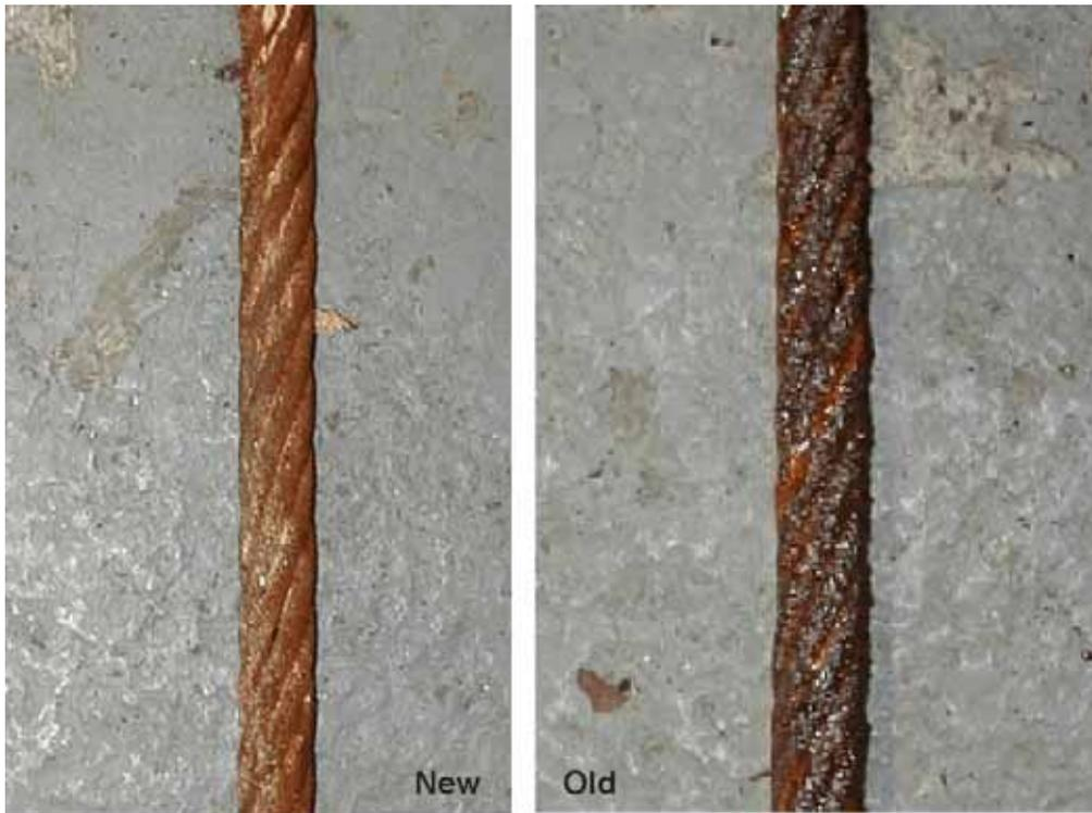
**Figure 8** Rope samples after accelerated corrosion for 5 weeks
