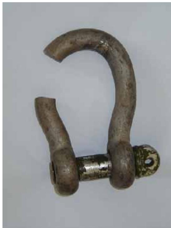
**Figure 9** Failure in the upper attachment shackle after 58,100 cycles
