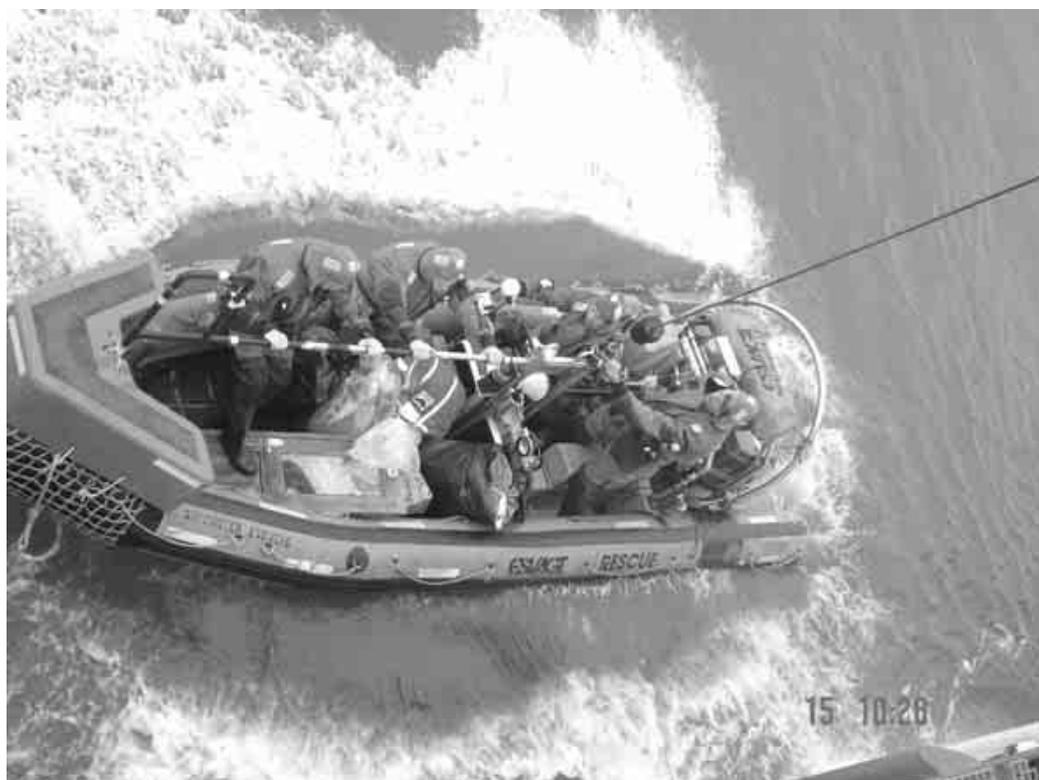
Handholds are provided all the personnel in this FRC with the addition of a longitudinal rail
