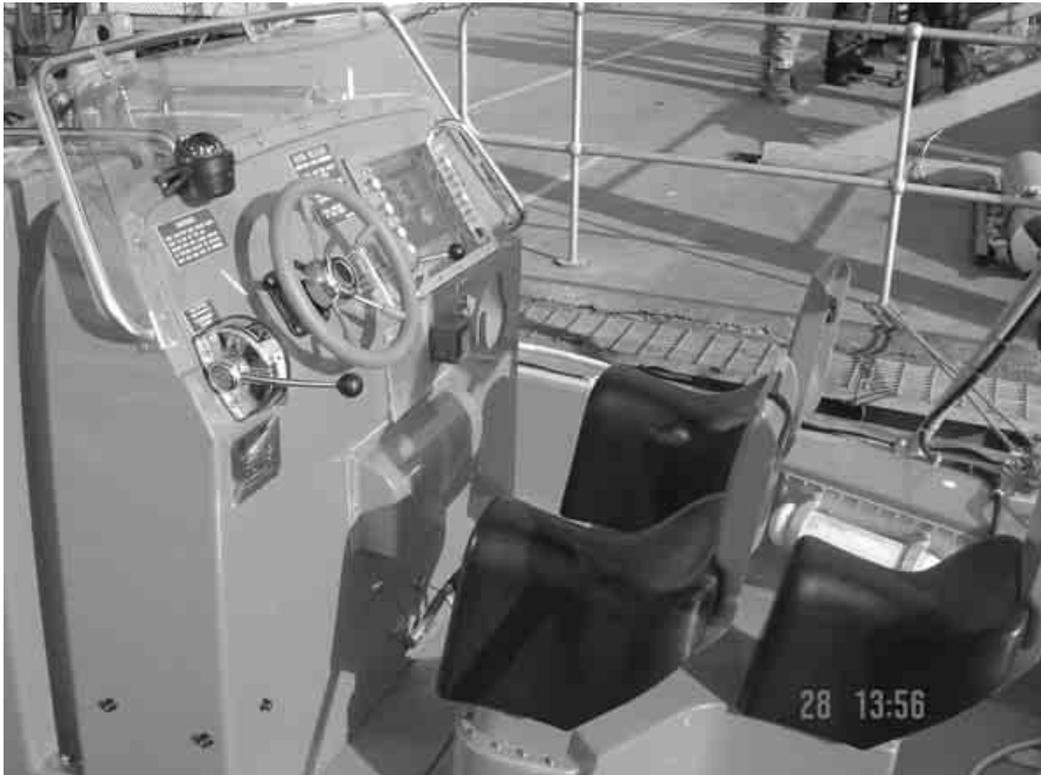
Double console and staggered saddle seating on an FRC
