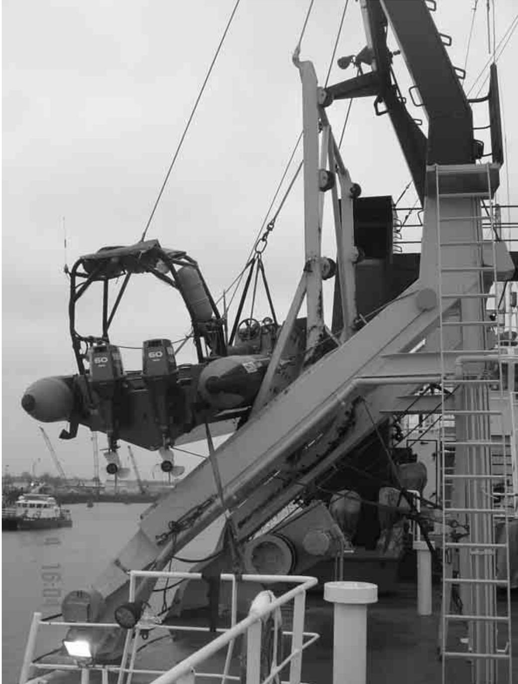
Miranda davit being used to handle an FRC
