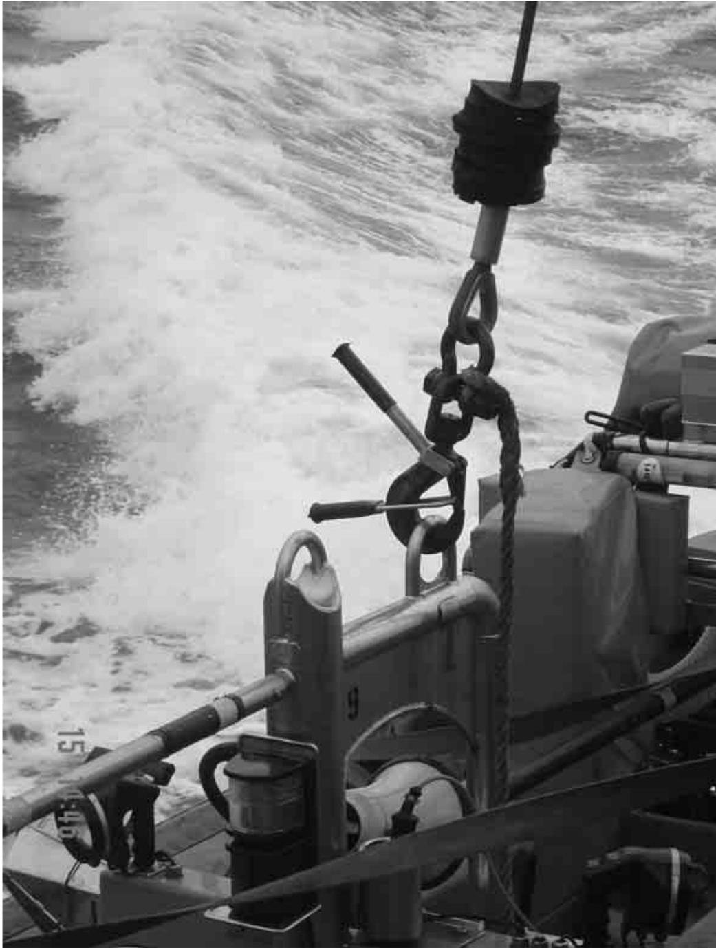
The modified snap hook used by Esvagt that is combined with a pole and hook system
