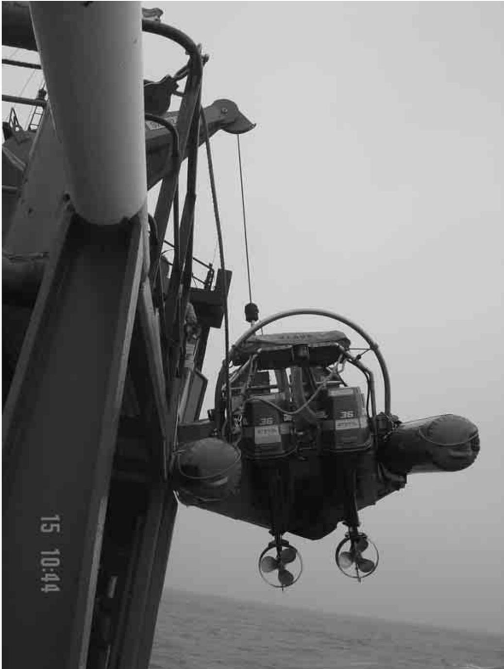
FRC pinned in against the ship's side ready for launch
