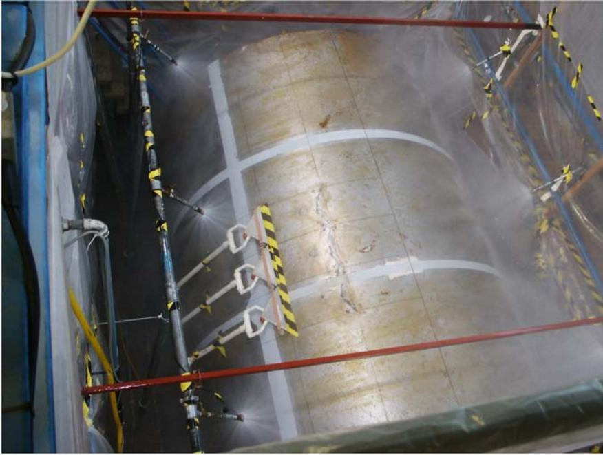
3.0 m diameter tank and 4-row water deluge system. Photograph courtesy of London South Bank University
