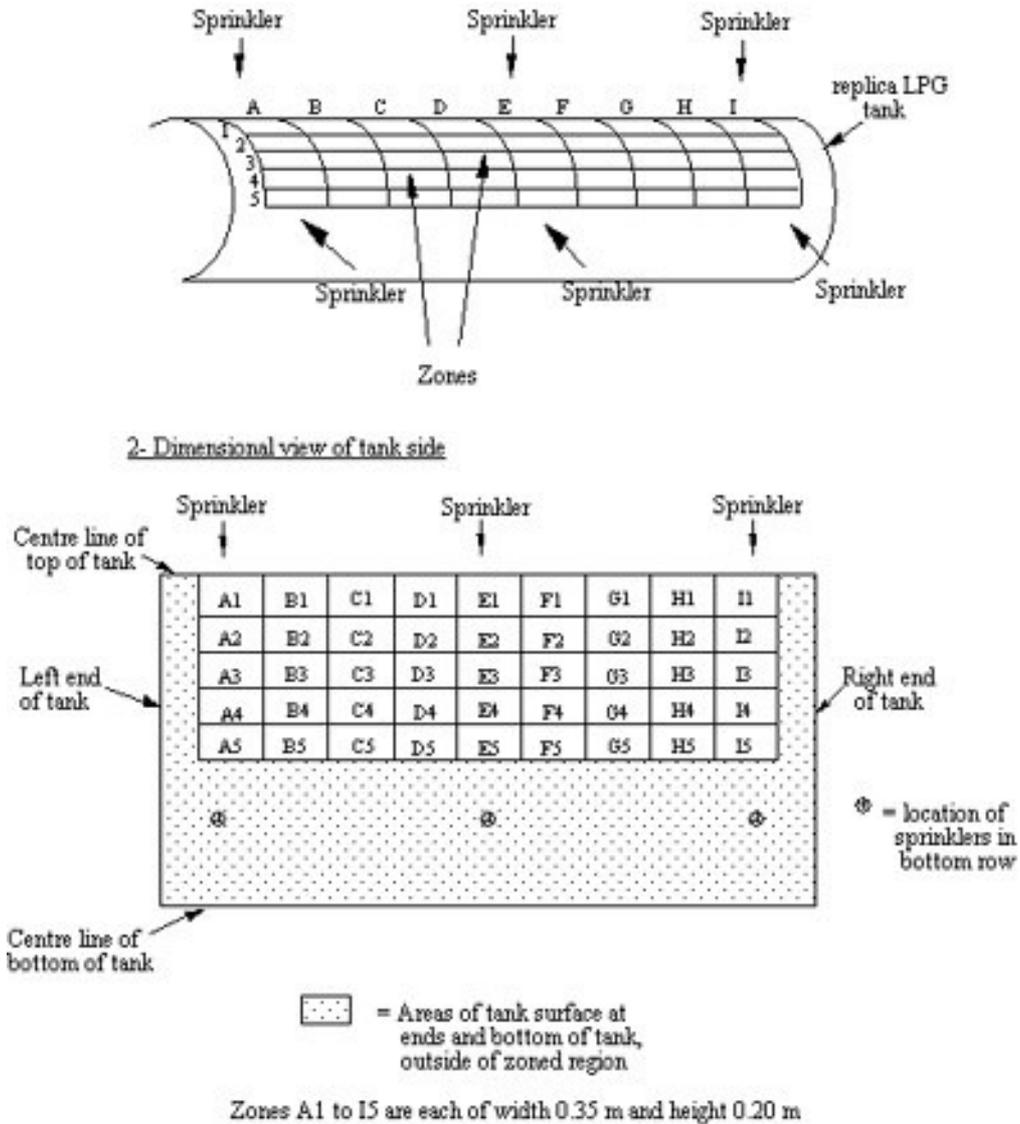
**Figure 2** Schematic showing the division of the replica tank surface into zones
