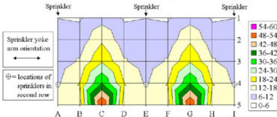
**Figure 6** Water distribution predicted for 2.2 m diameter tank and 5-row deluge using same water deluge settings as for optimum water distribution with 4-row deluge
