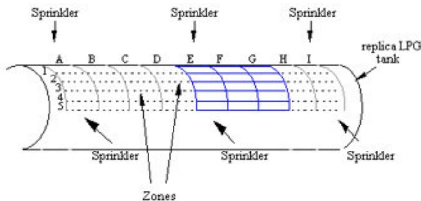
**Figure 3** 15 zone representative region of tank surface for 1.2 m tank and 3-row water deluge
