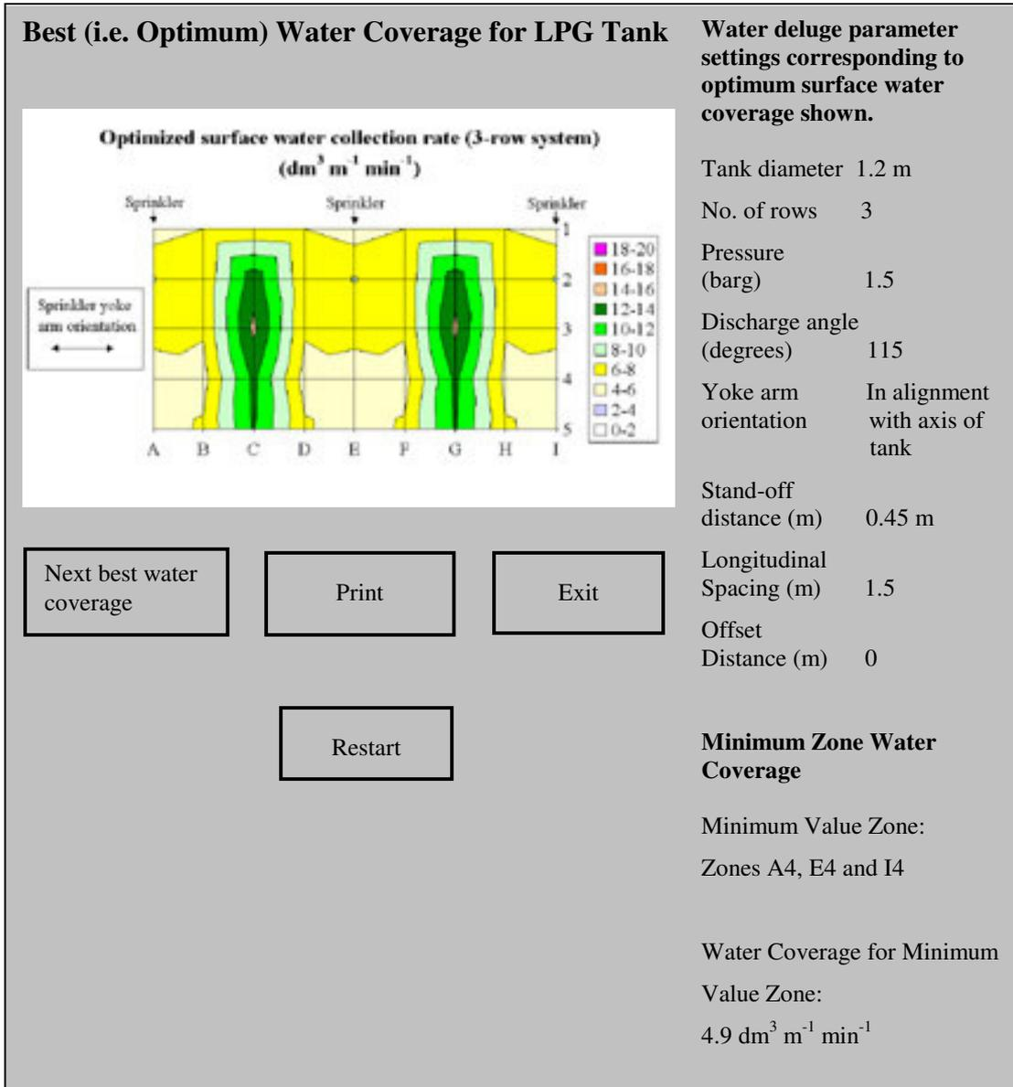
**Figure 11** Typical results output screen displayed by model
