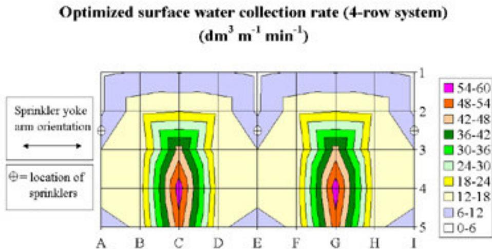
**Figure 7** Optimum water distribution predicted for a 3.0 m diameter tank and 4-row water deluge
