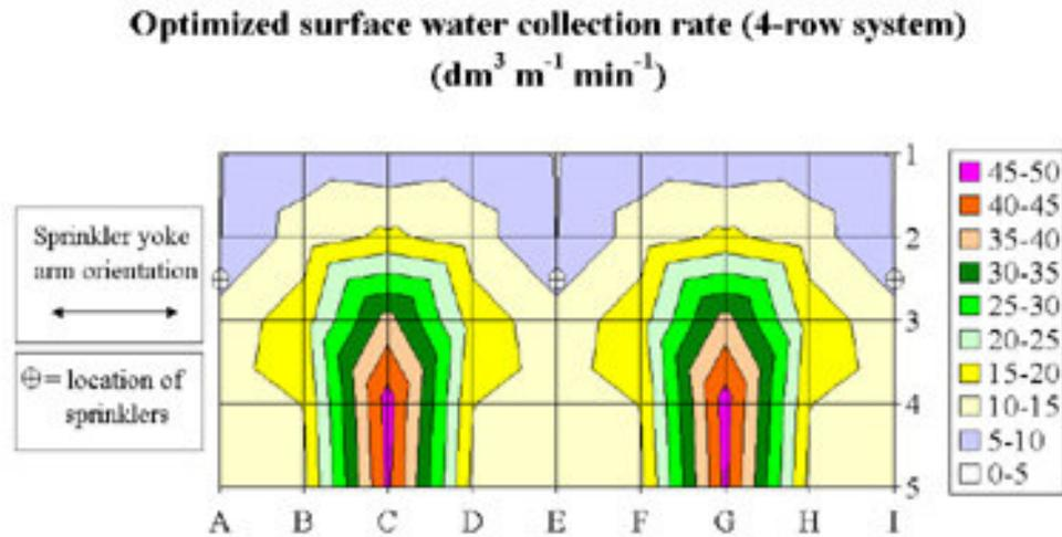
**Figure 8** Predicted water distribution for a 3.0 m diameter tank and 4-row deluge, using the optimum water deluge parameter settings determined for a 2.2 m diameter tank and 4-row deluge system
