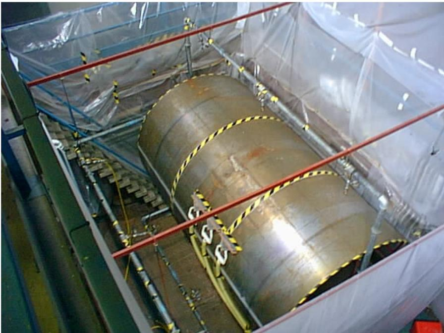
*2.2 m replica LPG tank and pentagonal water deluge system. Photograph courtesy of London South Bank University*
