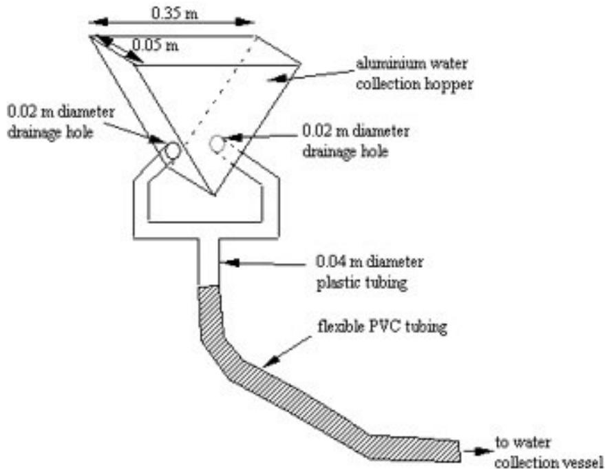
**Figure 1** Schematic of water collection device
