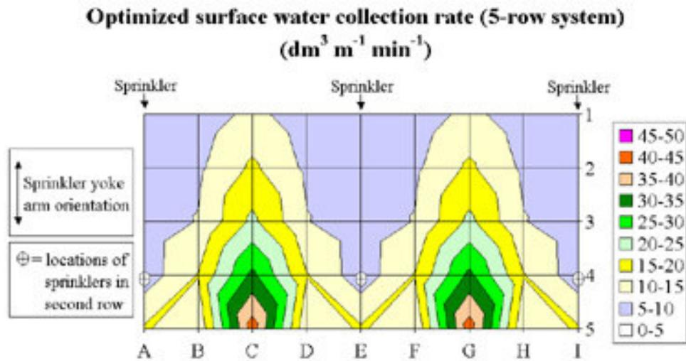
**Figure 4** Optimum water distribution predicted for 2.2 m diameter tank and 5-row deluge
