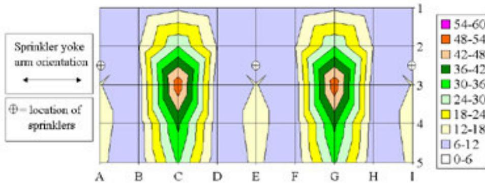
**Figure 5** Optimum water distribution predicted for 2.2 m diameter tank and 4-row deluge
