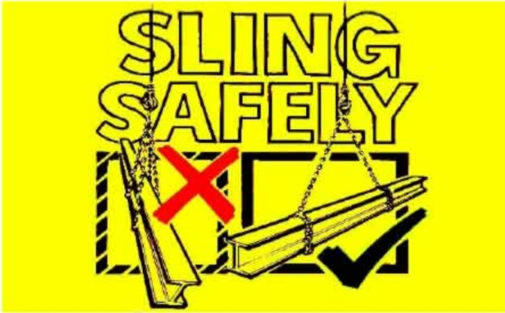
**Figure 9** Message for steel components
