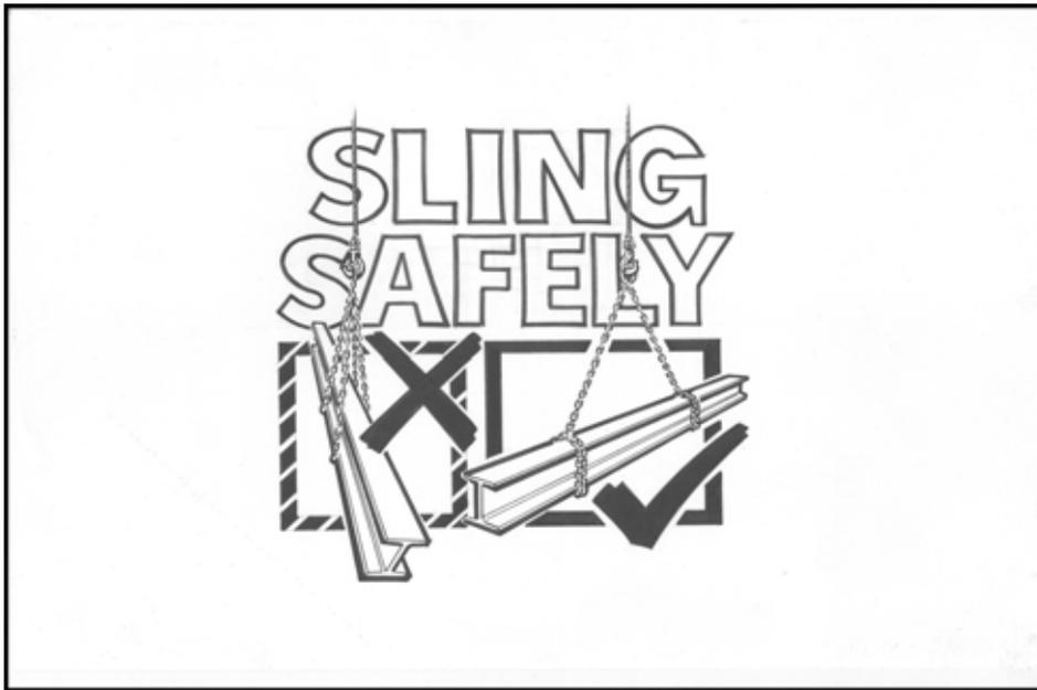
**Figure 4** Safety message for steel frame erection
