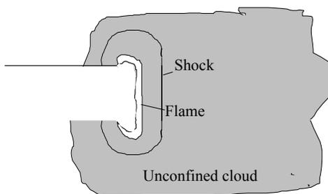
Recently it has been demonstrated that a more serious hazard is presented if a accelerating flame and associated shock front emerges from the pipe. The actual transition mechanism is not clearly understood. The significance is that this mechanism allows mixtures to be detonated that could not be detonated if an established detonation emerged from the pipe.
