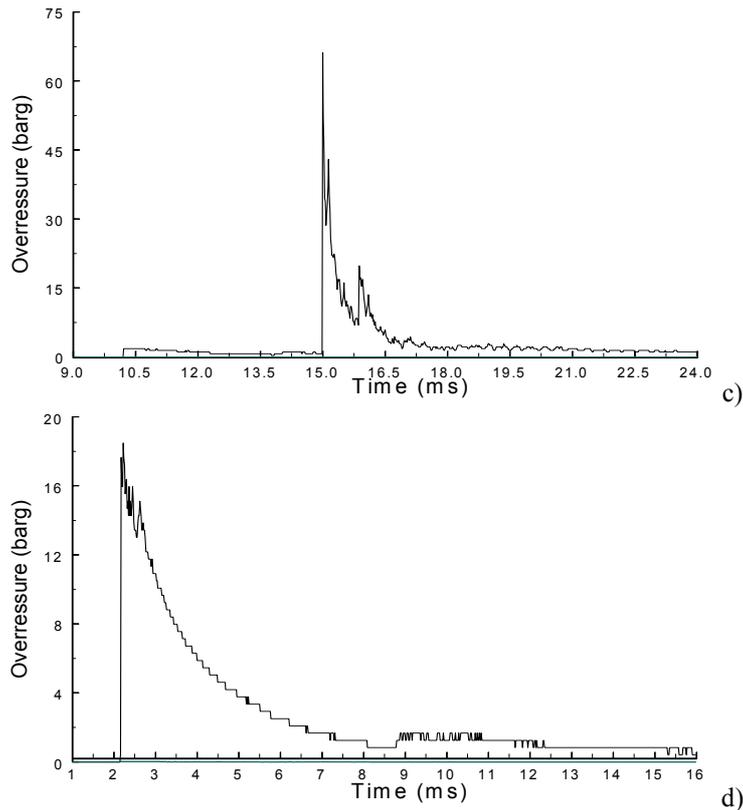
**Figure 4.1.** Typical pressure histories showing a) slow deflagration, b) fast deflagration, c) overdriven detonation and d) steady detonation
