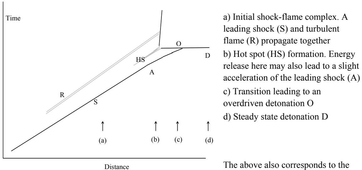
The above also corresponds to the final stages of the low velocity regime in a galloping detonation.
