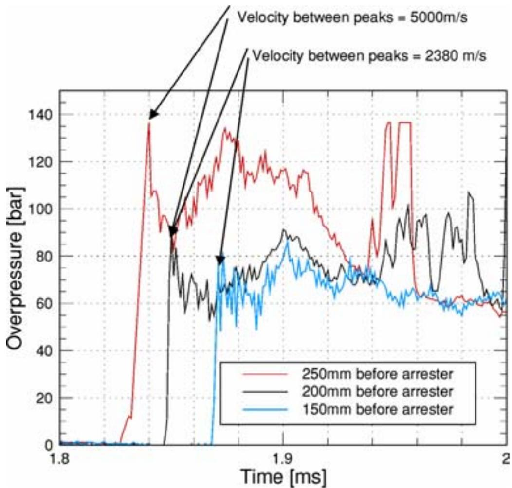
**Figure 6.6.3** Pressure histories from test km8t69. Note that in this case the deflagration to detonation transition is captured, and is occurring in the incident wave
