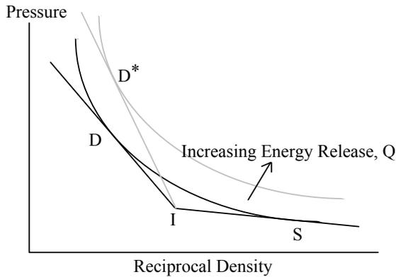
For detonations, a curve can be drawn that links all possible final states. This is called the Rankine-Hugoniot curve. The steady state solution is the point D, where a line drawn from the initial state, I, is a tangent to the Rankine-Hugoniot curve.
