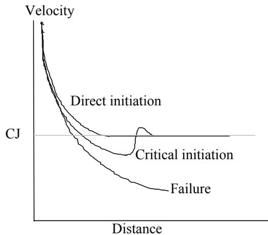
initiates the chemical reaction and sustains it until the detonation structure gives rise to a self-sustaining detonation. As the source strength decreases, or the mixture becomes less reactive, a point is reached where the source only just manages to initiate the detonation. In this case clear separation of the leading shock front and reaction can be seen. This is usually followed by a localised explosion in the shocked gas which then leads to an initiation. The velocity
