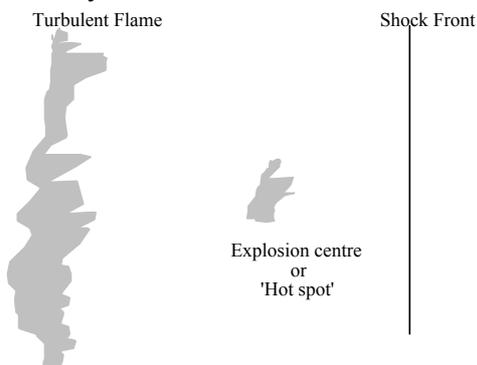
combustion to a point where a shock wave is formed ahead of the flame front.
