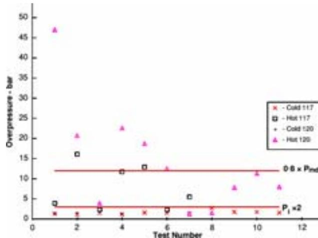
**Figure 6.5.2** Temperature effects on the flame acceleration in a 40 mm tube. Initial cold temperature is 6 - 7 centigrade; the hot tests were with a short zone if the tube heated to between 30 and 50 centigrade
