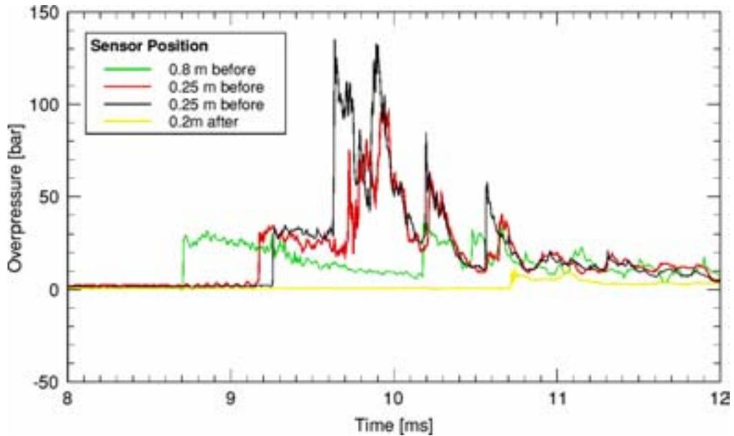
**Fig 6.6.4** Transition to detonation in reflected wave
