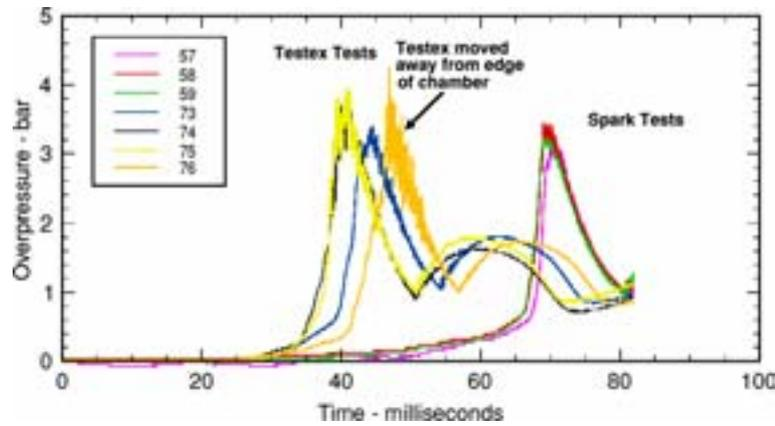
**Figure 6.3.1** Comparison of pressure histories from different ignition sources – IIB3 mixture.
