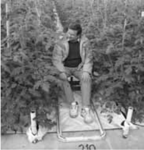
Low level seat running on heating pipes
