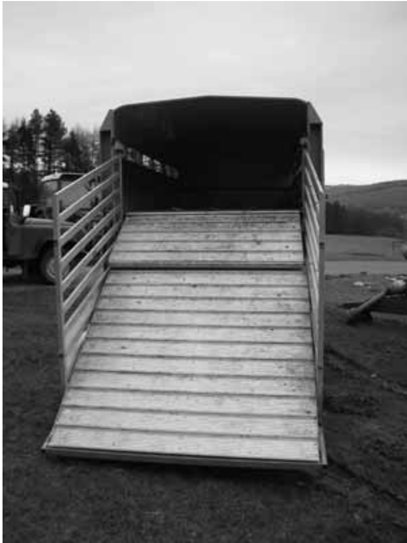
Modern twin deck livestock trailer with lightweight aluminium ramp
