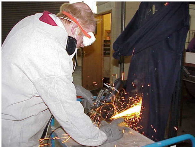
Figure 1. Grinder sparks being applied to manikin (FR “Proban” cotton boiler suit). No ignition occurred after five minutes of sustained application of the sparks
