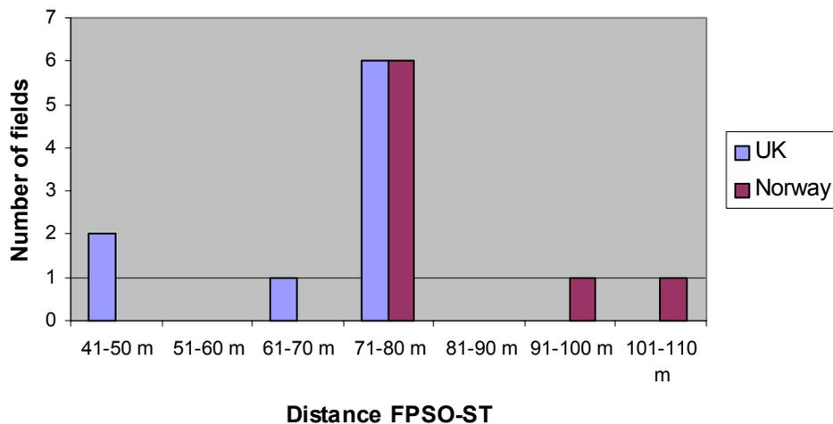
**Figure 5 Overview of off-loading distances between FPSO and ST**
