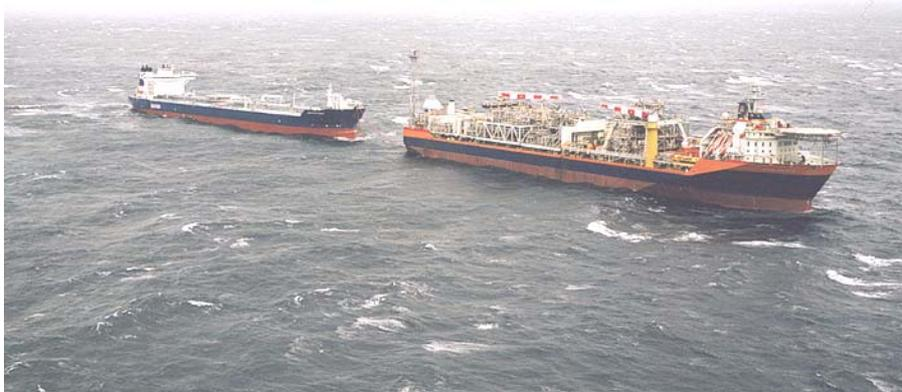
**Figure 1 Example of FPSO and shuttle tanker configuration**
