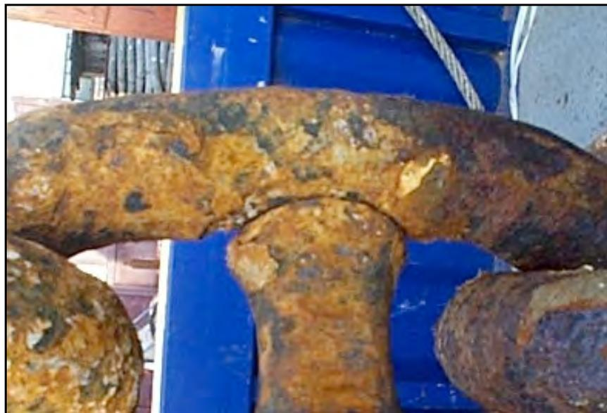
Figure 4-8 - Typical Corrosion Pattern on a chain after a Long Deployment
