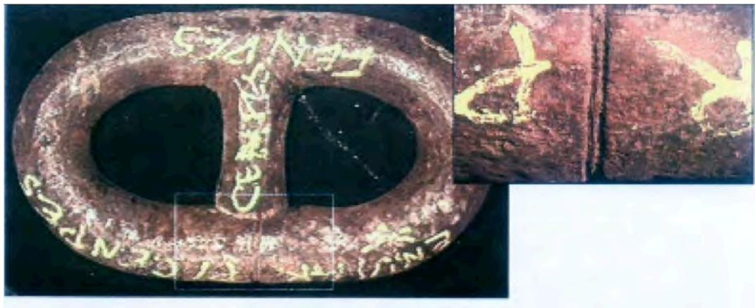
**Figure 4-6 - Examples of HAZ Corrosion on a Chain Link, from a M.Sc. Dissertation in 2003 from Pontificia Universidade Catolica do Rio de Janeiro [Ref 8]**
