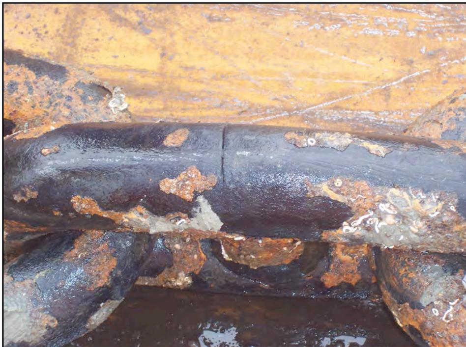
**Figure 4-2 - Example of “Black” Coloured Chain on the Back Deck of and Anchor Handling Tug**
