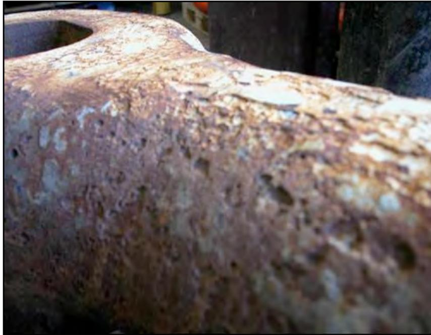
**Figure 4-9 - Example of the Corrosion Pattern on a Shackle Body After a Long Deployment**
