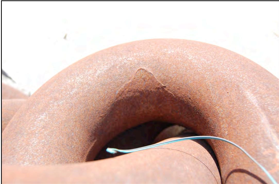
**Figure 5-2 - Example of a Fairly Pronounced Witness Mark Showing the Chain Has Been Tensioned**
