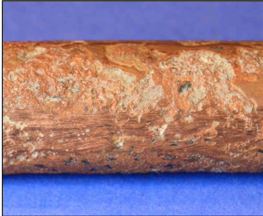
Figure 4-7 Example of stray current corrosion on a copper water pipe (ref. <http://metallurgist.com/html/Definitions/StrayCurrentCorrosion.htm>)
