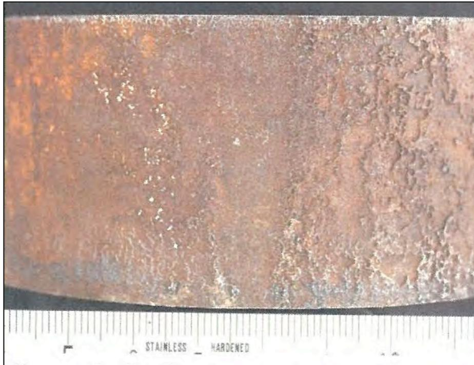
Figure 4-1: Corrosion pattern from case 1
