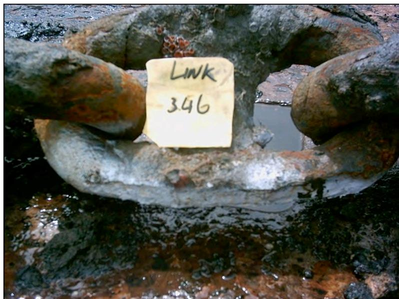
Figure 4-4: Corrosion pattern from case 4 showing significant loss of material
