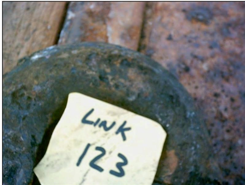
Figure 4-3: Corrosion pits among black patches from case 4
