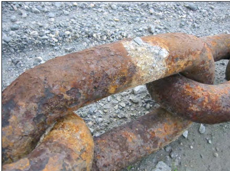
Figure 4-5: Link with corrosion pits with black patches from Case 5
