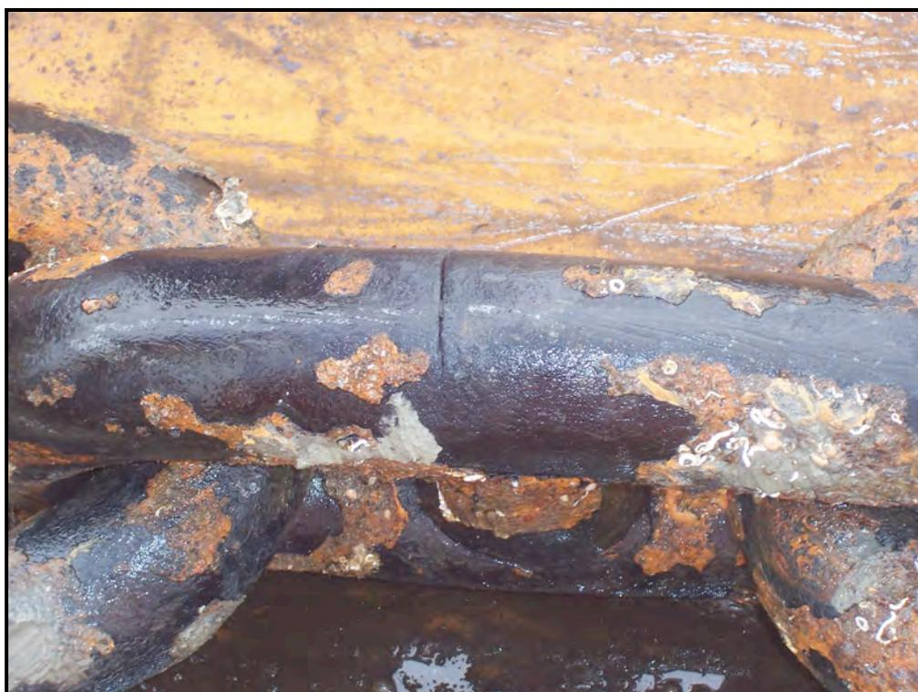
**Figure 3-6: Black Coloured Link when first recovered on the back of an Anchor Handling Tug**
