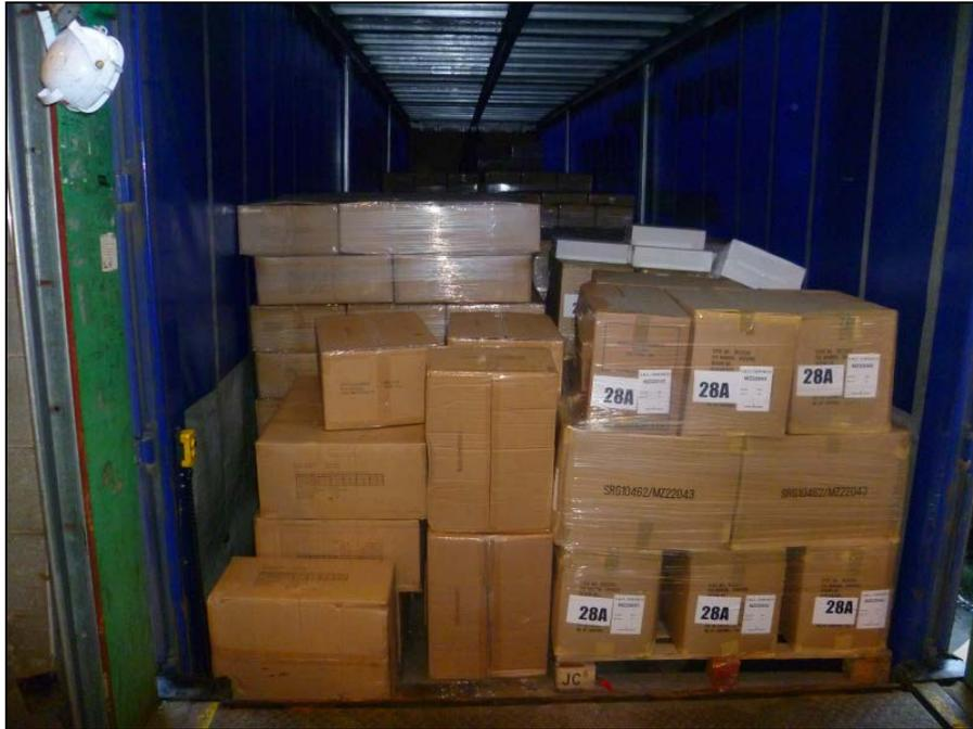
**Figure 9: Unsecured palletised load in a curtain-sided vehicle**
