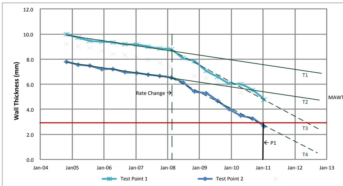
**Figure 9. Simulated vessel wall thickness data trends including change in deterioration rate**
