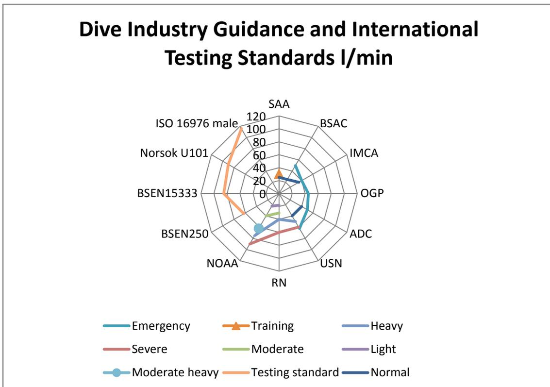
Figure 4. Graph of dive industry and standard recommended surface breathing rates and test rates for diving equipment in l/min.
