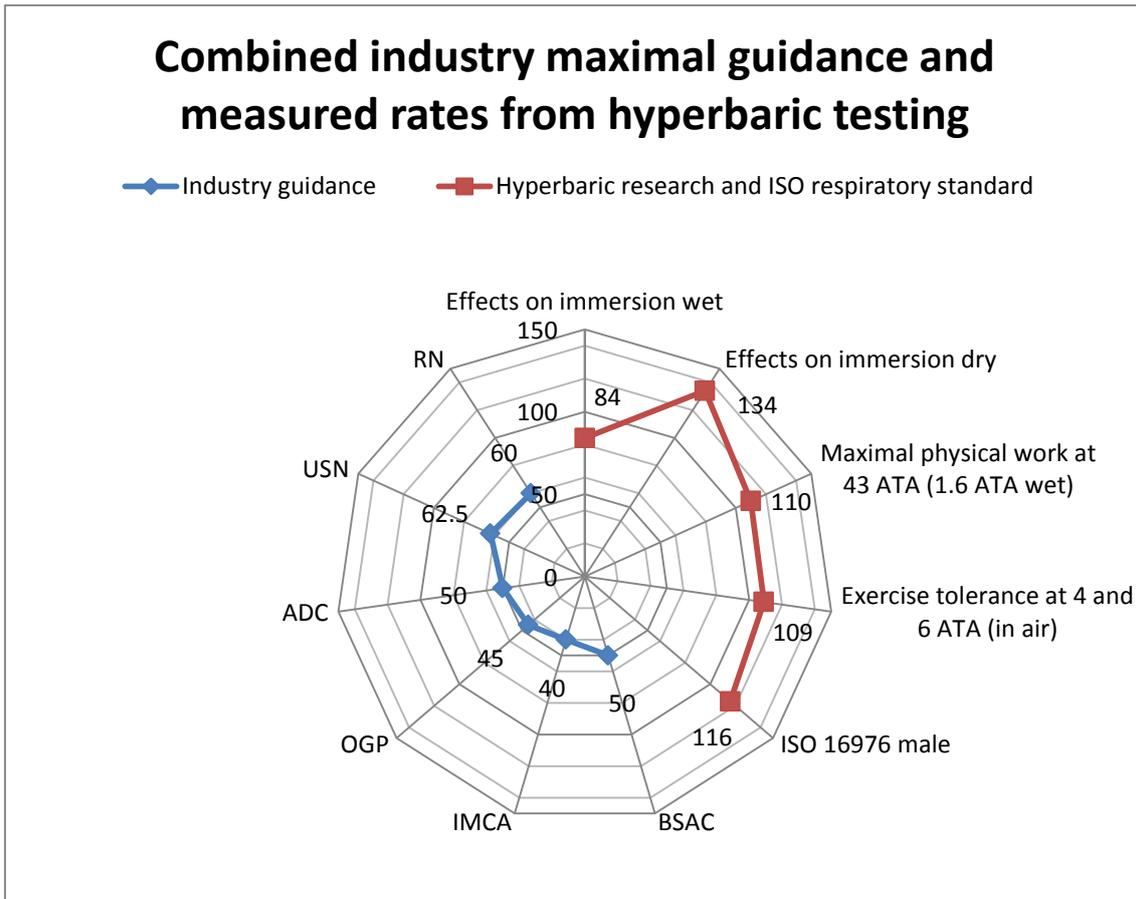
Figure 5. Combined scientific research and industry guidance surface breathing rates in l/min.
