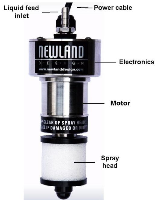
Figure 2. The Newland electric rotary atomiser
