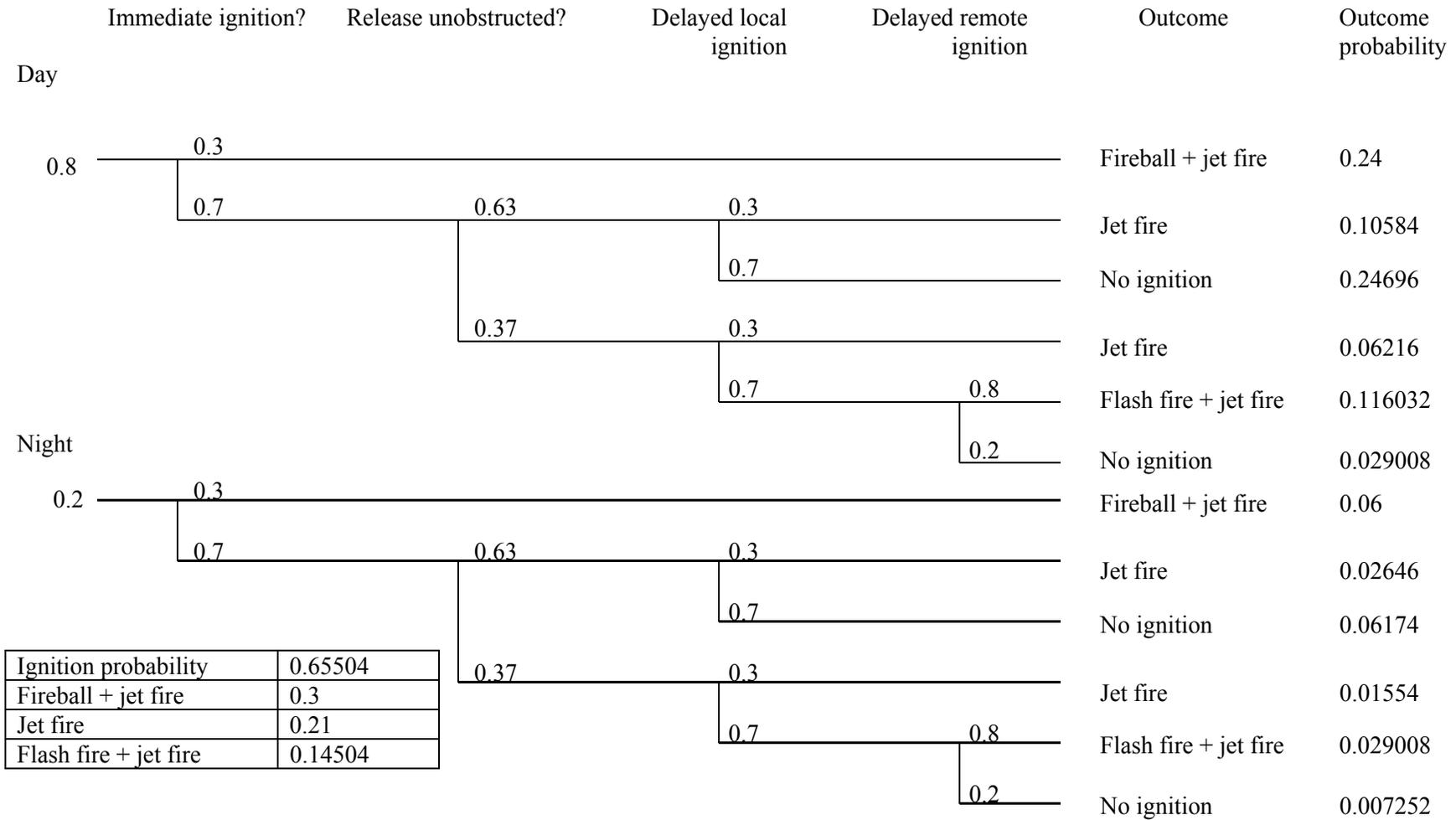
**Figure 9** Event tree 2 – R12 substances with minimum ignition energies  $\geq 0.2$  mJ
