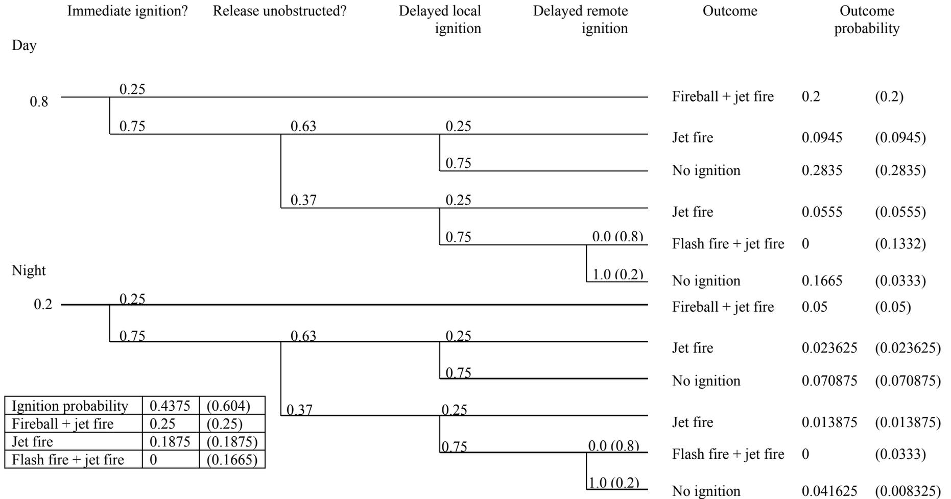
**Figure 10** Event tree 3 – Natural gas event tree. The values in brackets can be used for R11 and low reactive materials
