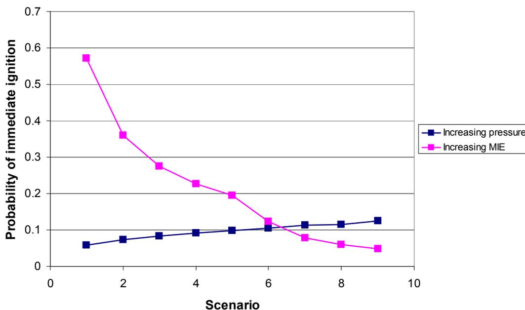
**Figure 7** The blue line illustrates how the probability of immediate ignition varies with increasing pressure (constant minimum ignition energy) and the pink line with increasing minimum ignition energy (constant source pressure). Note that the pink line is completely independent from the blue line, i.e., the pink scenario 1 does not correspond to the blue scenario 1 and so on.
