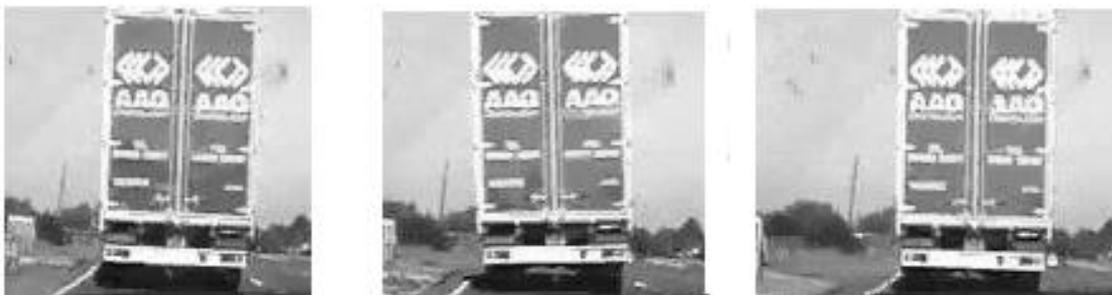
**Figure 15** Lorry sway while driving over a bump: frame times at (from left) 2207s, 2207.5s and 2208s (see also figure 16)
