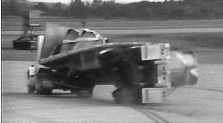
**Figure 1** A typical rollover where the trailer tips over first and pulls the tractor unit over afterwards [reproduced from ref.12 with permission of the author]
