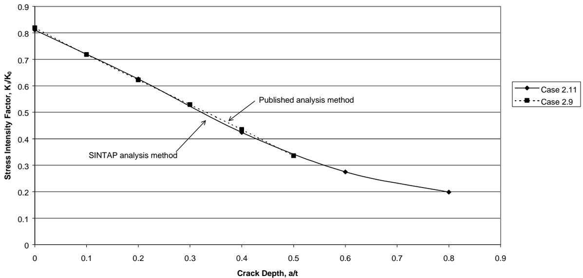
Fig. 20. Normalised SIF at deepest point of short surface crack at toe of T-butt weld. Comparison of SIFs with different analysis methods with aspect ratio 3.33
