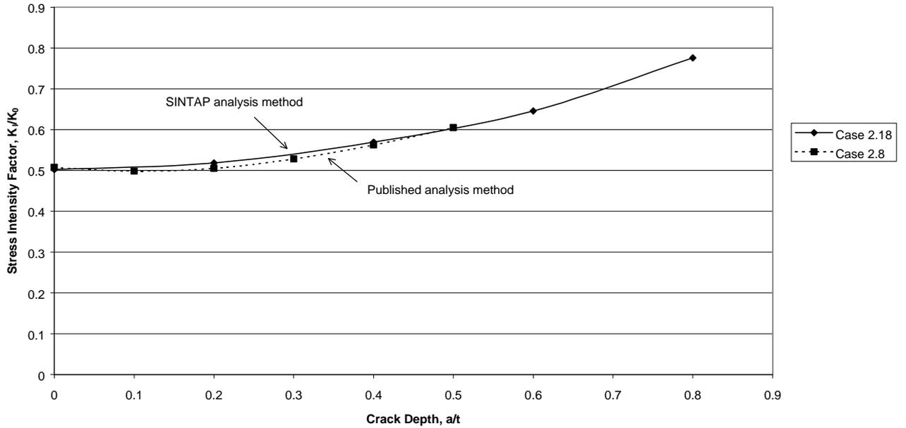
Fig. 19. Normalised SIF at surface intersections of short surface crack at toe of T-butt weld. Comparison of SIFs for different analysis methods with aspect ratio 10.
