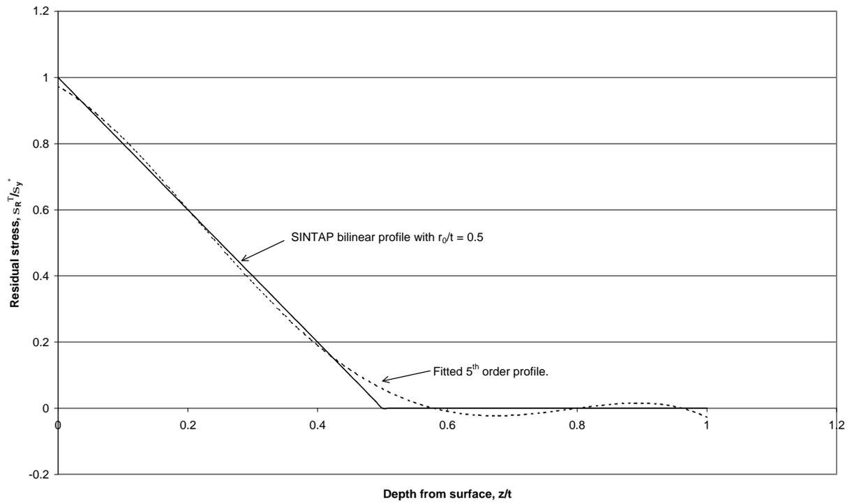
Fig. 11. Through wall distribution of transverse residual stresses at toe of T-butt weld. Comparison of SINTAP and fitted profiles.
