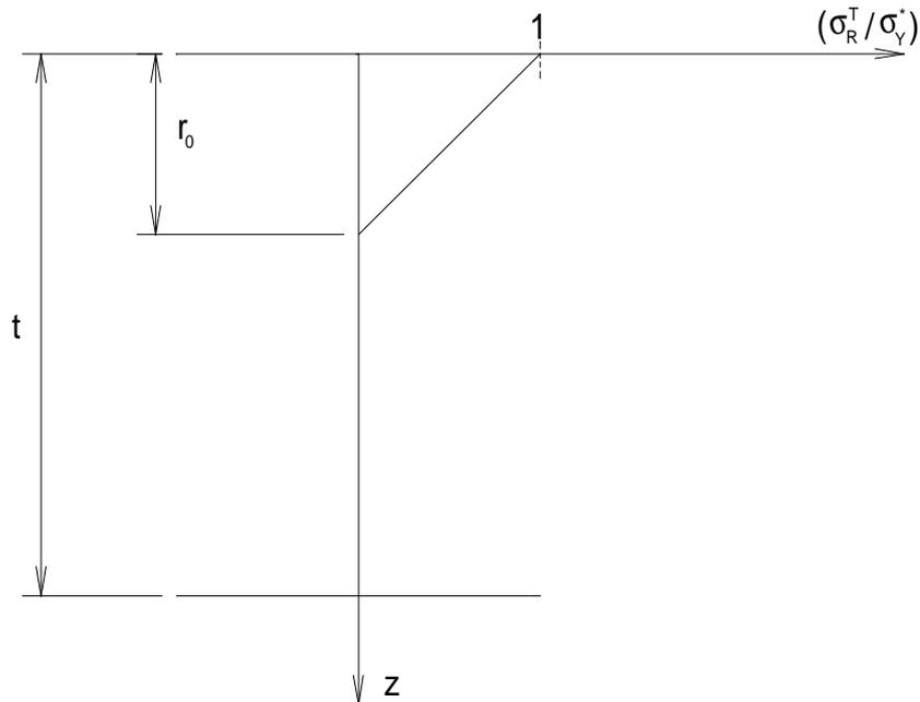
Fig. 10. SINTAP recommended through-thickness bilinear profile of transverse stresses in base plate at toe of T-butt weld.
