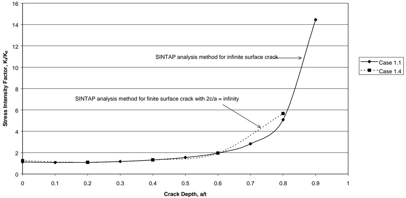
Fig. 3. Normalised SIF at longitudinal infinite surface crack at butt weld in plate. Effect of analysis method.
