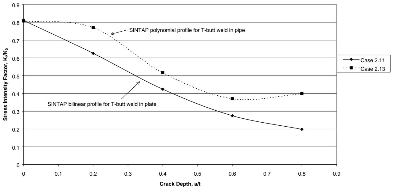
Fig. 22. Normalised SIF at deepest point of short surface crack at toe of T-butt weld. Comparison of SIFs for SINTAP profiles for T-butt welds in plate and pipe.
