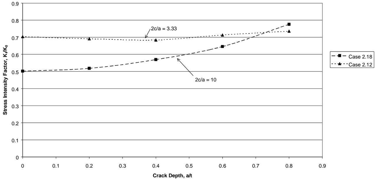
Fig. 17. Normalised SIF at surface intersections of short surface crack at toe of T-butt weld. Effect of aspect ratio.
