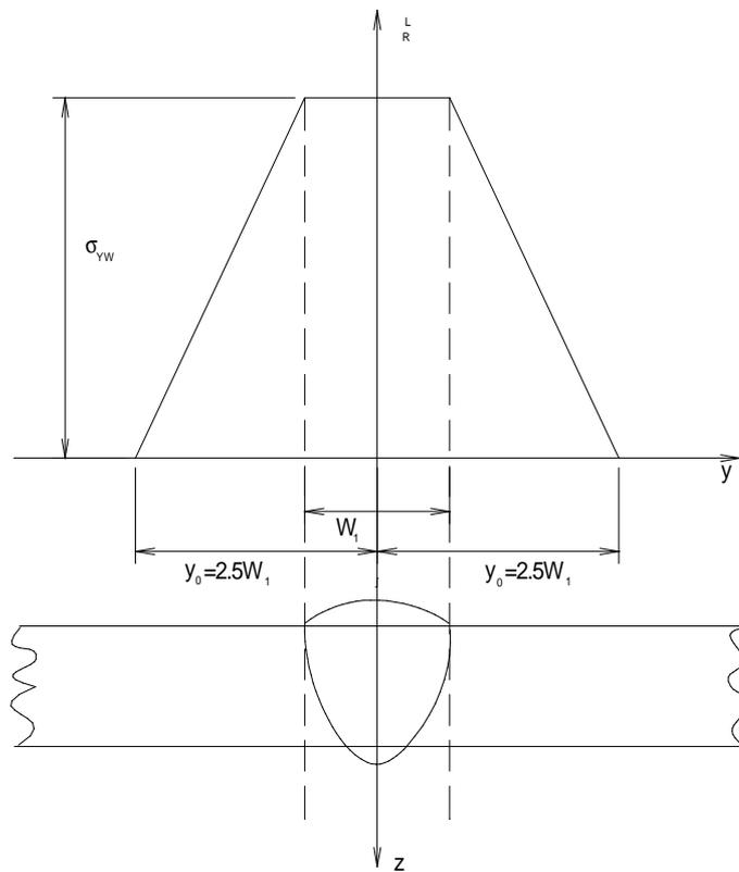
Fig. 2. Profile of longitudinal residual stresses at butt weld in plate.
