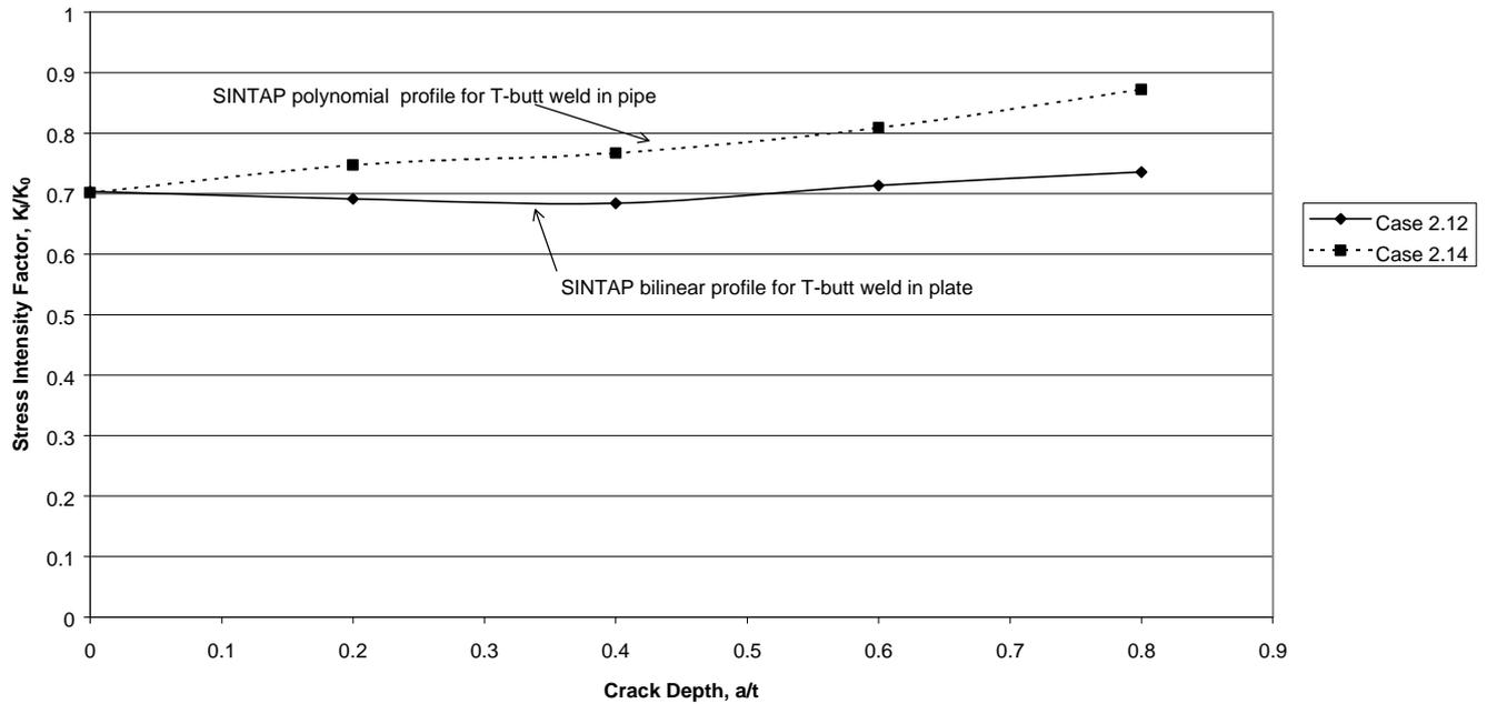
Fig. 23. Normalised SIF at surface intersections of short surface crack at toe of T-butt weld. Comparison of SIFs for SINTAP profiles for T-butt welds in plate and pipe.
