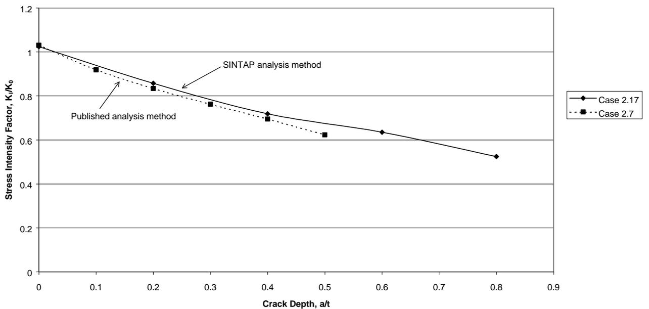
Fig. 18. Normalised SIF at deepest point of short surface crack at toe of T-butt weld. Comparison of SIFs for different analysis methods with aspect ratio = 10.
