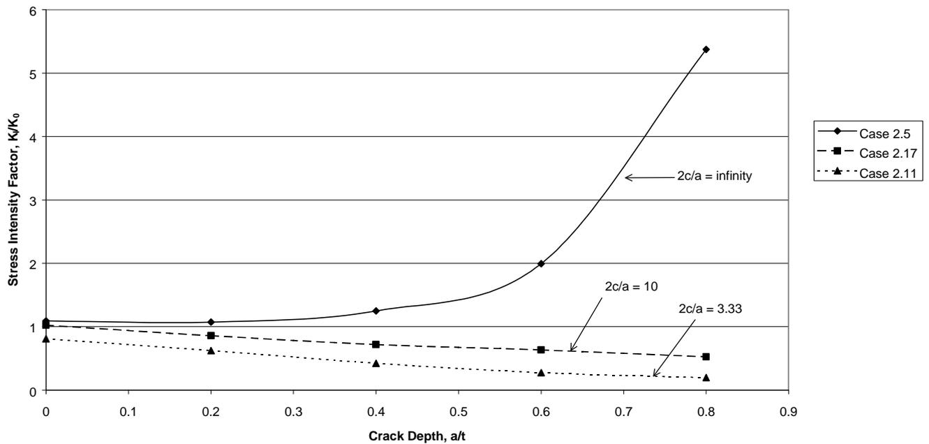
Fig. 16. Normalised SIF at deepest point of short surface crack at toe of T-butt weld. Effect of aspect ratio.
