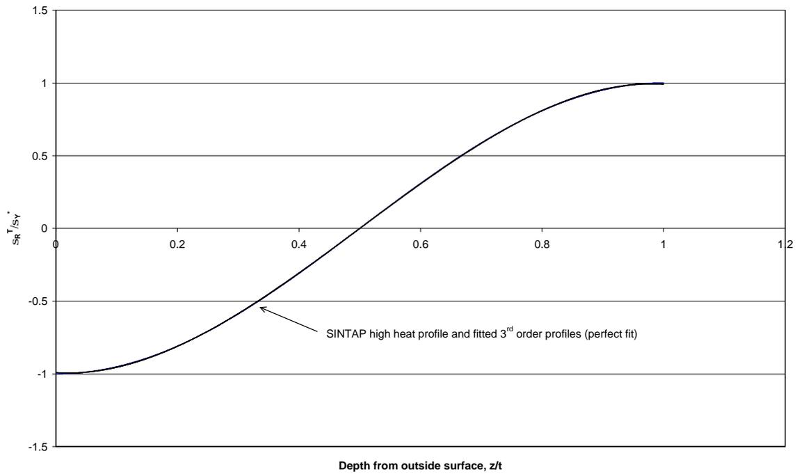
Fig. 27. Through-thickness profile of transverse residual stresses at high heat input pipe butt weld. Comparison of SINTAP profile and fitted 3<sup>rd</sup> order profile.
