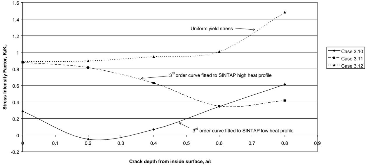
Fig. 31. Normalised SIF at part circumferential crack at inside surface of pipe. Comparison of SIFs for different residual stress profiles.
