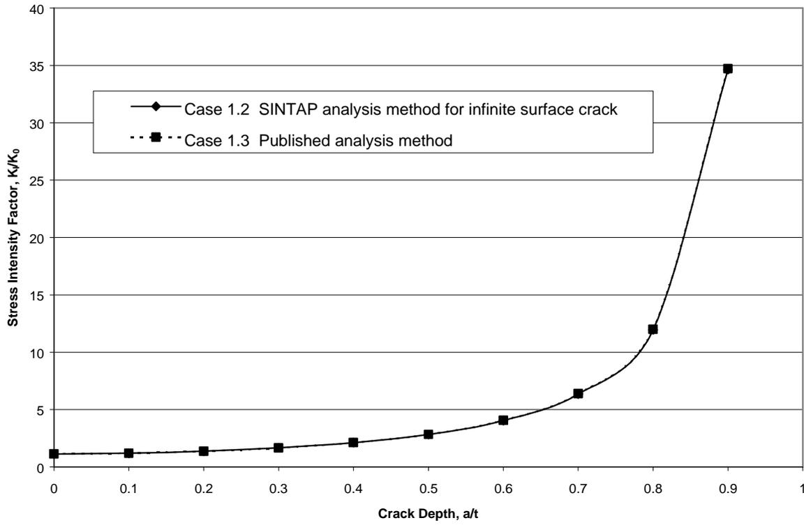
Fig. 5. Normalised SIF at longitudinal infinite surface crack at butt weld in plate. Effect of analysis method.
