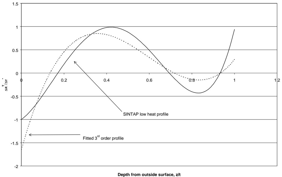
Fig. 26. Through thickness profile of transverse residual stress at low heat input pipe butt weld. Comparison of SINTAP profile and fitted 3<sup>rd</sup> order profile.
