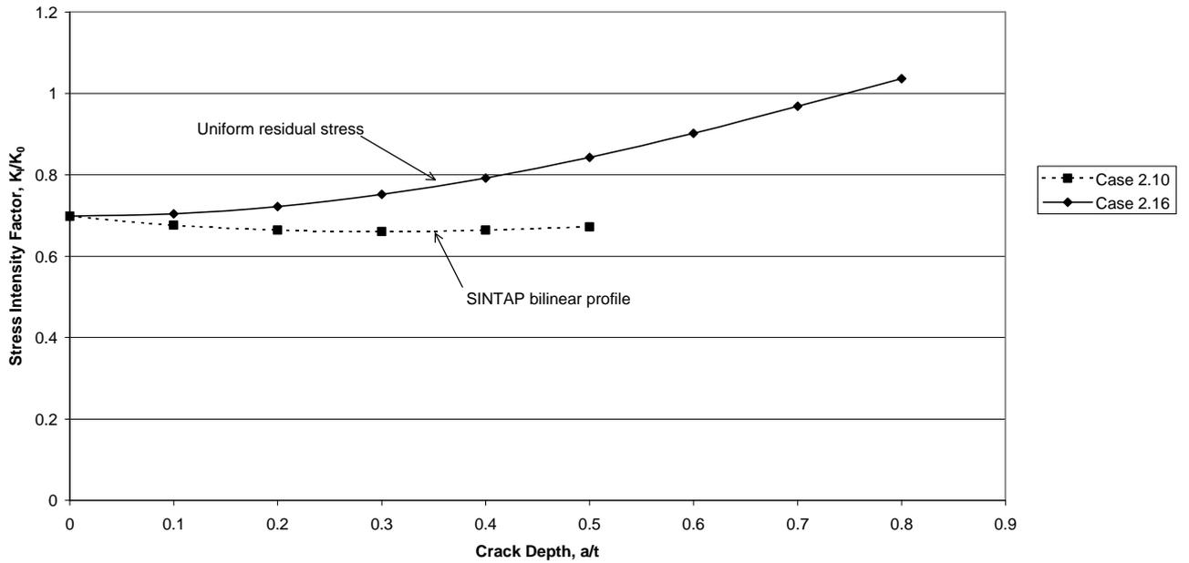
Fig. 25. Normalised SIF at surface intersections of short surface crack at toe of T-butt weld Comparison of SIFs for different residual stress profiles.
