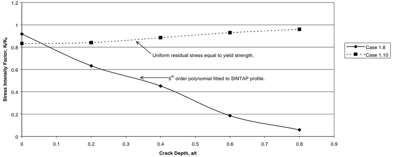
Fig. 7. Normalised SIF at deepest point of finite surface crack at butt weld in plate. Effect of residual stress profile.
