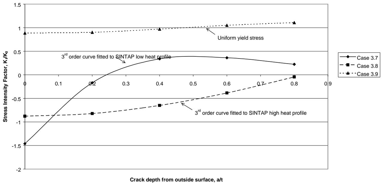
Fig. 30. Normalised SIF at part circumferential crack at outside surface of pipe. Comparison of SIFs for different residual stress profiles.
