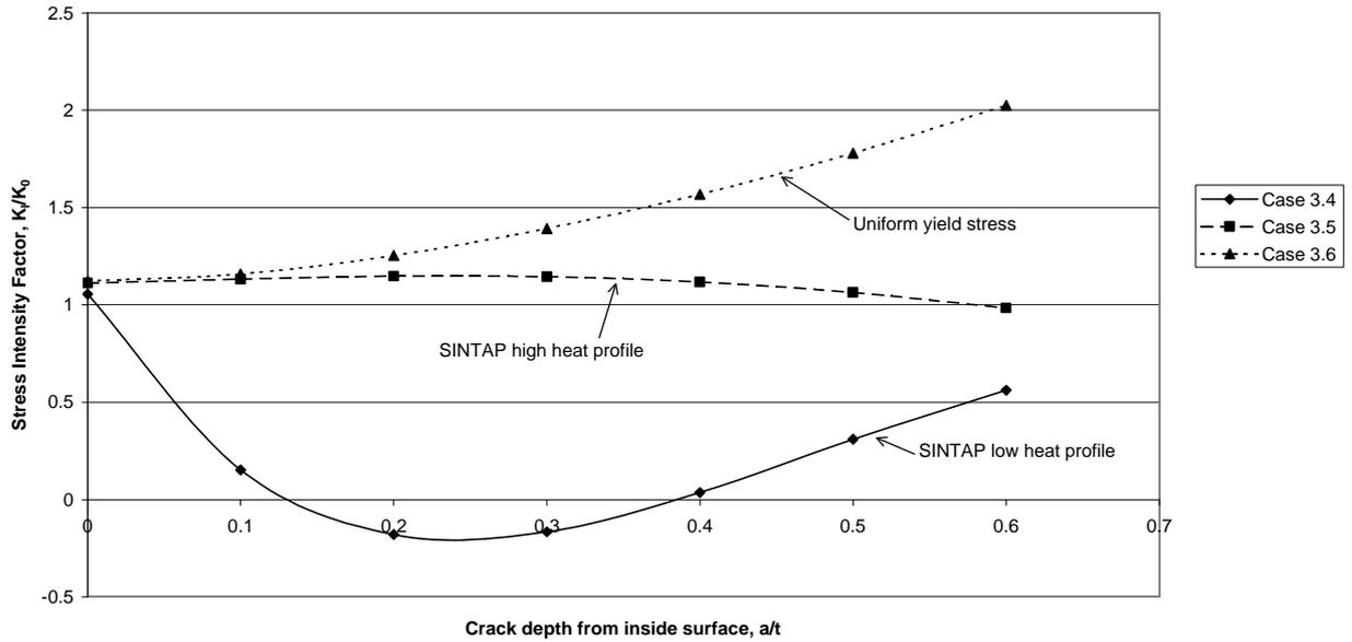
Fig. 29. Normalised SIF at fully circumferential crack at inside surface of pipe. Comparison of SIFs for different residual stress profiles.
