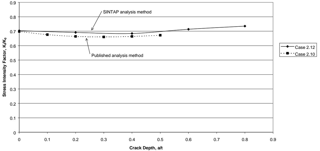
Fig. 21. Normalised SIF at surface intersections of short surface crack at toe of T-butt weld. Comparison of SIFs for different analysis methods with aspect ratio 3.33
