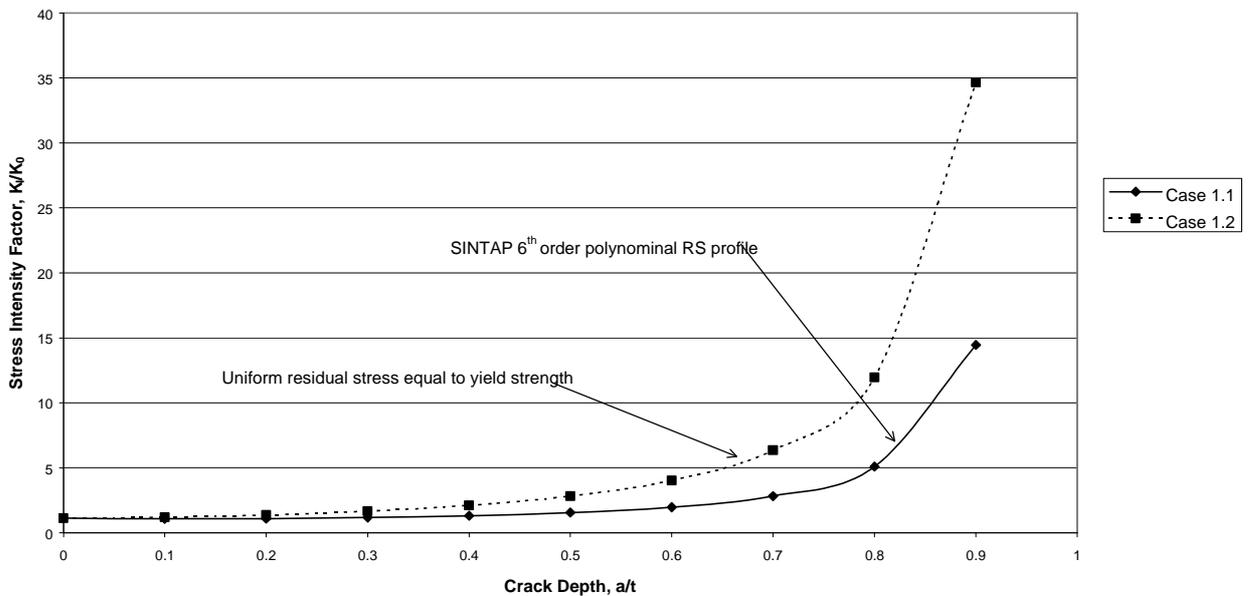
Fig. 4. Normalised SIF at longitudinal infinite surface crack at butt weld in plate. Effect of residual stress profile.
