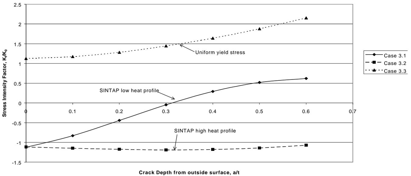
Fig. 28. Normalised SIF at fully circumferential crack at outside surface of pipe. Comparison of SIFs for different residual stress profiles.
