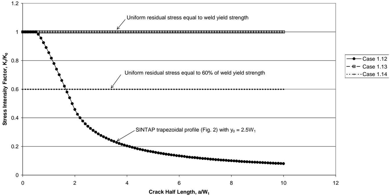
Fig. 9. Normalised SIF at transverse through thickness crack at butt weld in plate. Effect of residual stress profile.
