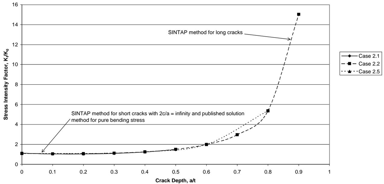
Fig. 13. Normalised SIF at long surface crack at toe of T-butt weld. Comparison of solution methods.
