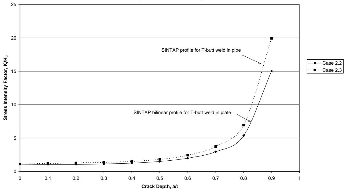
Fig. 14. Normalised SIF at long surface crack at toe of T-butt weld. Comparison of SIFs for SINTAP profiles for T-butt welds in plate and pipe.
