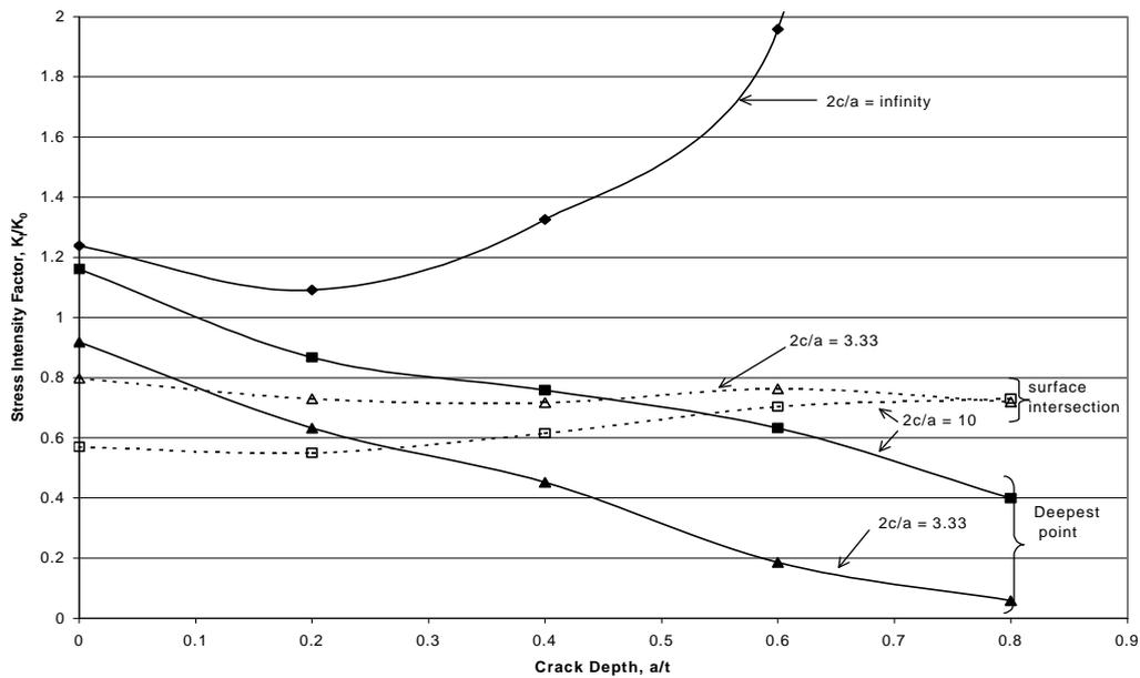
Fig. 6. Normalised SIF at finite surface crack at butt weld in plate. Effect of crack aspect ratio at deepest point and surface intersection.
