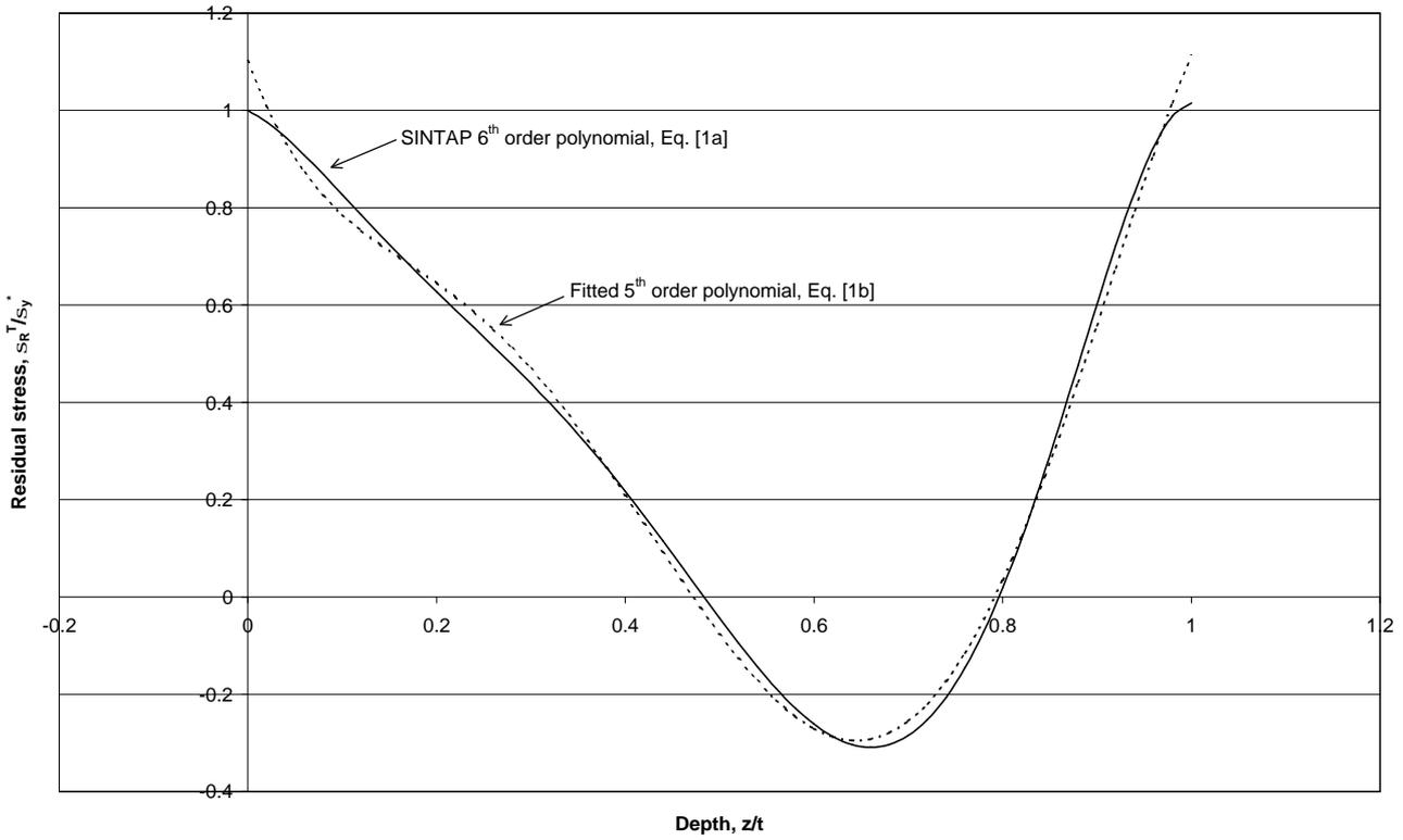
Fig. 1. Through thickness profiles of transverse residual stress at butt weld in plate.
