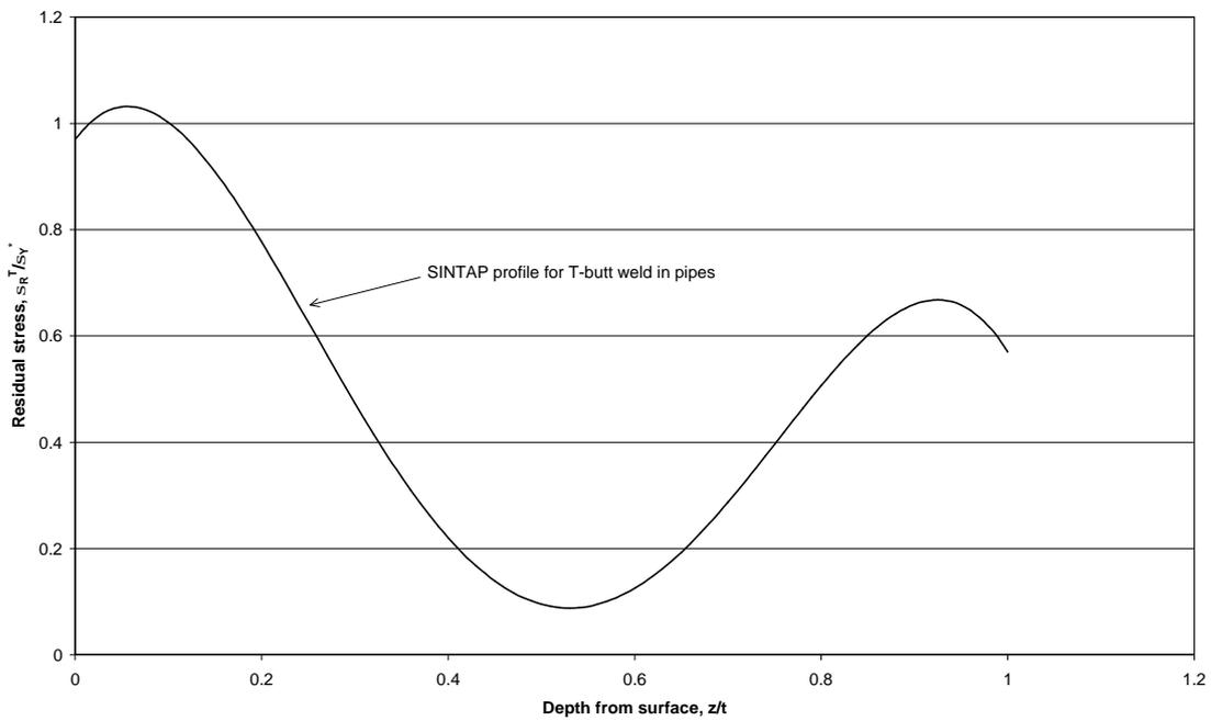
Fig. 12. Through wall distribution of transverse residual stresses at toe of T-butt weld.
