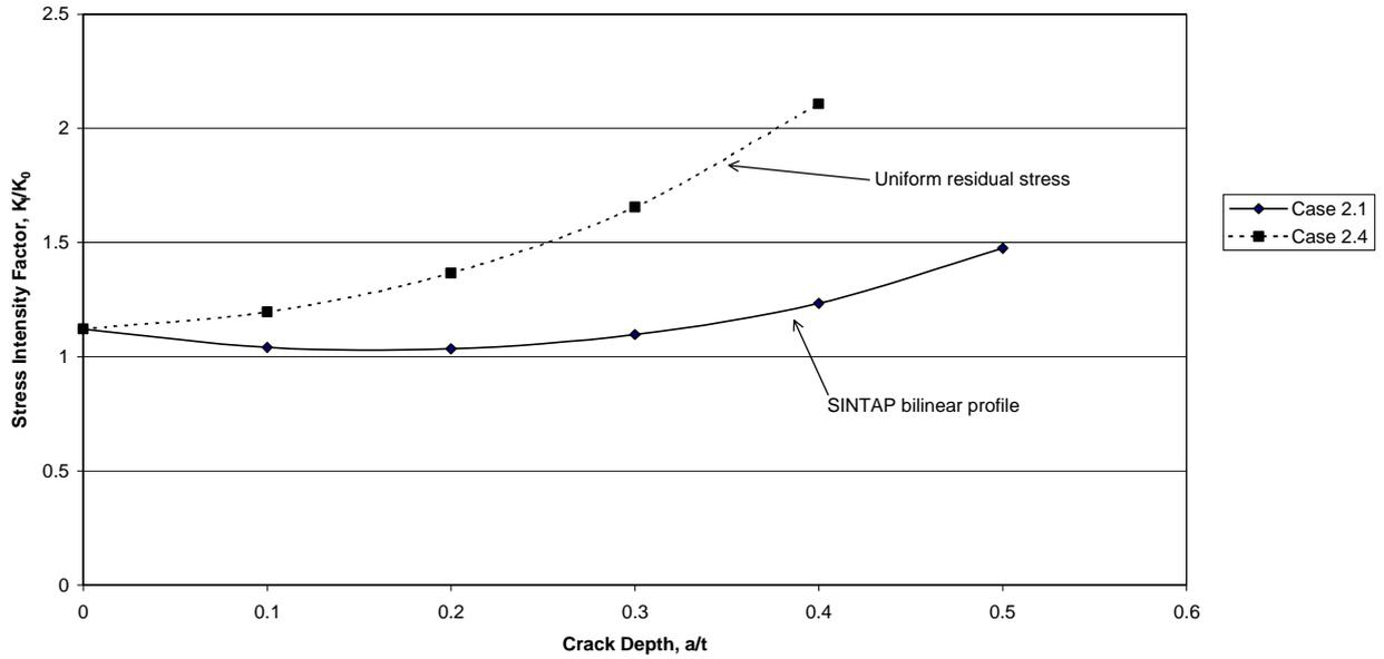
Fig. 15. Normalised SIF at long surface crack at toe of T-butt weld. Comparison of SIFs for different residual stress profiles.
