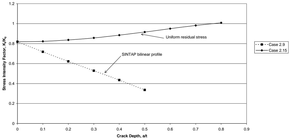
Fig. 24. Normalised SIF at deepest point of short surface crack at toe of T-butt weld. Comparison of SIFs for different residual stress profiles.
