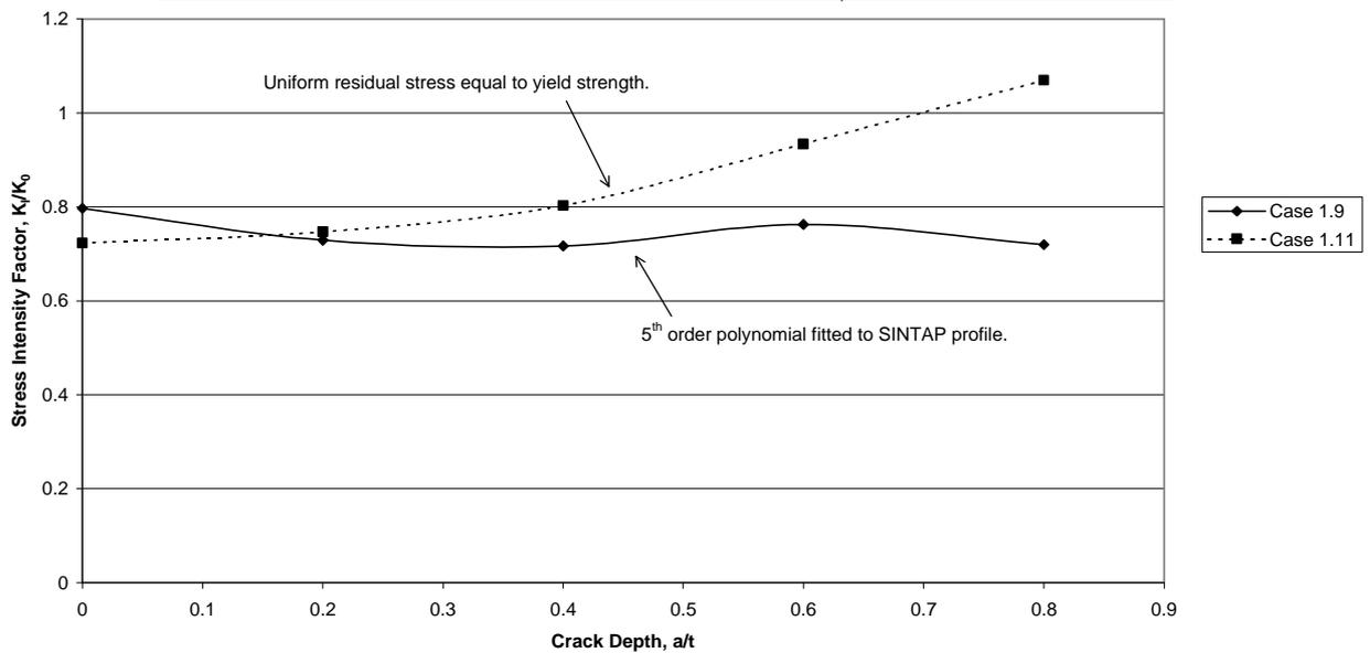
Fig. 8. Normalised SIF at surface intersections of finite surface crack at butt weld in plate. Effect of residual stress profile.
