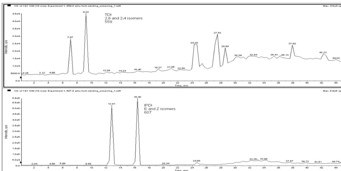
Figure 4. Comparison of chromatograms obtained using Hypercarb 2 (upper) and C18 (lower) methods for an air sample taken during spot welding of polyurethane painted car part.
