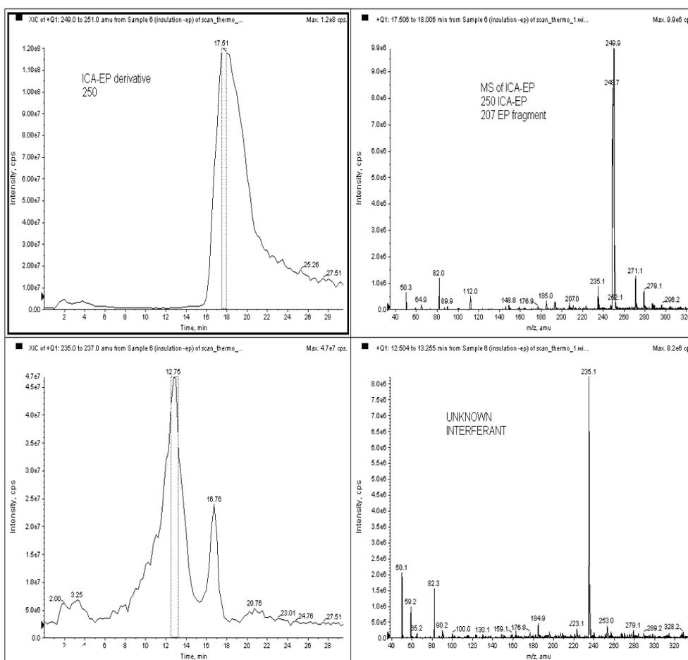
Figure 7. Chromatogram of air sample obtained on an EP coated GF/A during the pyrolysis of spray (insulation) foam – Scan mode MS.
