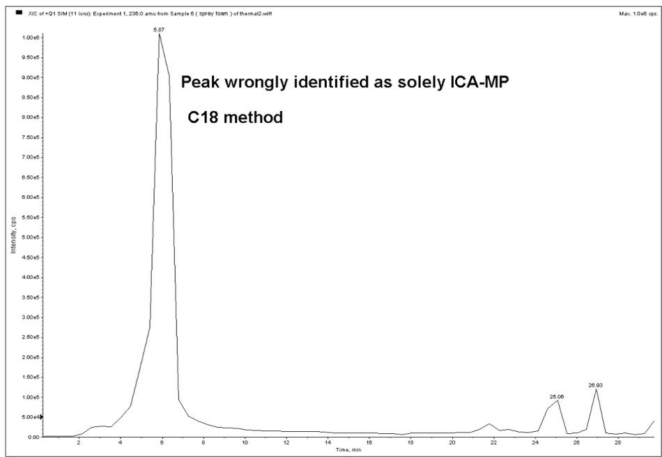
Figure 6a. Comparison of chromatograms obtained for the peaks identified as ICA-MP using the C18 SIM method for pyrolysed insulation (spray) foam.
