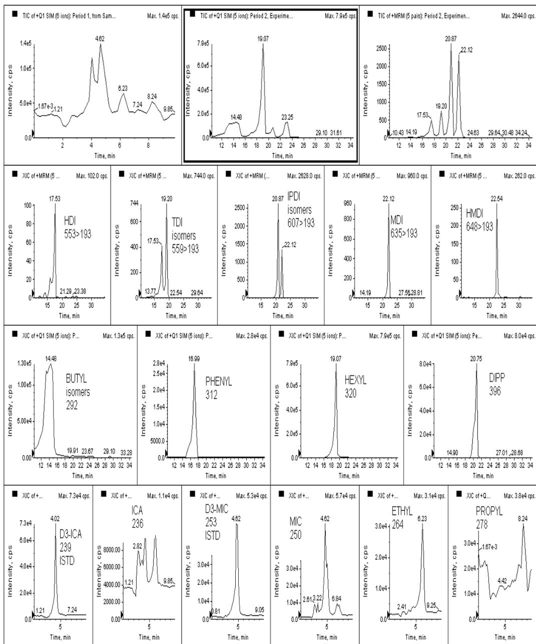
Figure 2. Example chromatograms for C18 screening method (spiked filter)
