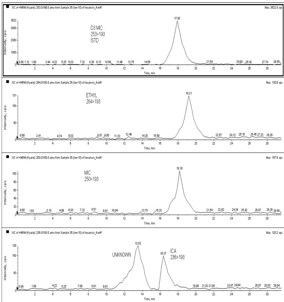
Figure 3. Example MRM chromatograms for Hypercarb 2 method (spiked filter).
