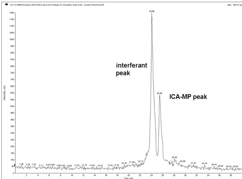
Figure 6b. Comparison of chromatograms obtained for the peaks identified as ICA-MP using the Hypercarb 2 MRM method for pyrolysed insulation (spray) foam.
