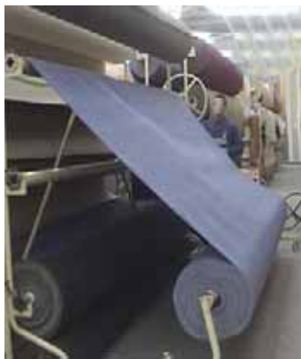
Figure 14. Winding on a new roll using carpet manipulator and wheel.
