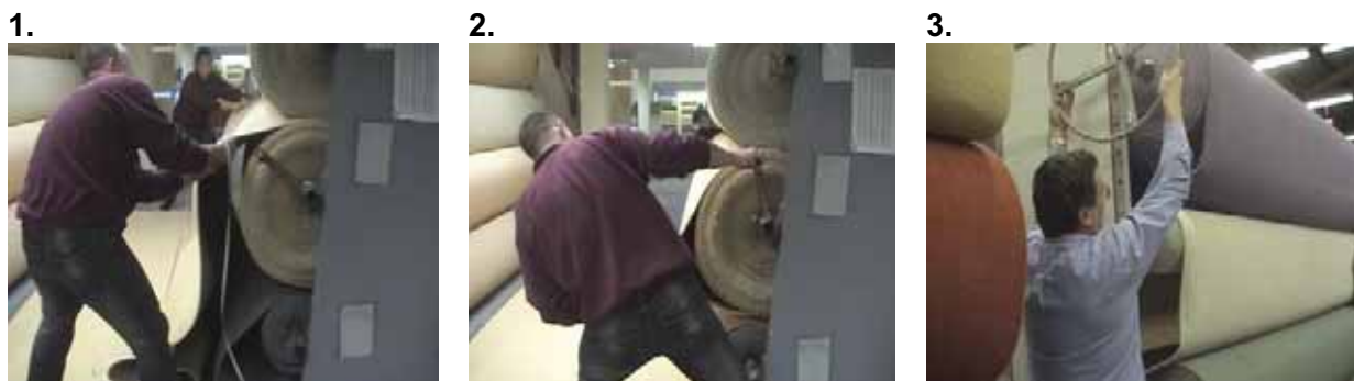
Figure 21. Different methods of unwinding / winding carpet rolls on the display rack.
