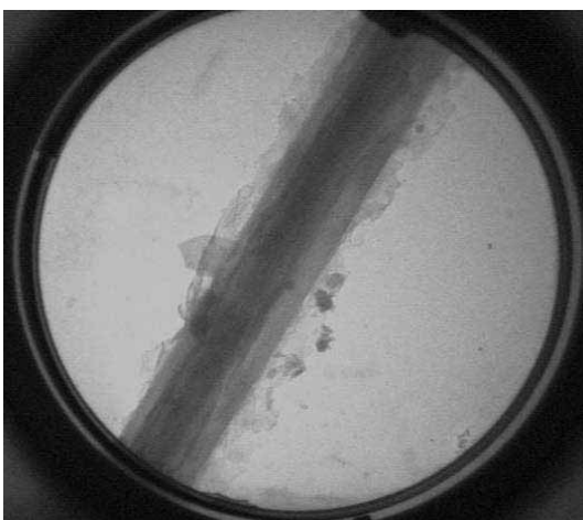
Figure 3: Example of an anthophyllite fibre from a cement matrix, which appears to be coated with a calcium and aluminium material and small particles.
