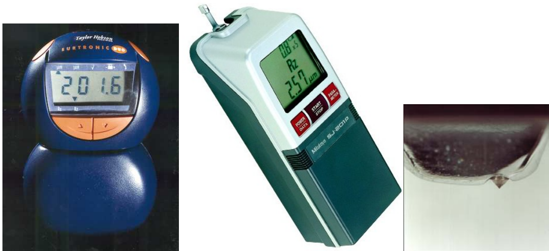
[a] Figure 2.1: [a] The Surtronic Duo Rz surface microroughness transducer, [b] The Mitutoyo Surftest SJ201P, [c] Stylus detail
