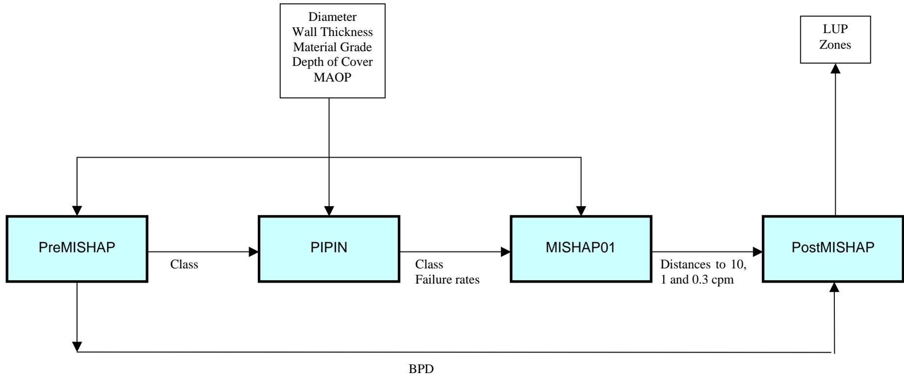
**Figure 2** Pipeline RISKAT architecture (Natural Gas exemplar)
