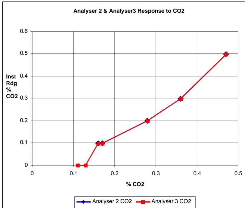
**Fig 4.3 Response of Analysers 2 and 3 to low carbon dioxide concentrations. Note: blue and red datapoints overlap at all % CO<sub>2</sub> (see Table 4.6).**
