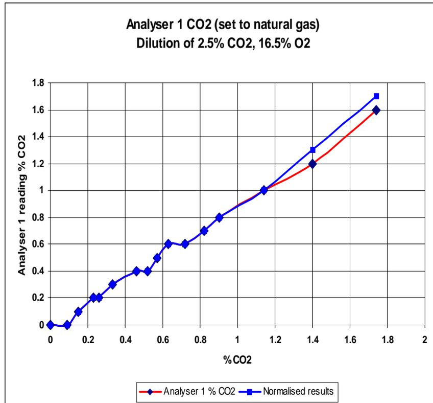
**Fig. 4.1 Response of Analyser 1 to low flue gas carbon dioxide concentrations. Note: blue and red datapoints overlap between 0 and 1.14% CO<sub>2</sub> (see Table 4.2).**
