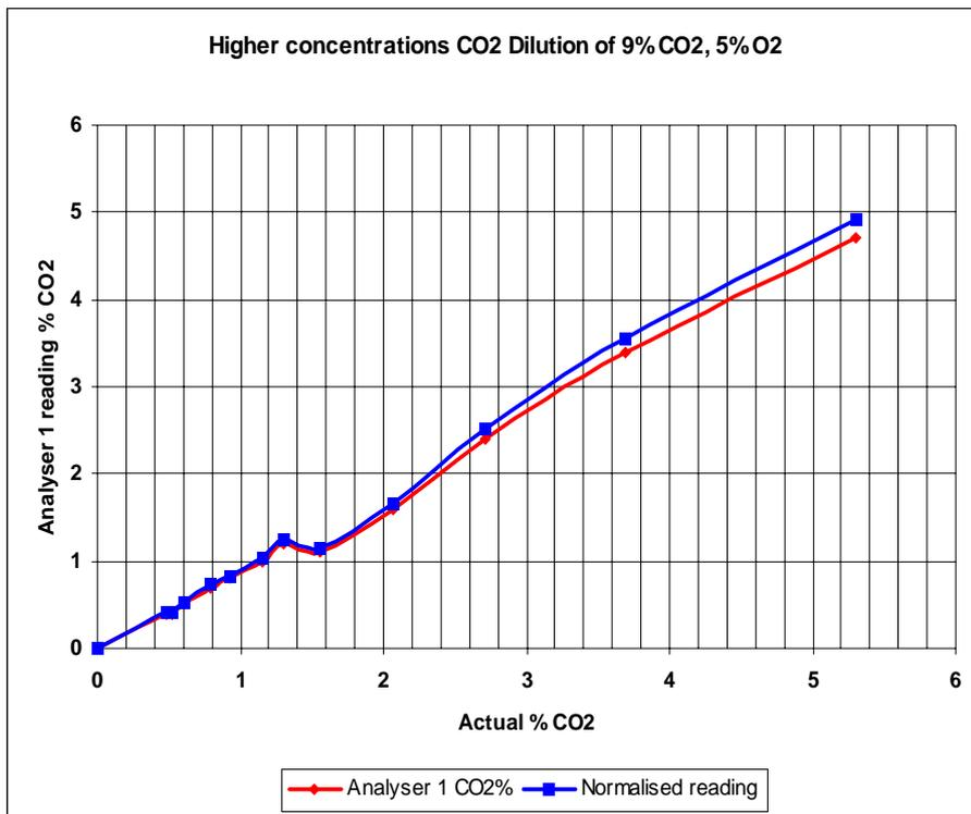
**Fig 4.2 Response of Analyser 1 to high flue gas carbon dioxide concentrations**
