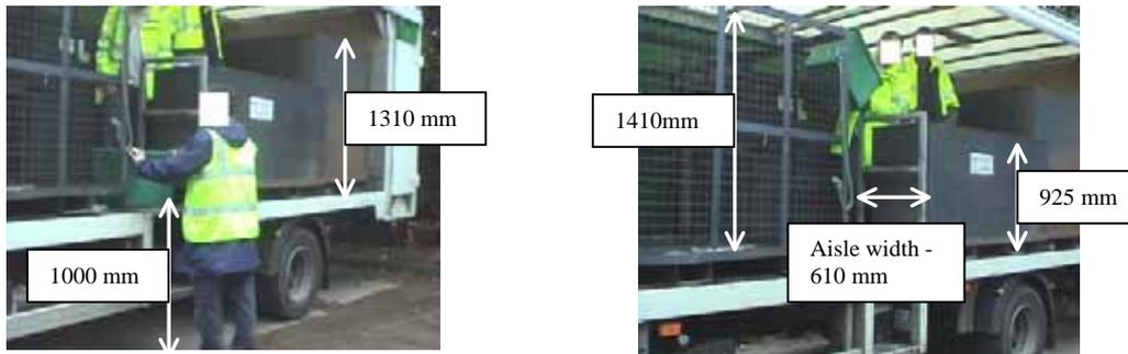
**Figure 14** Diagram to show the dimensions of vehicle 2
