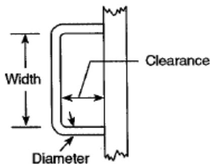
**Figure 8** Diagram of the one-handed style handhold (diagram cited in Chengalur *et al.*, 2004)
