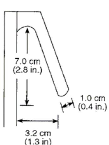
**Figure 7** Diagram of the recommended dimensions of a drawer pull handout (diagram cited in Chengalur *et al.*, 2004)
