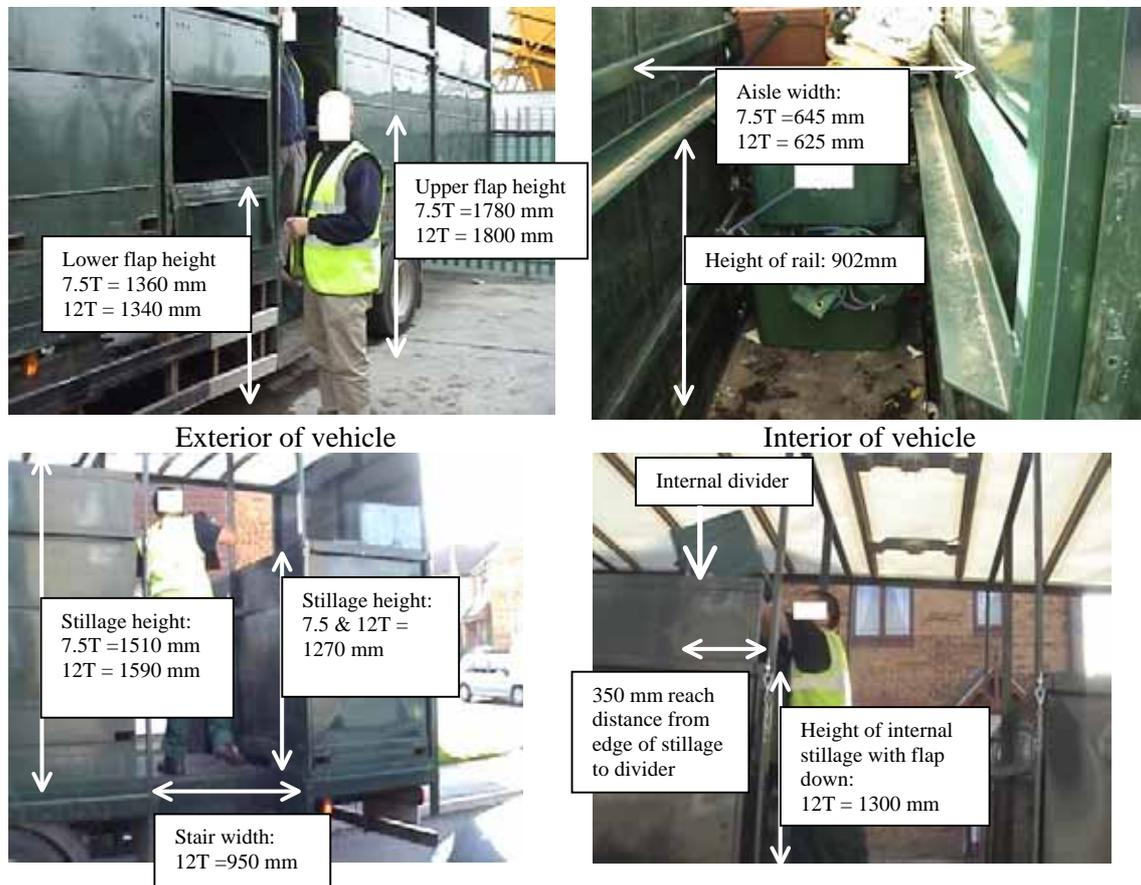
**Figure 15** Diagrams to show the dimensions of vehicle 3
