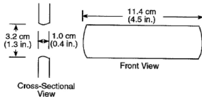
**Figure 6** Diagram of the recommended dimensions of a handhold cutout (diagram cited in Chengalur *et al.*, 2004)
