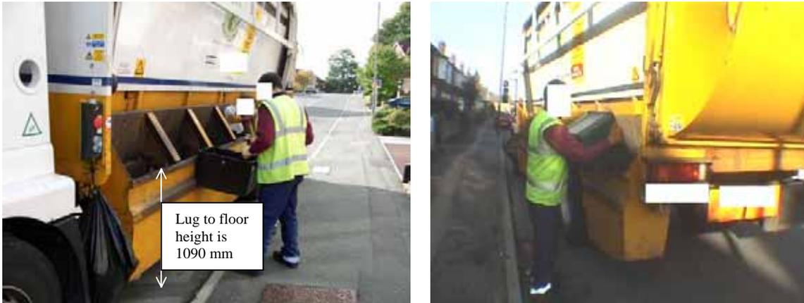
**Figure 13** A box resting on the lugs of the hopper and the contents of a box being tipped into the hopper
