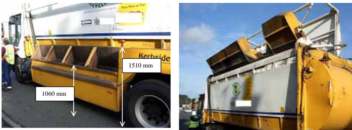
**Figure 12** The hoppers on vehicle 1 in the loading position and in a raised position, tipping the contents into the stillages within the vehicle
