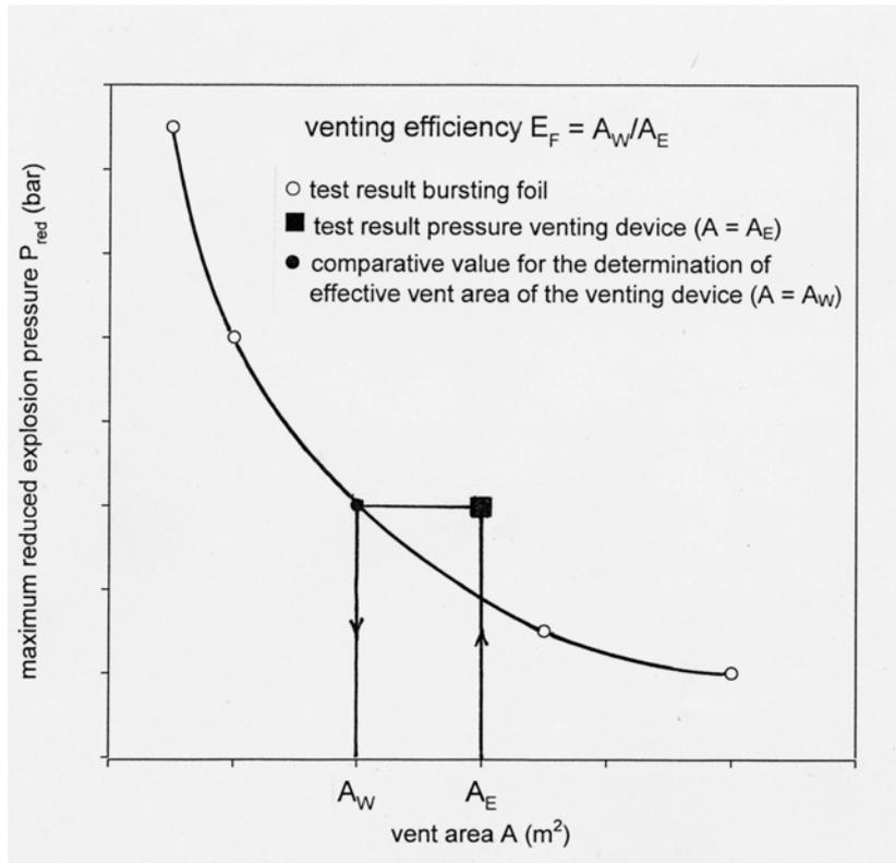
**Figure 10: Venting efficiency**
