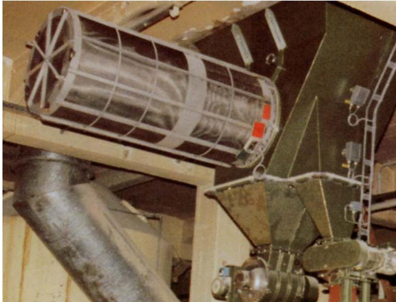
**Figure 1: Q-Rohr device installed on a vessel in a brewery**
