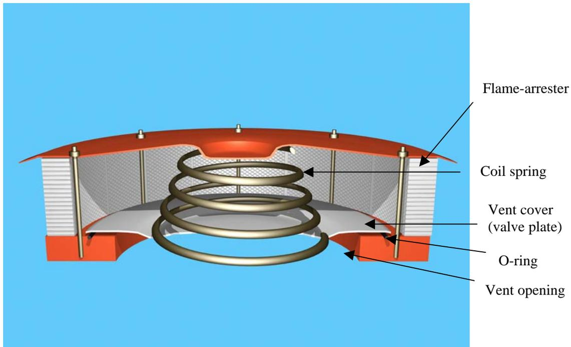
**Figure 9: Principal features of the Hoerbiger device**
