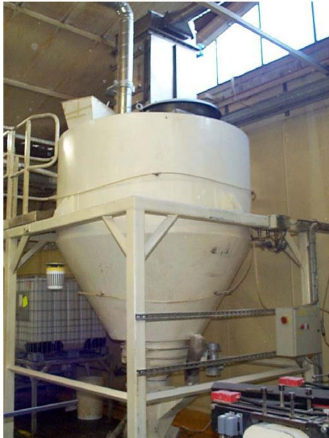
**Figure 14: Flameless venting device fitted to a batch bin**
