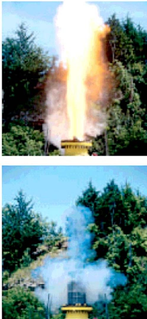
**Figure 5: Vented explosion test with and without the FlamQuench II device**
