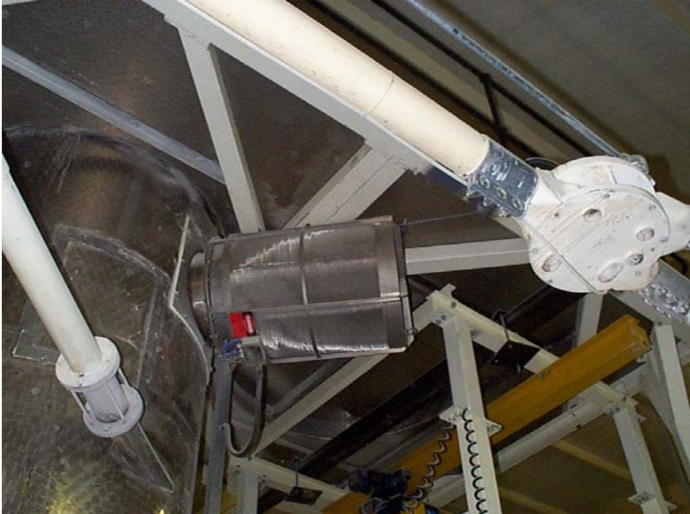
**Figure 12: Venting device in a biscuit factory**
