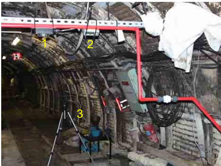
**Figure 3. Sensors used in the field tests. The Hart XL is connected to the red aspiration tube. Beneath the tube is an aviation Blue/IR sensor (1) and a MultiRae (2). In the background is the coal dust dispersion apparatus (3).**
