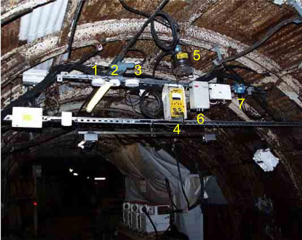
**Figure 2. Sensors used in the field tests. Ionisation smoke detector (1), domestic optical smoke sensor (2), blue/IR optical smoke detector (3), Fidesco POC: TGS 711 and CO electrochemical sensor (4), Trolex ionisation smoke detector (5), TGS 2106, 2442 and 2600 POC semiconductor sensors (6), NO<sub>2</sub> electrochemical (7).**
