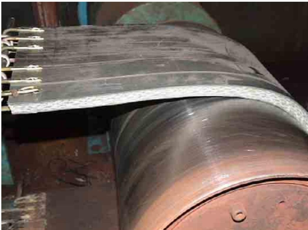
**Figure 14. Conveyor belt drum friction apparatus.**
