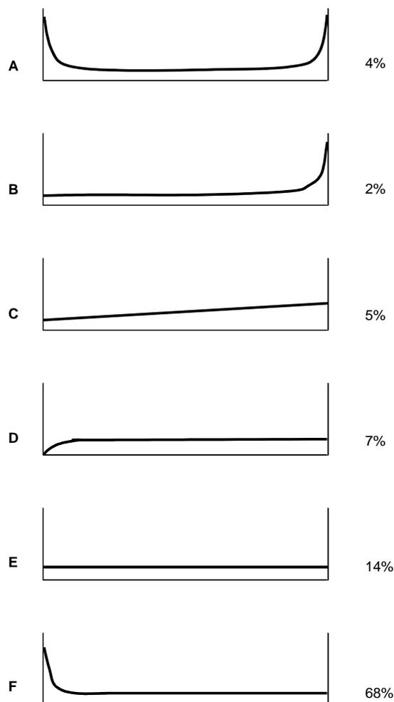
**Figure 4** Probability of failure with time (time from installation as horizontal axis, probability of failure as vertical axis). Taken from (Wilson, 1999)
