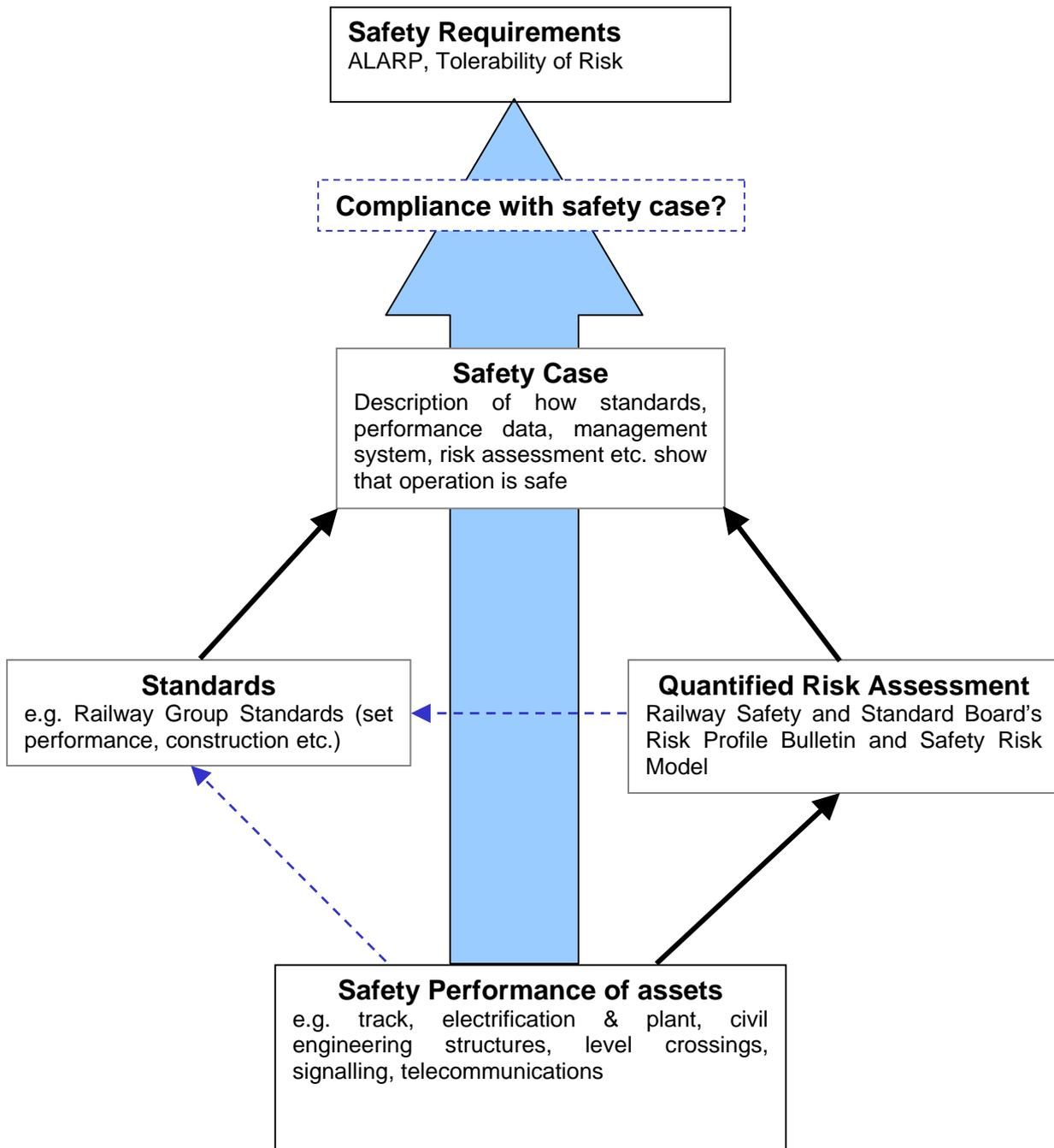
**Figure 1** Crude representation of how safety is managed on the railway network. Refer to main text for explanation
