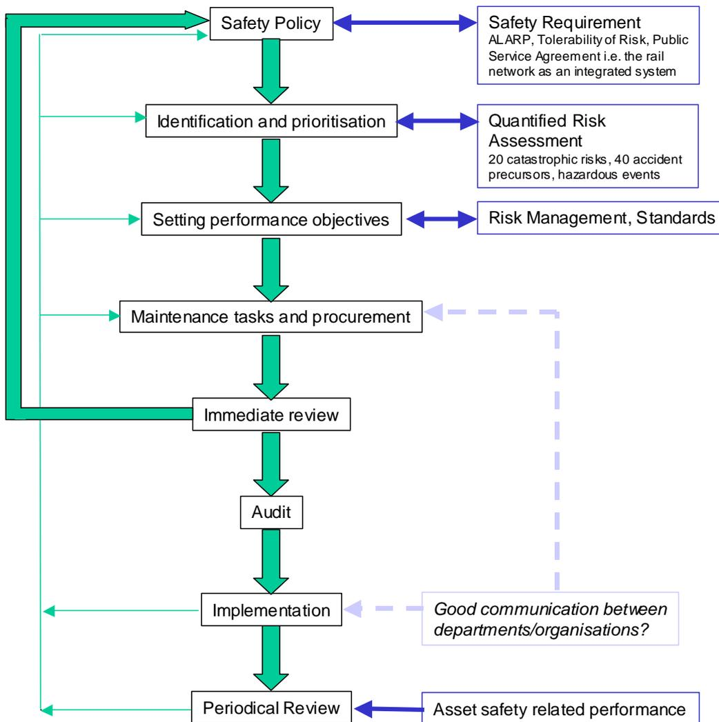
**Figure 5** Schematic of the proposed asset management approach, including linkages to items in Figure 1
