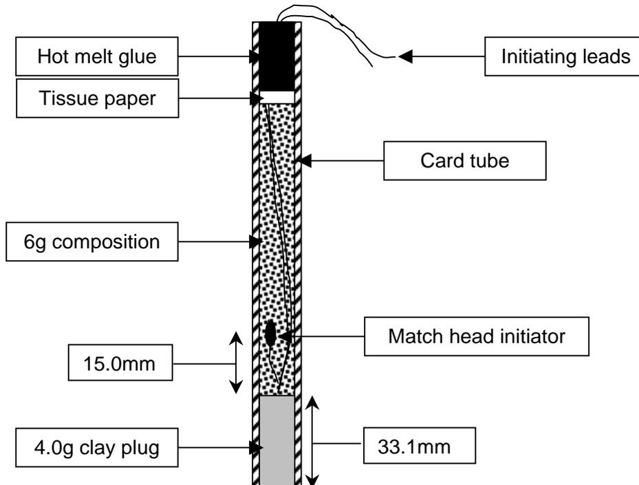
**Figure 1** Diagram showing components of prepared sample
