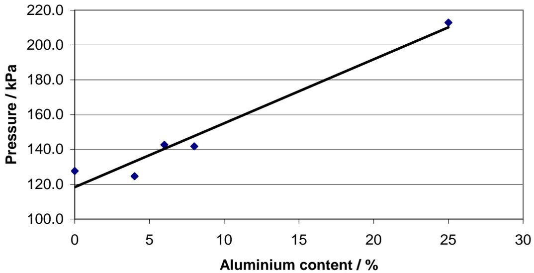
**Figure 3** Variation in peak overpressure with proportion of aluminium in the composition
