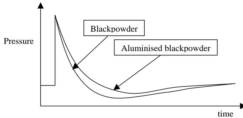
**Figure 5** Representation of the effect on the pressure time curve of energising blackpowder with aluminium
