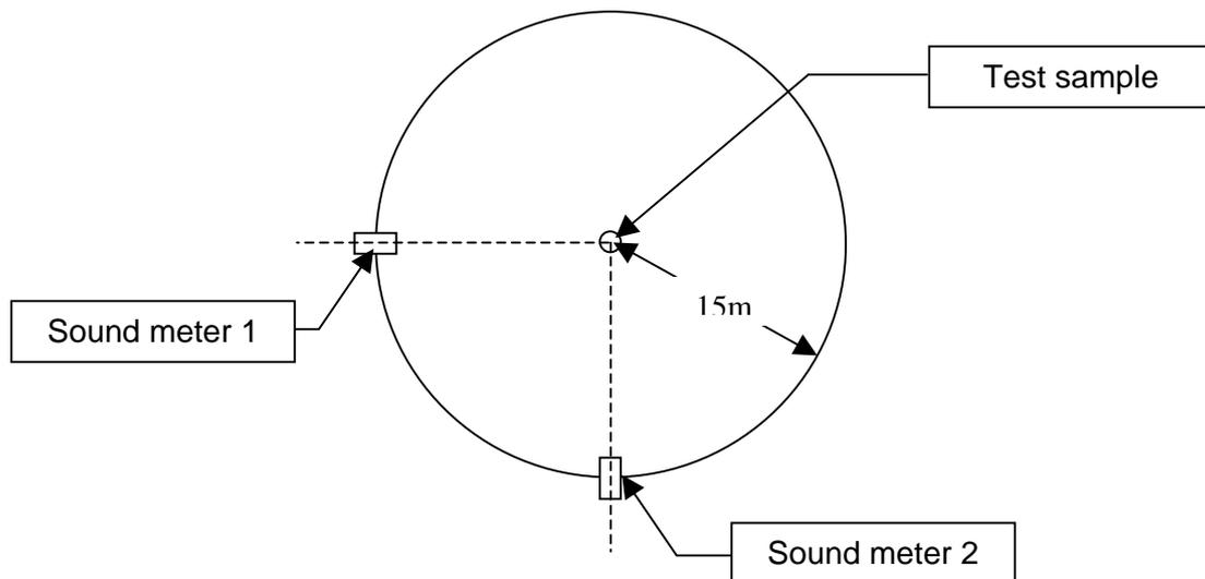
**Figure 2** Experimental set up showing relative positions of the sample and the sound meters
