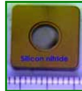
Figure 4:  $\text{Si}_3\text{N}_4$  blocks, about 5 mm thick with a 4 mm central hole. Although they were gold coloured they did not have a metallic appearance. An image of a silicon nitride tip is shown as figure 4.
