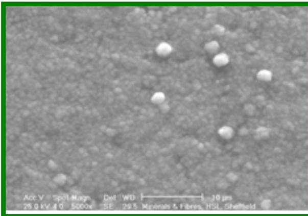
Figure 5: silicon carbide surface as received.
