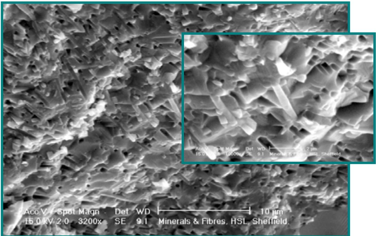
Figure 3: SiC – clean fracture surface showing SiC fibres protruding from the surface. Insert is a higher magnification image of the fibres at the centre of the main image.
