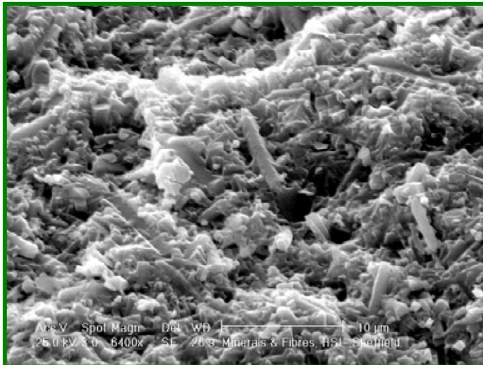
Figure 6: SEM image of silicon nitride showing fibres protruding from the fracture surface.
