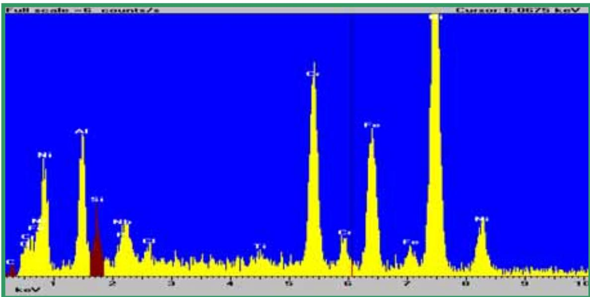
Figure 2: Typical EDX from the surface of an 'as received' silicon carbide tip.
