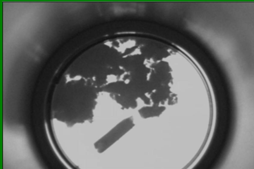
Figure 7b: TEM image of Si<sub>3</sub>N<sub>4</sub> fibres.
