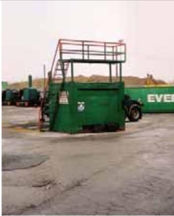
Another container modified to form a viewing platform for visual checks of the tank top at a rail freight terminal.
