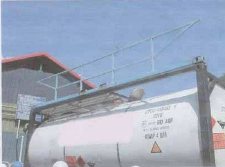
Container handrail and duckboard. Duckboard do not cover all the surface of container.
