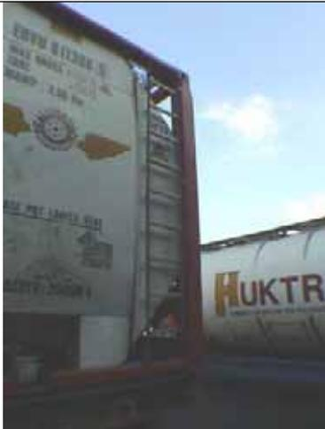
This tank has a cut away design to the end of the tank insulation to ensure reasonable toe clearance. Stiles continuous, but not enough clearance on right hand side to allow the stile to be grasped.
