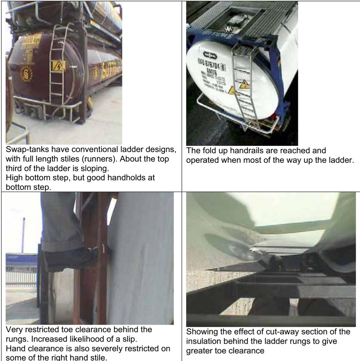
**Figure 8. The variety of tank based access features**
