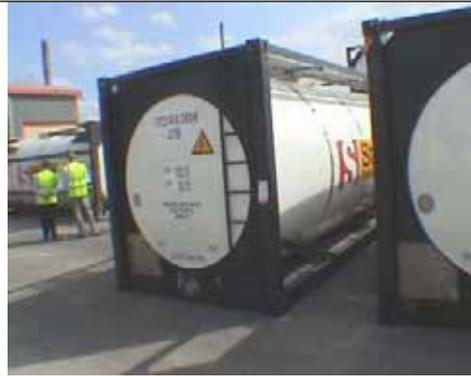
This is a frame-tank design with a full length ladder, but the toe clearance is severely restricted throughout the climb. Stiles on both sides, but the lack of clearance behind may obstruct a gloved hand. Solid design means that the position of the rungs cannot be seen through the walkway from above.
