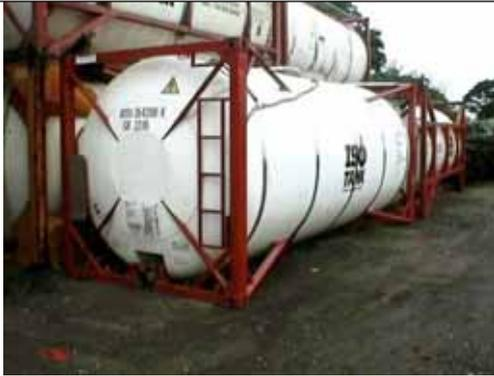
Another beam tank design. Here the ladder is partial. There appears to be a small additional step provided close to the top. Toe clearance appears to be reduced for the central portion of the climb. Stile on both sides, at least partially. High first rung. Offset top step.
