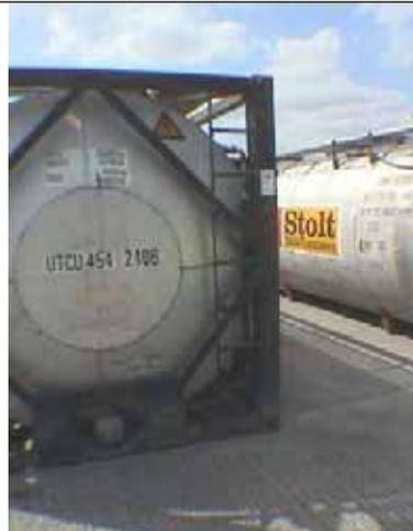
Good toe clearance but obstructed/altered rungs at the middle of the ladder. Rungs obstructed near the mid point of the ladder. Right hand stile is the tank frame. Too large to grasp.
