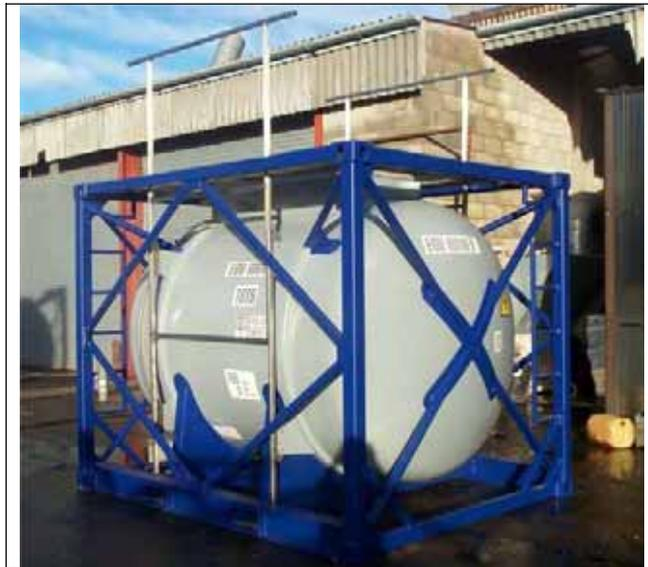
**Figure 3. 10 foot tank container unit with slide-up handrails**
