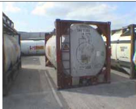
A beam tank with a conventional ladder. However the structure of the end frame obstructs the ladder rungs at the top and bottom. There also appears to be restricted toe clearance. While there are stiles on both sides, the clearance around the left hand stile appears to be restricted, especially for a gloved hand.
