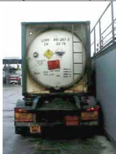
This design appears to enable a complete conventional ladder to be provided, with good toe and hand clearance throughout (6 rungs). Only criticism is that the position of rungs cannot be seen from above.
