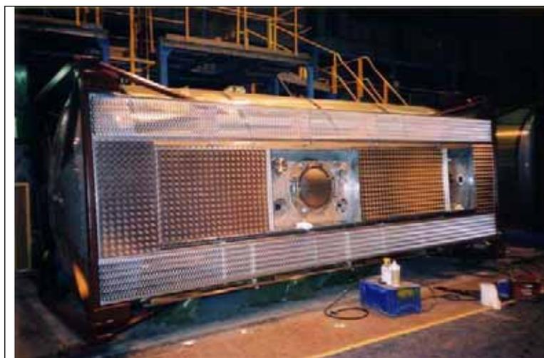
**Figure 6. Tank rotated to give access to the top surface during manufacture.**
