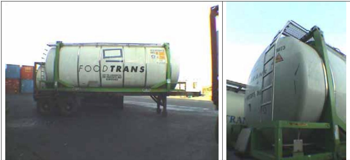
**Figure 4. A swap-body or swap tank on a trailer ready for transport by road. Note the extension beyond the corner castings, and the design of the ladder. This one has a fold up handrail, which can be raised once at the top of the ladder.**
