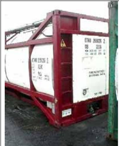
A further design variation. The frame structure forms the top and bottom rung, but the toe clearance is very restricted. Hand holds are on the rungs only.
