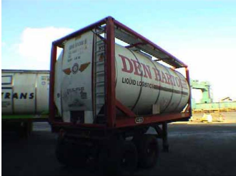
**Figure 1. A typical tank container of the original, or 'frame-tank' design on a trailer chassis.**
