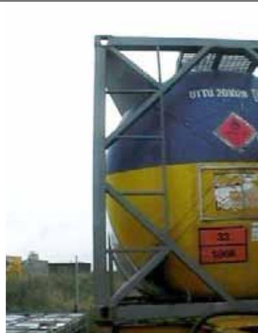
This illustrates the difference in the vertical spacing between the rungs provided, as there are 4 rungs. Rung spacing is consistent though. Angled structure is not in the place of a rung, and so less likely to present a hazard.
