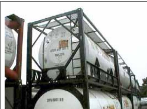
Frame tank with a largely uninterrupted ladder. The structure of the end frame interferes with the ladder towards its centre rather than at the top or bottom. Toe clearance looks to be good throughout the length of the ladder. However the ladder has a stile on one side only. The right side is too large to be grasped
