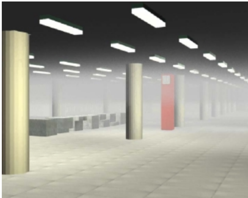
Figure 6 - Illustration of smoke visibility obtained from CFD predictions on an underground station concourse - top: no smoke; bottom: visibility through smoke (courtesy of Mott MacDonald Limited)
