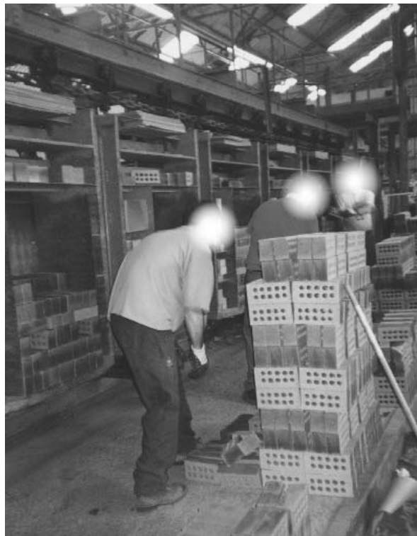
Figure 10: Packing using a monorail. The fronts of the kiln packs have been stripped down before removing bricks from the rear. Seconds are put in jig pockets and above the jig
