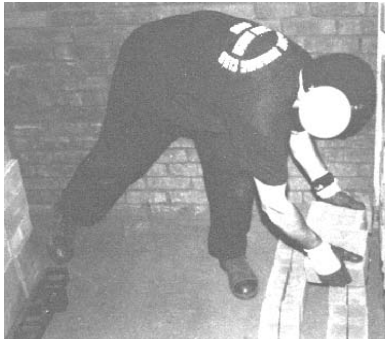
Figure 13: Hand packing from kiln packs on the floor to despatch packs on trays with a bent and twisted posture
