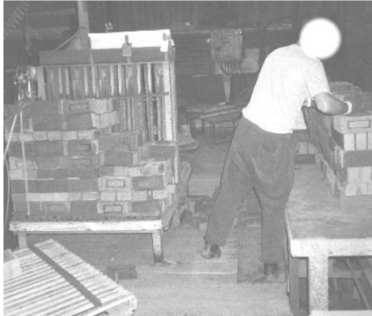
Figure 14: Hand packing from kiln packs two blades deep to jigs five blades deep. The kiln pack is on a platform to bring its base to about knee height
