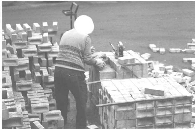
Figure 18: Hand packing in the open from kiln packs on the ground to despatch packs on the ground.
