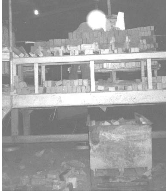
Figure 16: Hand packing of bricks on a high level platform. Waste bricks go into the skip beneath the platform. The end on orientation of the bricks permits handling of large numbers at once
