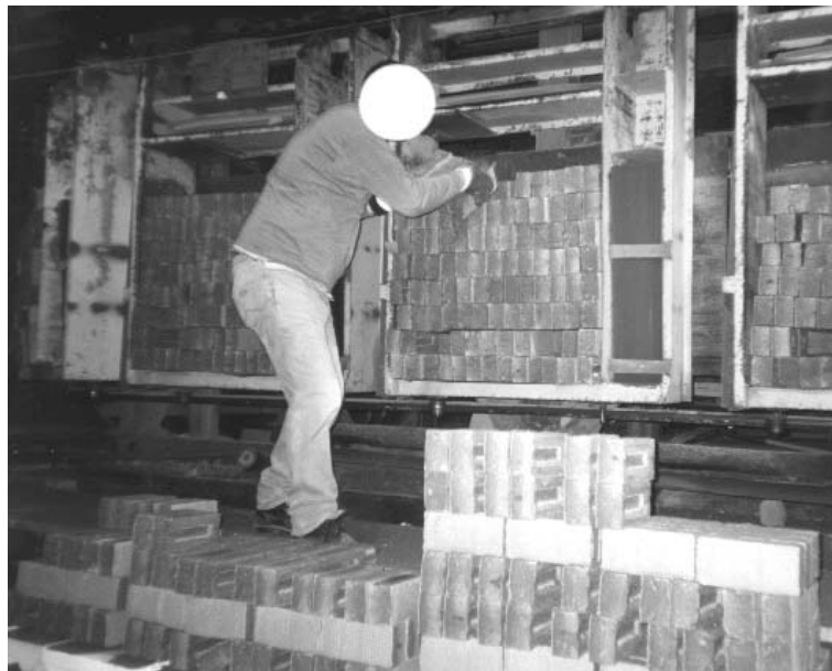
Figure 17: Packing from kiln cars using a high level monorail. At this point there is a large vertical distance between the start and the finish of the lift
