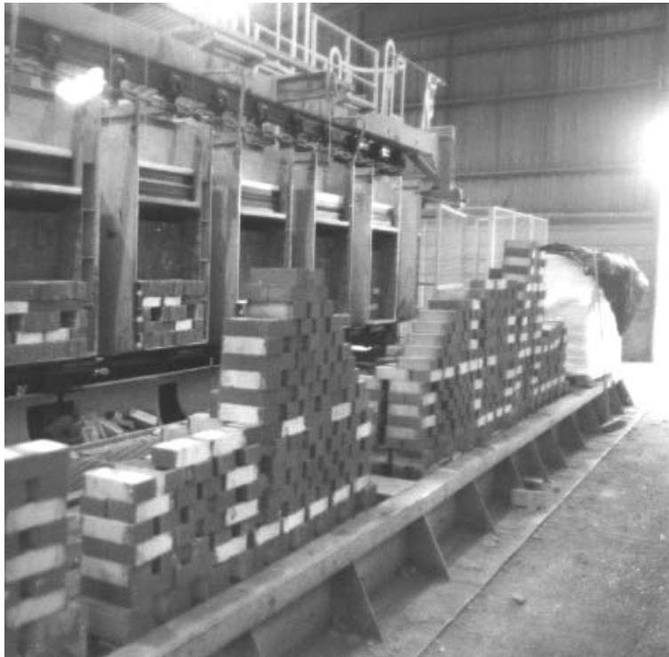
Figure 11: A monorail with the bottom half of the kiln packs lowered into recesses. The fronts of the kiln packs have been stripped down before removing bricks from the rear.
